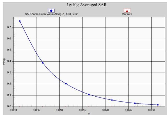
**Fig. 1-42 Z-Scan at power reference point (LTE Band 7)**
