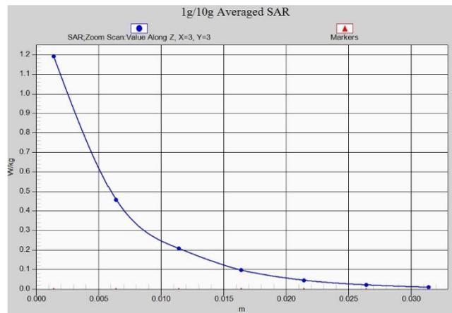
Fig. 1-46 Z-Scan at power reference point (2450 MHz)
