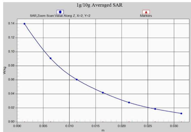
**Fig. 1-43 Z-Scan at power reference point (LTE Band38)**
