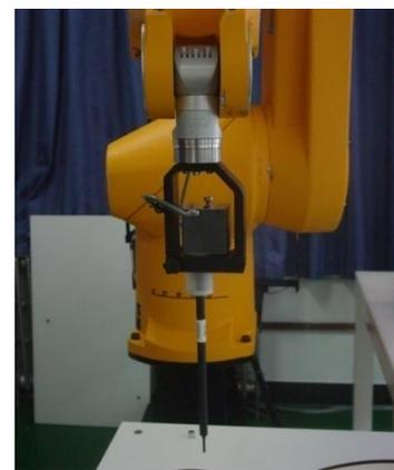
Picture C.3 E-field Probe
