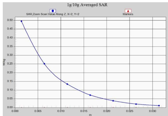
**Fig. 1-51 Z-Scan at power reference point (BT)**
