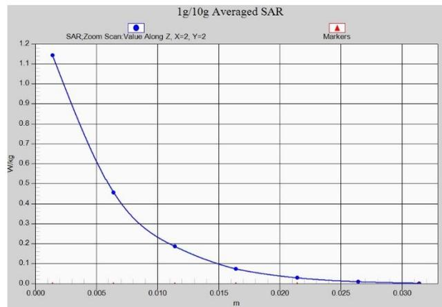
**Fig. 1-19 Z-Scan at power reference point (LTE Band38)**
