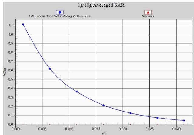
**Fig. 1-22 Z-Scan at power reference point (PCS1900)**
