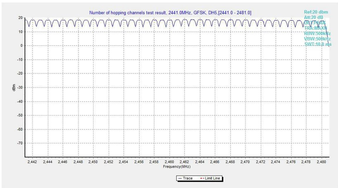
Fig.110. Number of hopping frequencies: GFSK, Channel 40 - 78
