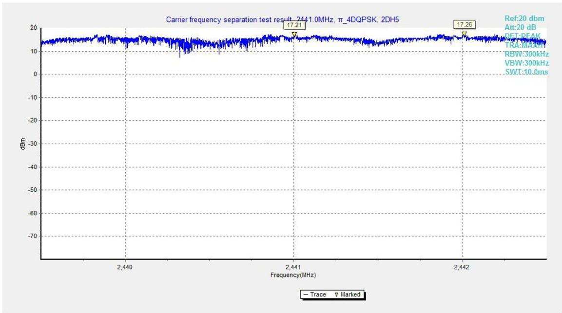
Fig.107. Carrier frequency separation measurement:  $\pi/4$  DQPSK, Channel 39
