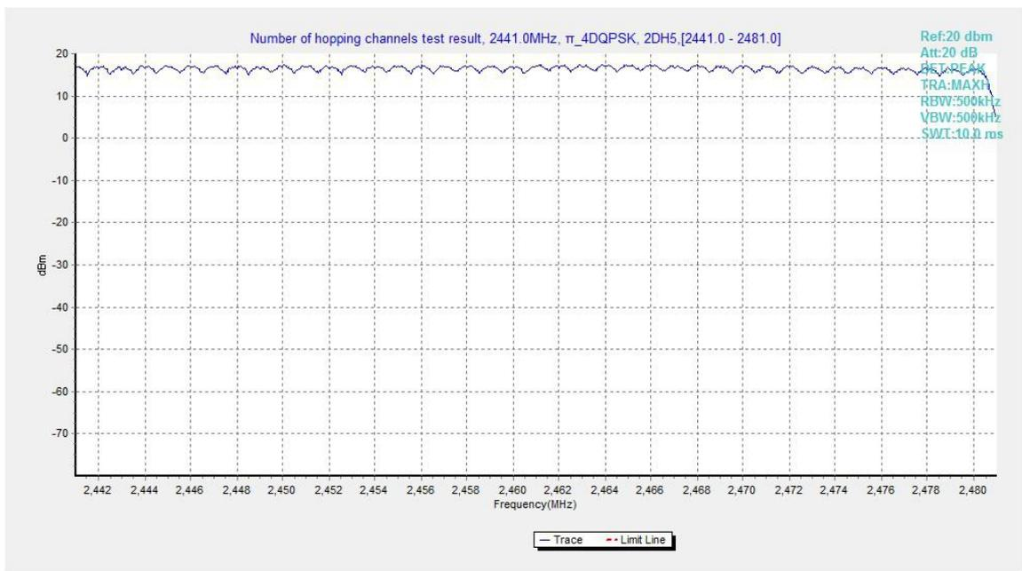
Fig.112. Number of hopping frequencies:  $\pi/4$  DQPSK, Channel 40 - 78
