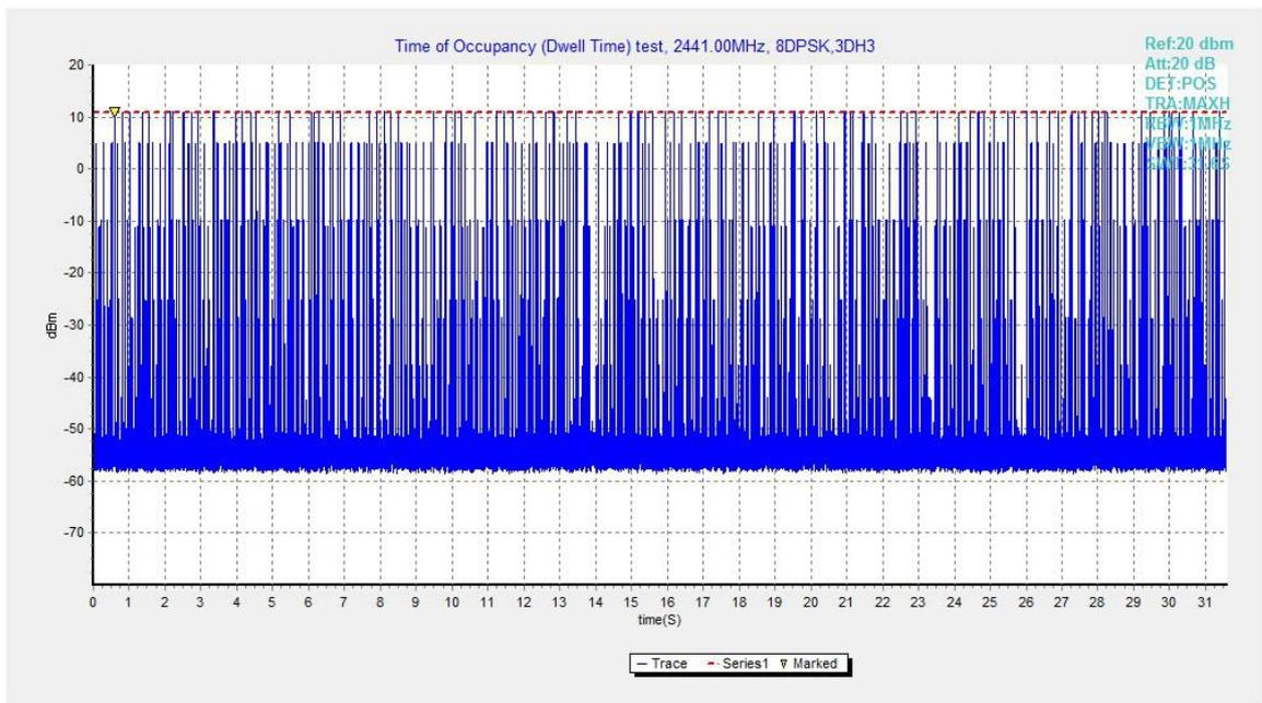
Fig.94. Number of Transmissions Measurement: Channel 39,Packet 3-DH3
