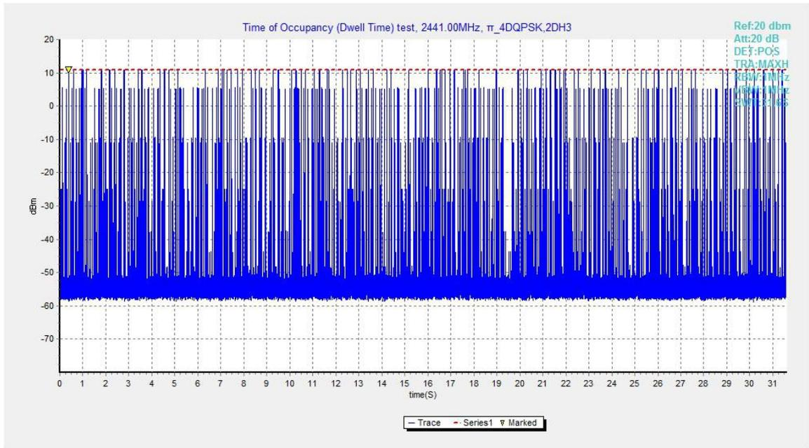
Fig.88. Number of Transmissions Measurement: Channel 39,Packet 2-DH3
