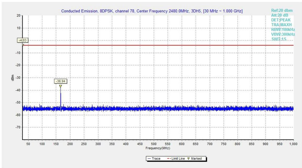
Fig.75. Conducted spurious emission: 8DPSK, Channel 78, 30MHz - 1GHz
