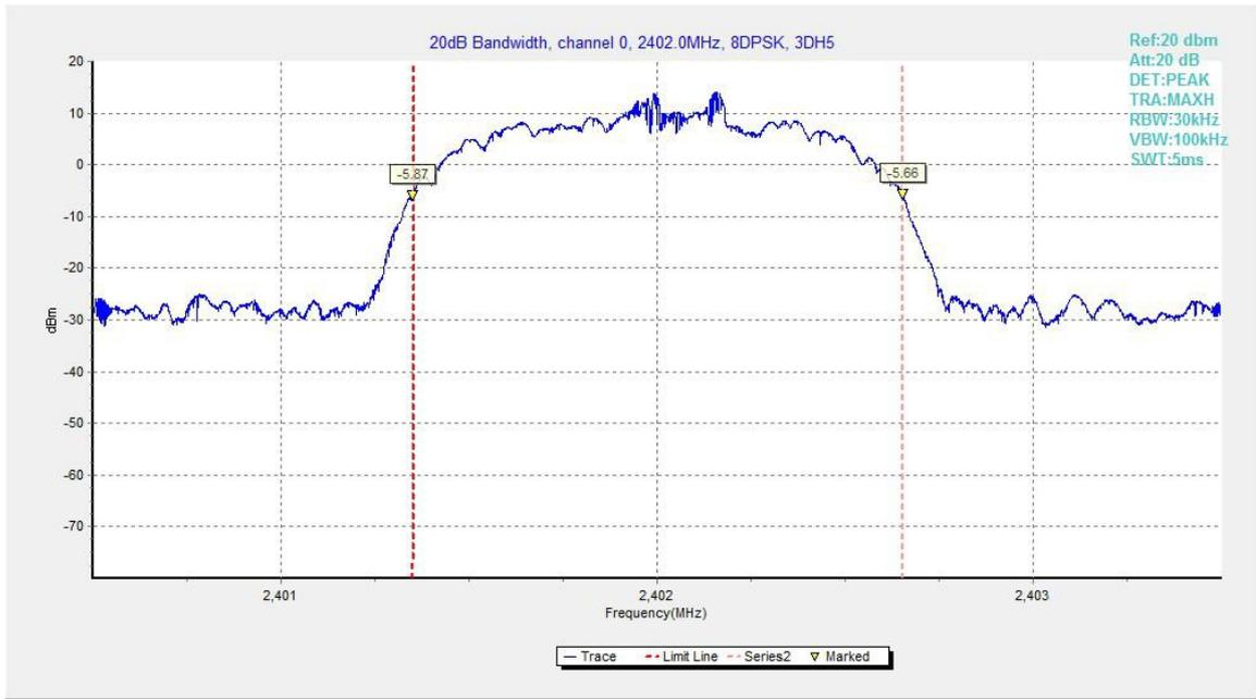
Fig.103. 20dB Bandwidth: 8DPSK, Channel 0
