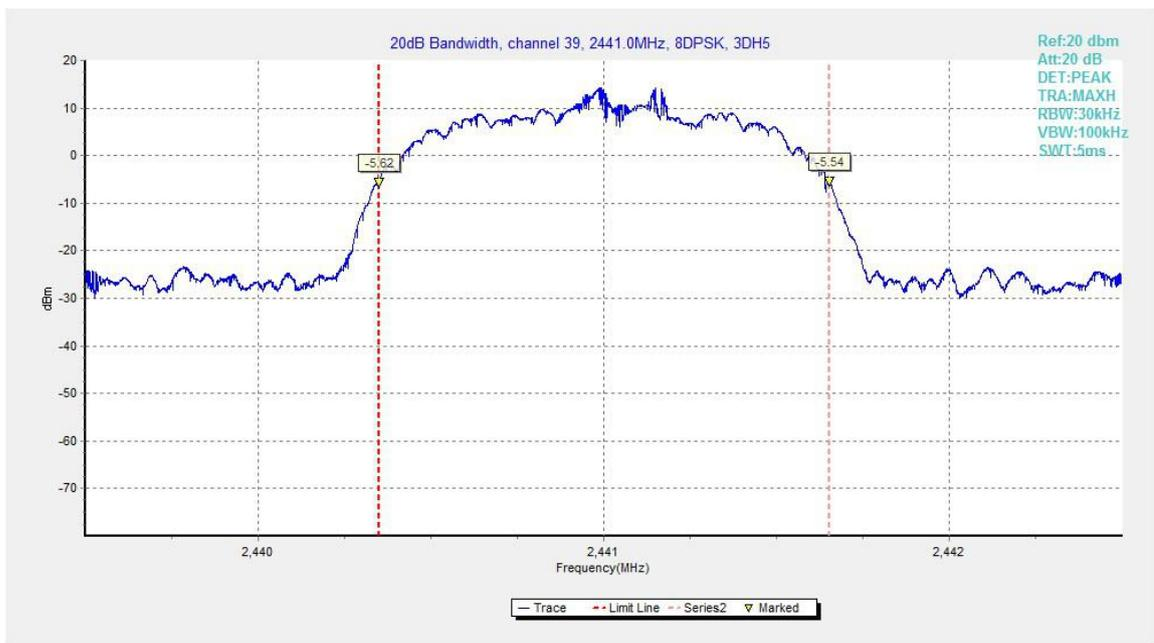
Fig.104. 20dB Bandwidth: 8DPSK, Channel 39
