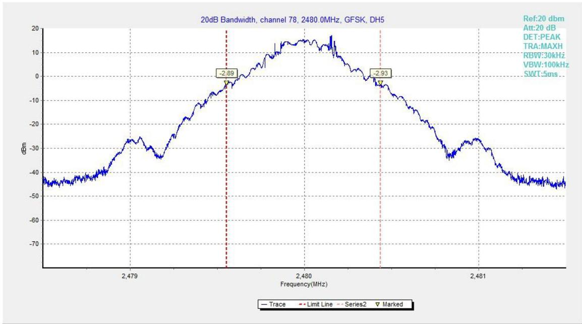
Fig.99. 20dB Bandwidth: GFSK, Channel 78
