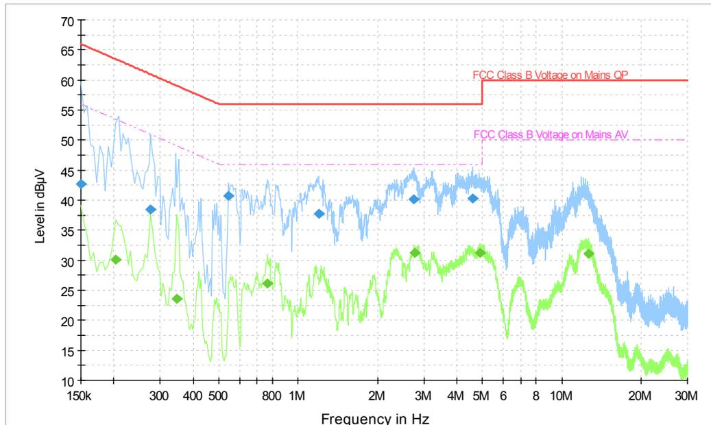
**Fig.A.11.3 AC Powerline Conducted Emission- Bluetooth
