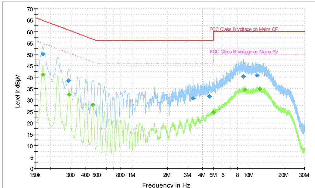
**Fig.A.11.2 AC Powerline Conducted Emission-Idle EUT3(M2001J2G)+AE1+AE3+AE6**
