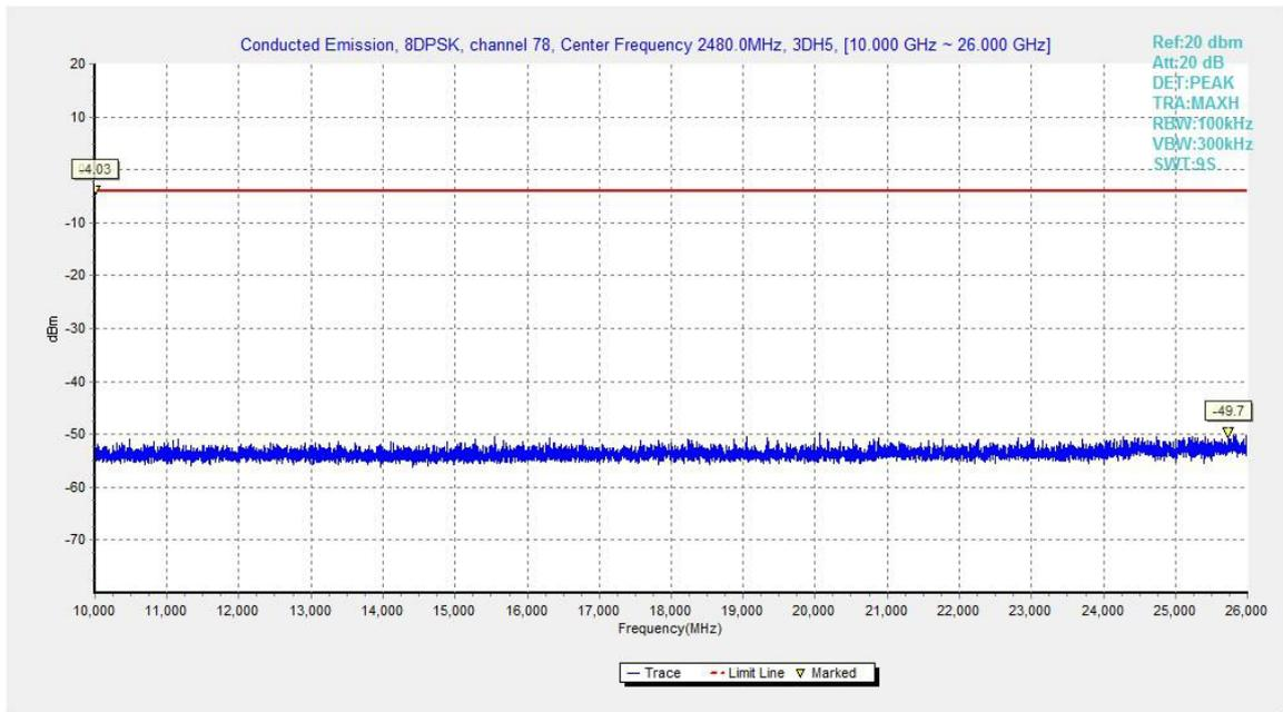
Fig.78. Conducted spurious emission: 8DPSK, Channel 78, 10GHz - 26GHz
