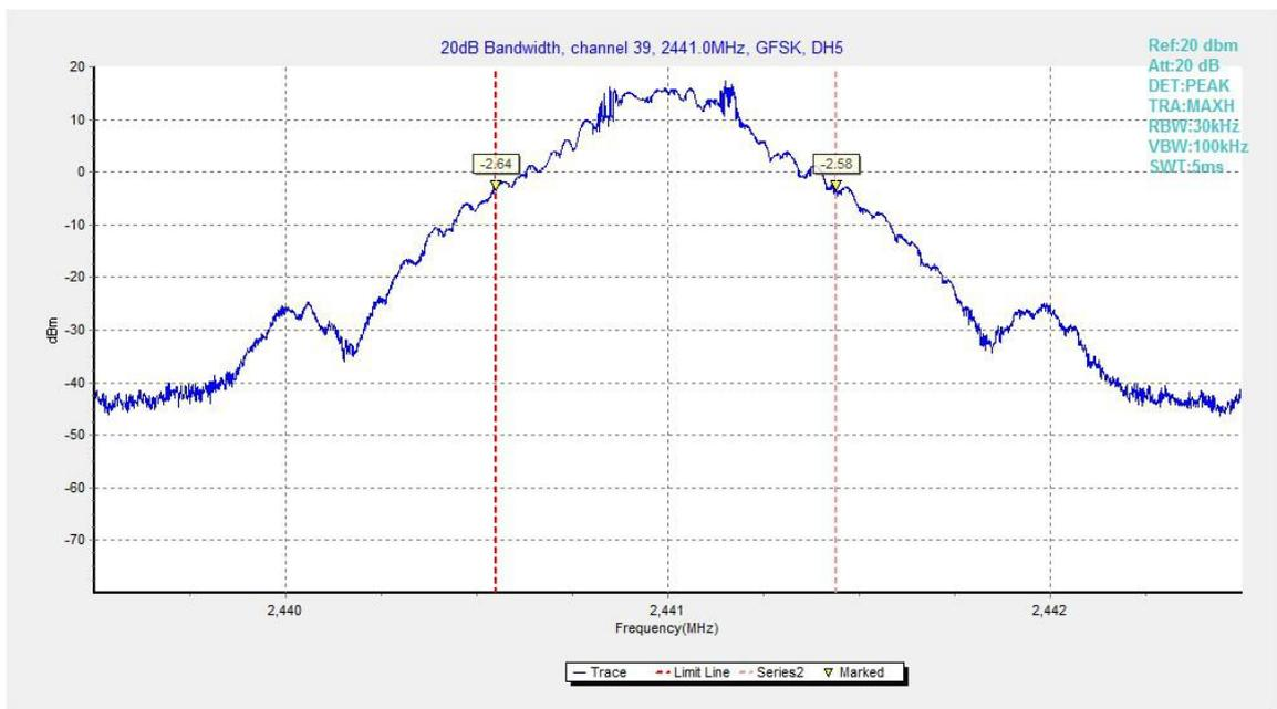
Fig.98. 20dB Bandwidth: GFSK, Channel 39
