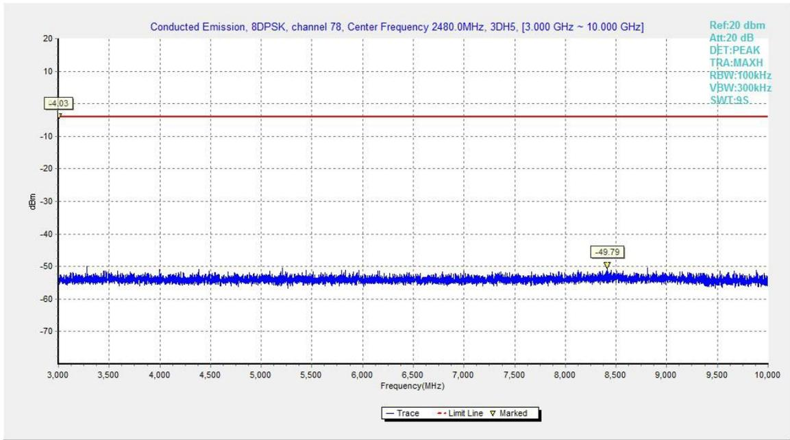
Fig.77. Conducted spurious emission: 8DPSK, Channel 78, 3GHz - 10GHz
