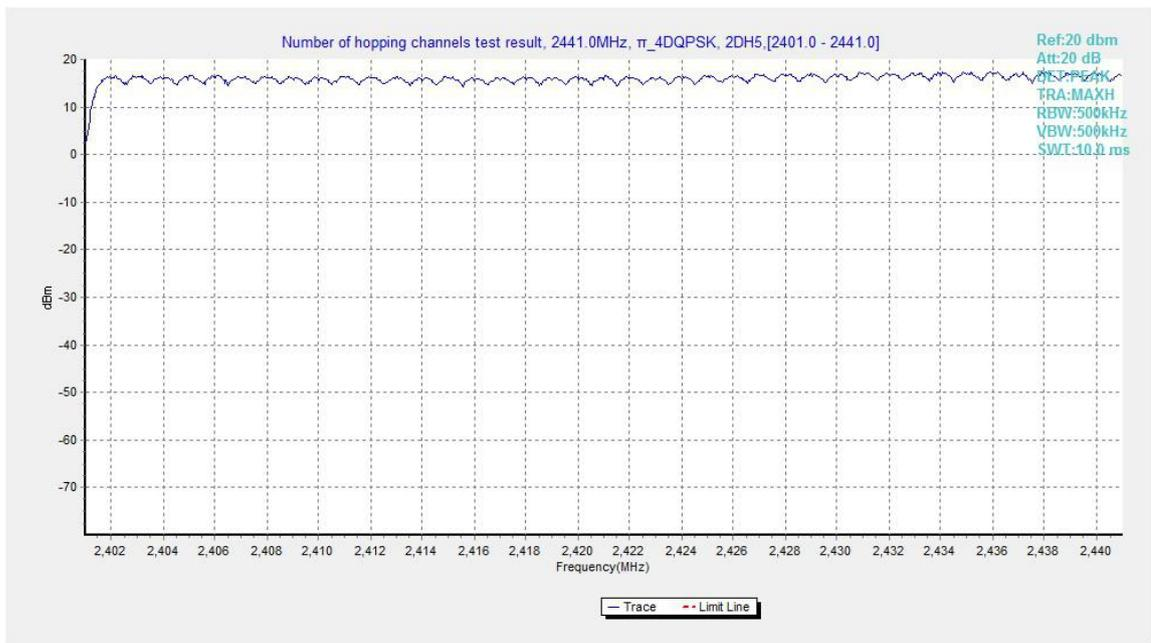
Fig.111. Number of hopping frequencies:  $\pi/4$  DQPSK, Channel 0 - 39
