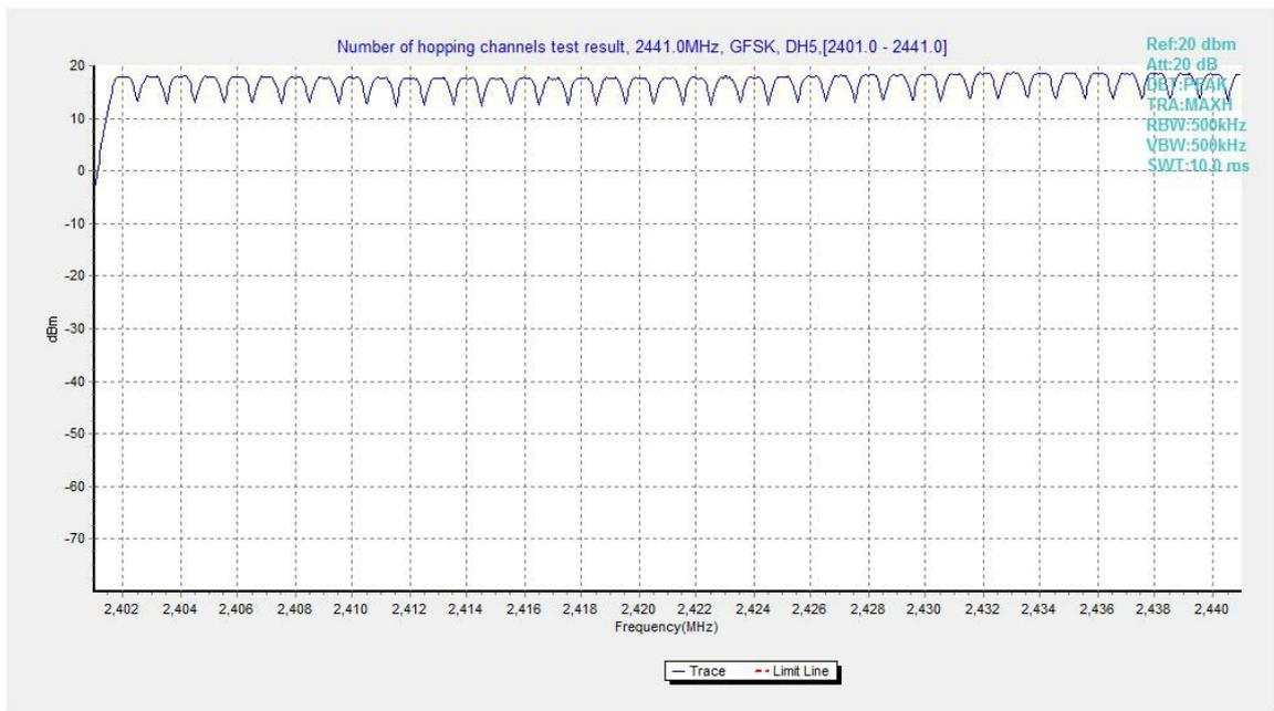
Fig.109. Number of hopping frequencies: GFSK, Channel 0 - 39
