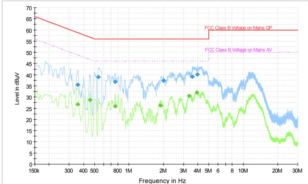
**Fig.A.11.4 AC Powerline Conducted Emission-Idle
