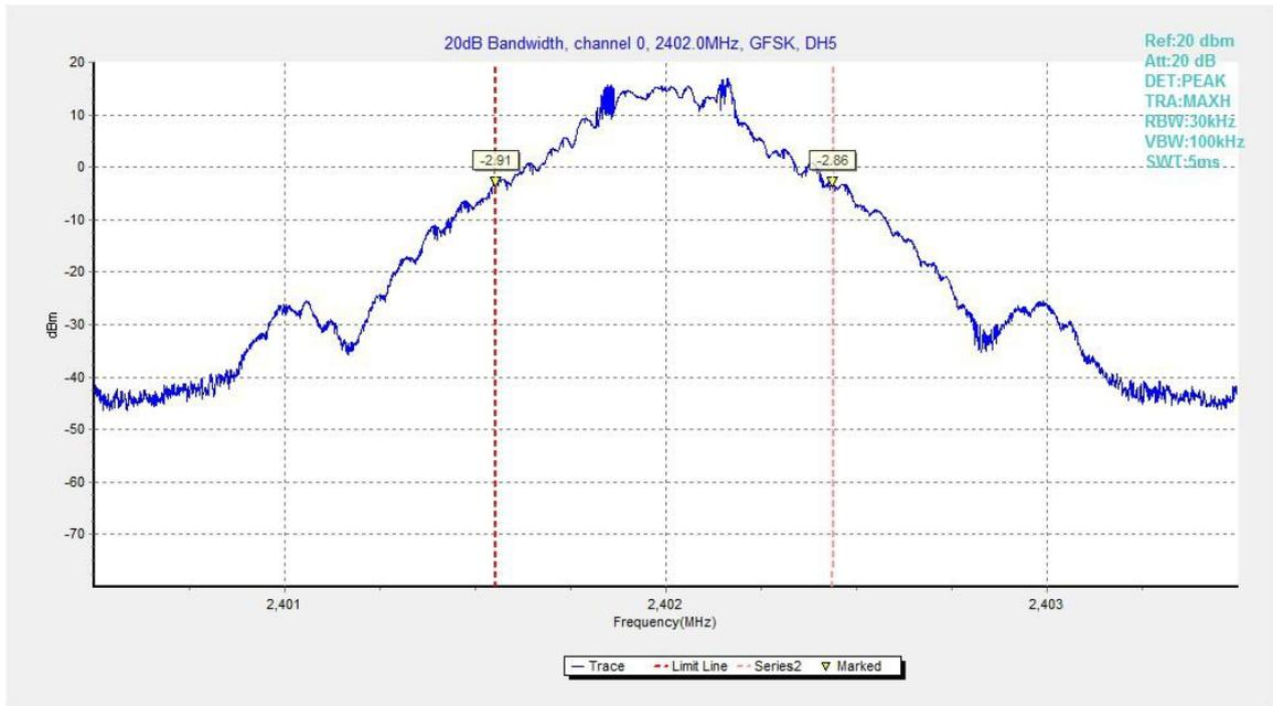
Fig.97. 20dB Bandwidth: GFSK, Channel 0
