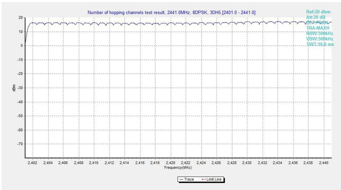
Fig.113. Number of hopping frequencies: 8DPSK, Channel 0 - 39
