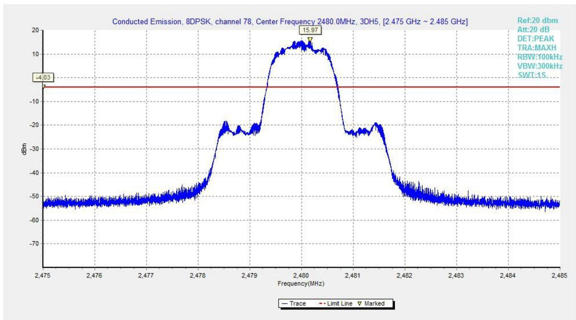
Fig.74. Conducted spurious emission: 8DPSK, Channel 78, 2480MHz
