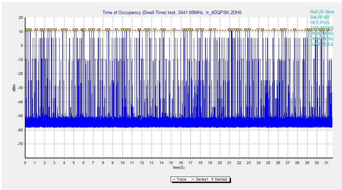
Fig.90. Number of Transmissions Measurement: Channel 39,Packet 2-DH5
