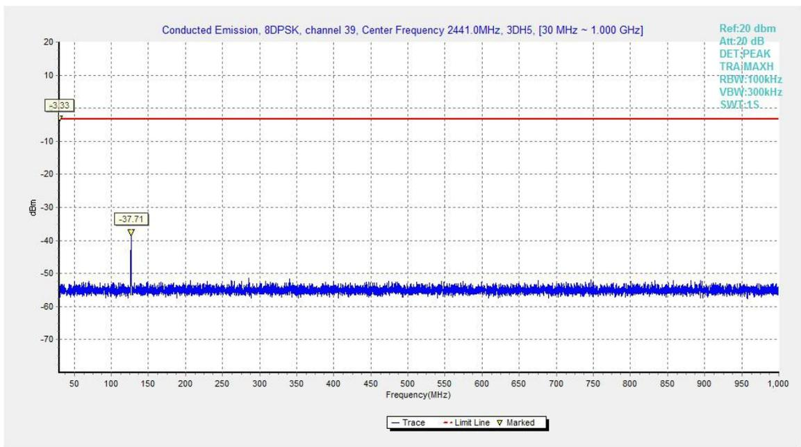
Fig.70. Conducted spurious emission: 8DPSK, Channel 39, 30MHz - 1GHz
