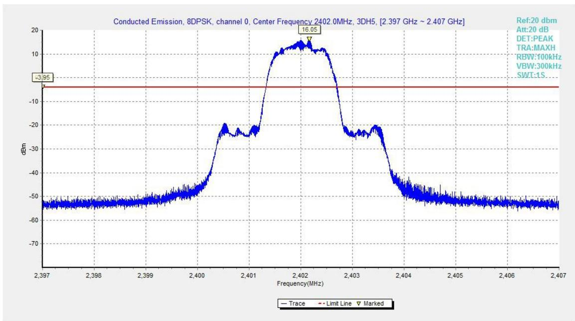
Fig.64. Conducted spurious emission: 8DPSK, Channel 0, 2402MHz
