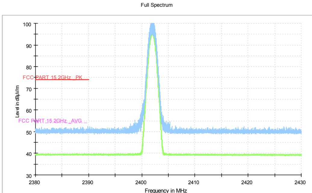
**Fig.22. Frequency Band Edges: EUT3 ANT3 GFSK, Channel 0, Hopping Off, 2.38 GHz – 2.45GHz**
