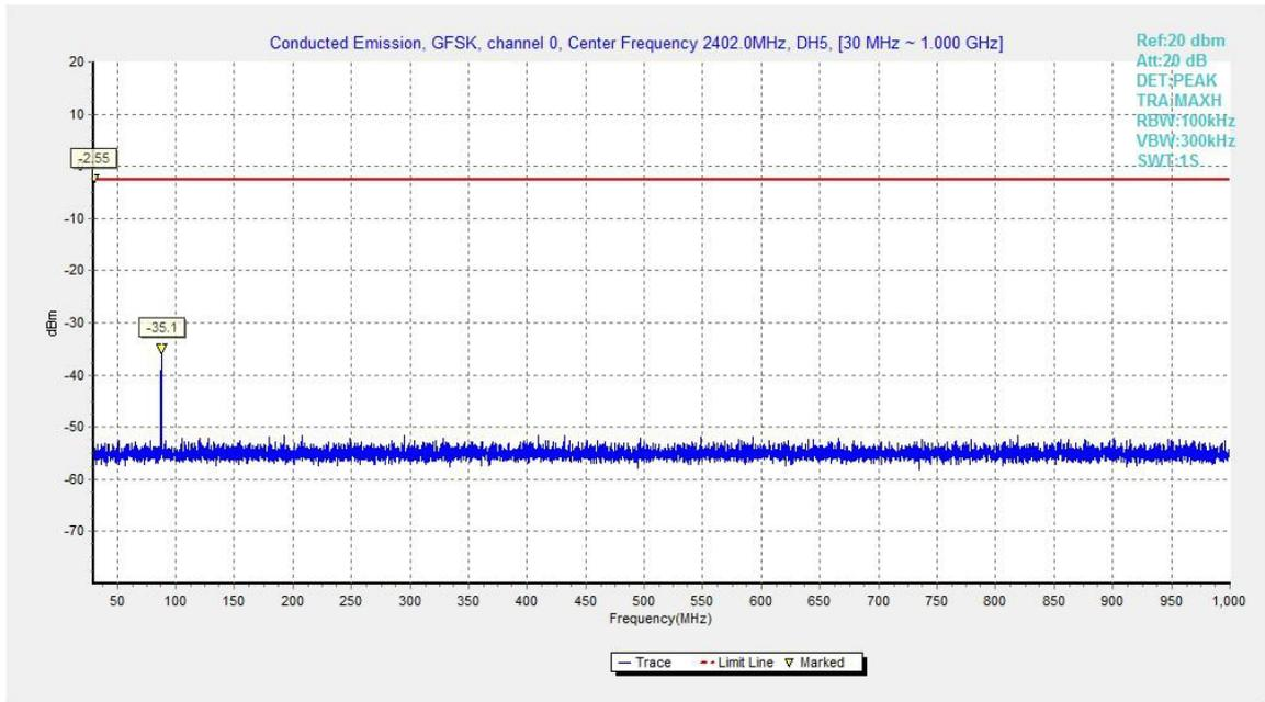
Fig.35. Conducted spurious emission: GFSK, Channel 0, 30MHz - 1GHz
