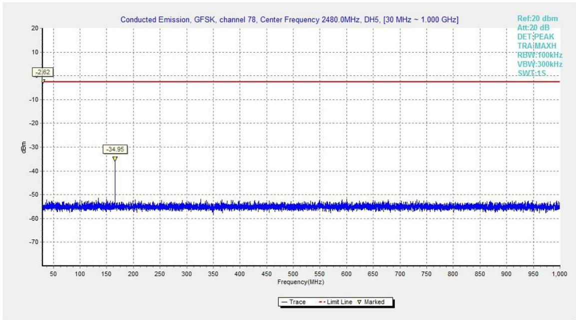
Fig.45. Conducted spurious emission: GFSK, Channel 78, 30MHz - 1GHz
