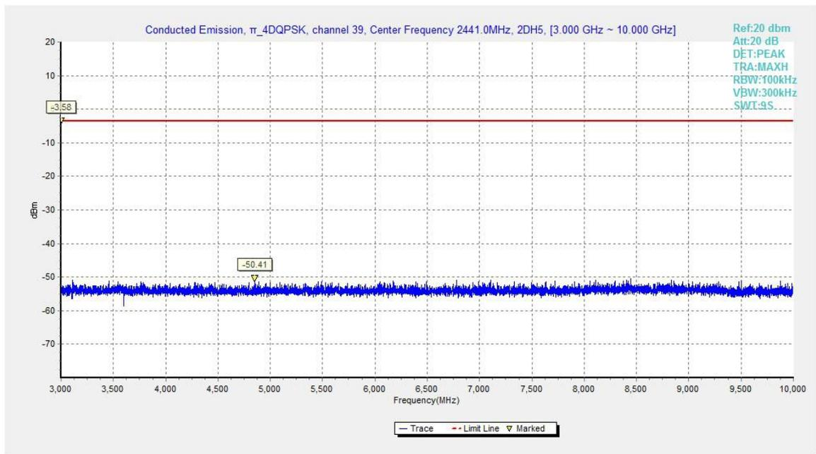
Fig.57. Conducted spurious emission:  $\pi/4$  DQPSK, Channel 39, 3GHz - 10GHz
