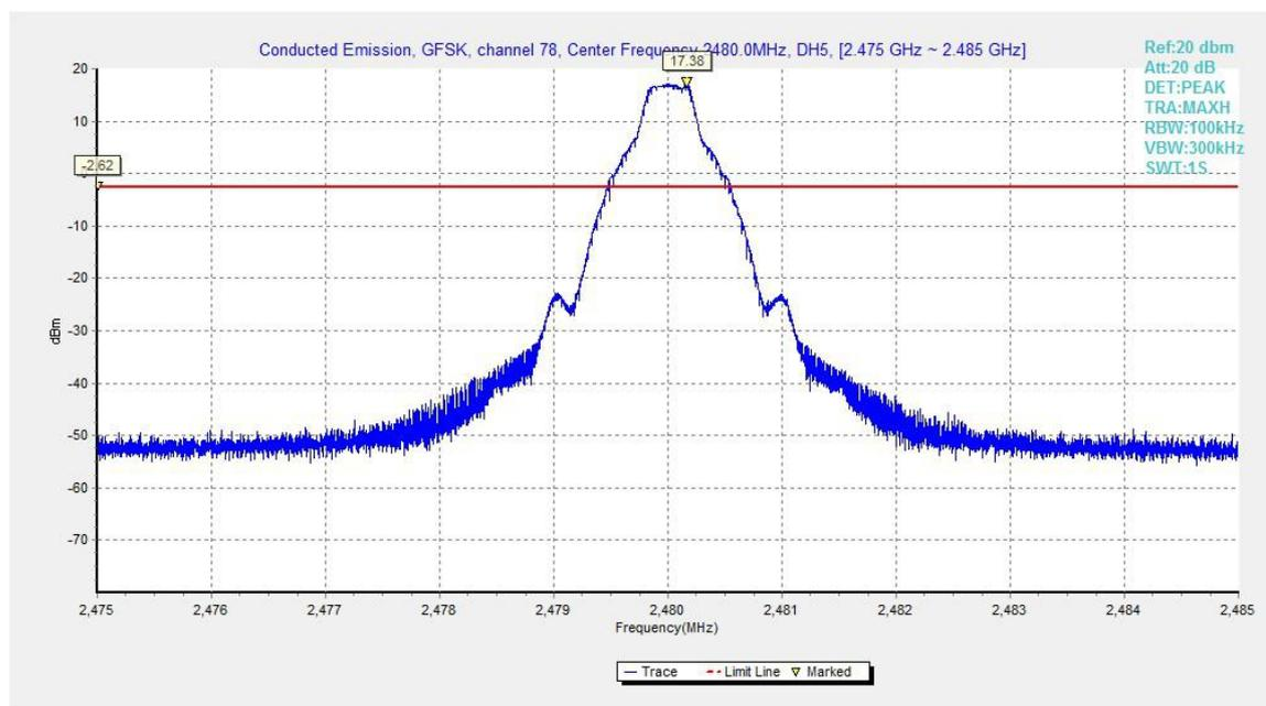
Fig.44. Conducted spurious emission: GFSK, Channel 78, 2480MHz
