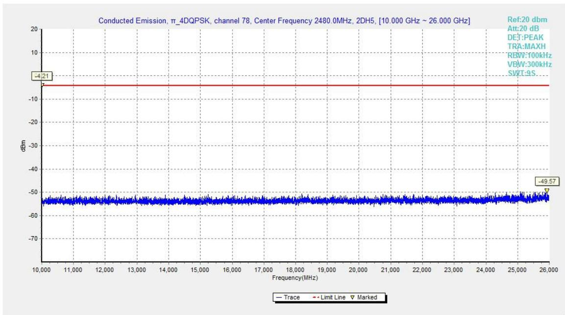
Fig.63. Conducted spurious emission:  $\pi/4$  DQPSK, Channel 78, 10GHz - 26GHz
