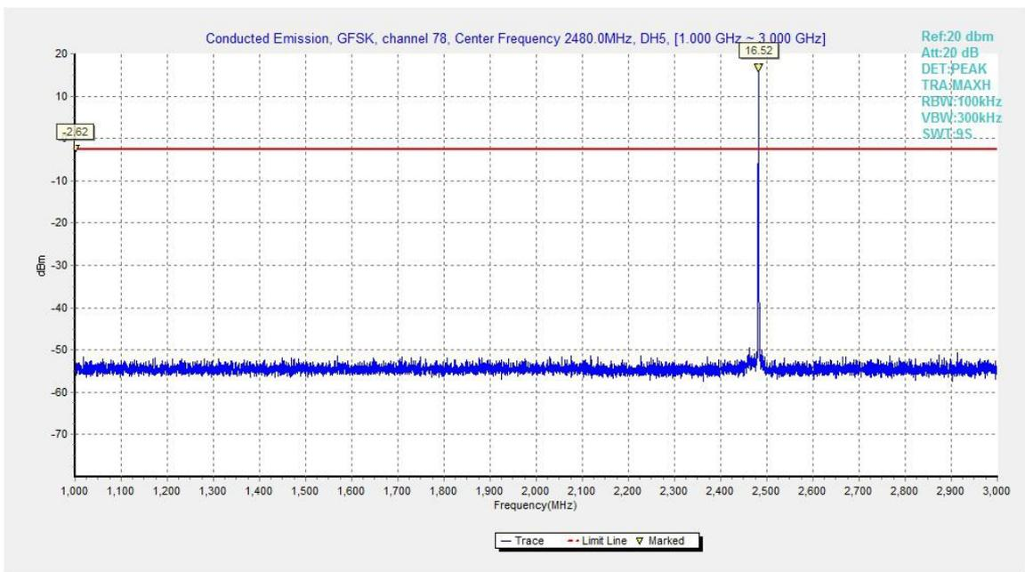
Fig.46. Conducted spurious emission: GFSK, Channel 78, 1GHz - 3GHz
