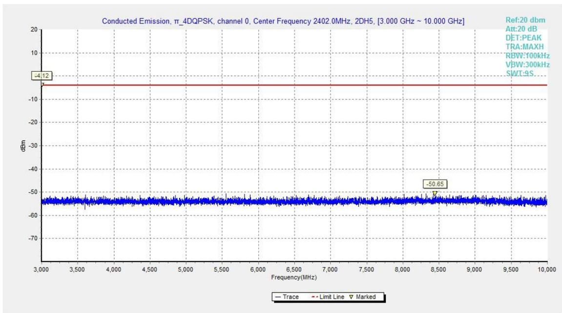
Fig.52. Conducted spurious emission:  $\pi/4$  DQPSK, Channel 0, 3GHz - 10GHz
