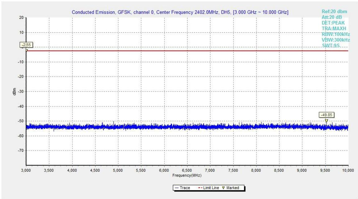
Fig.37. Conducted spurious emission: GFSK, Channel 0, 3GHz - 10GHz
