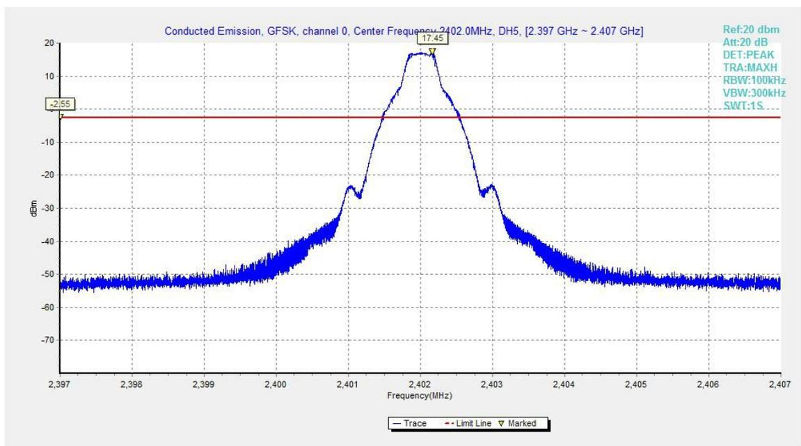
Fig.34. Conducted spurious emission: GFSK, Channel 0,2402MHz
