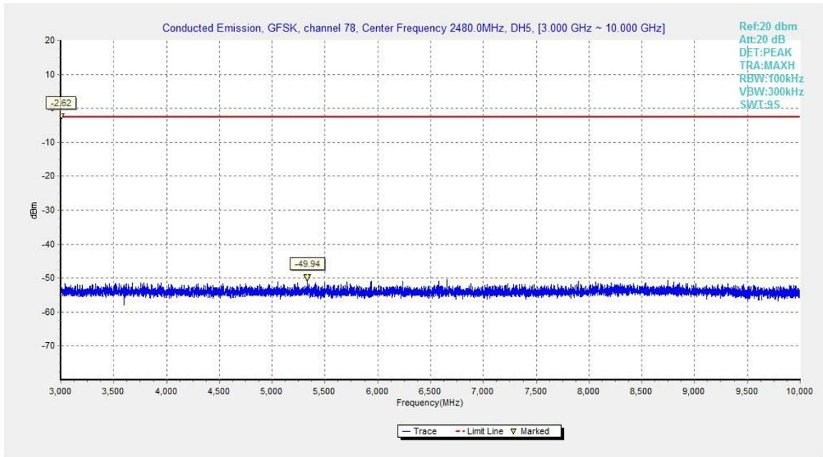
Fig.47. Conducted spurious emission: GFSK, Channel 78, 3GHz - 10GHz
