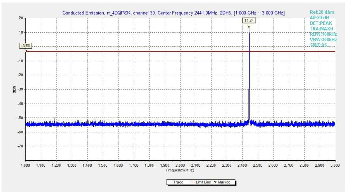
Fig.56. Conducted spurious emission:  $\pi/4$  DQPSK, Channel 39, 1GHz - 3GHz
