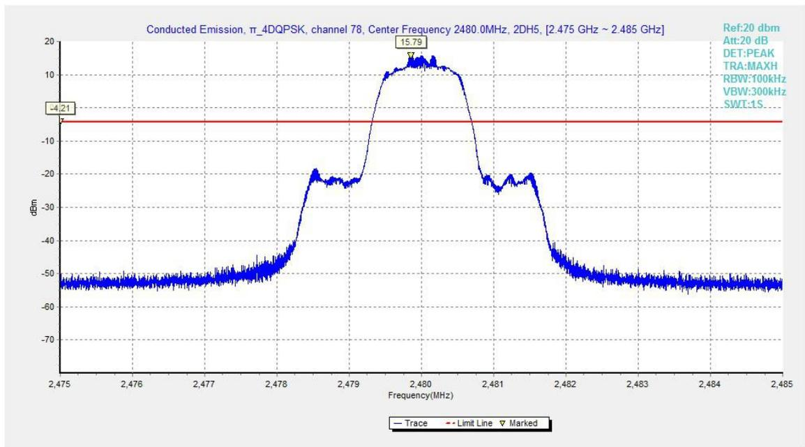
Fig.59. Conducted spurious emission:  $\pi/4$  DQPSK, Channel 78, 2480MHz
