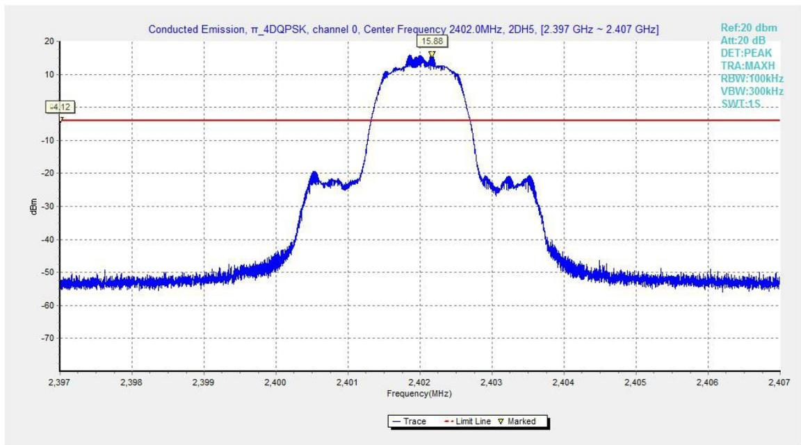
Fig.49. Conducted spurious emission:  $\pi/4$  DQPSK, Channel 0,2402MHz
