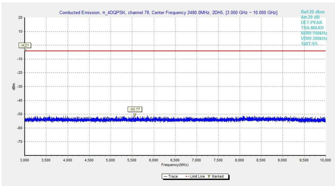
Fig.62. Conducted spurious emission:  $\pi/4$  DQPSK, Channel 78, 3GHz - 10GHz
