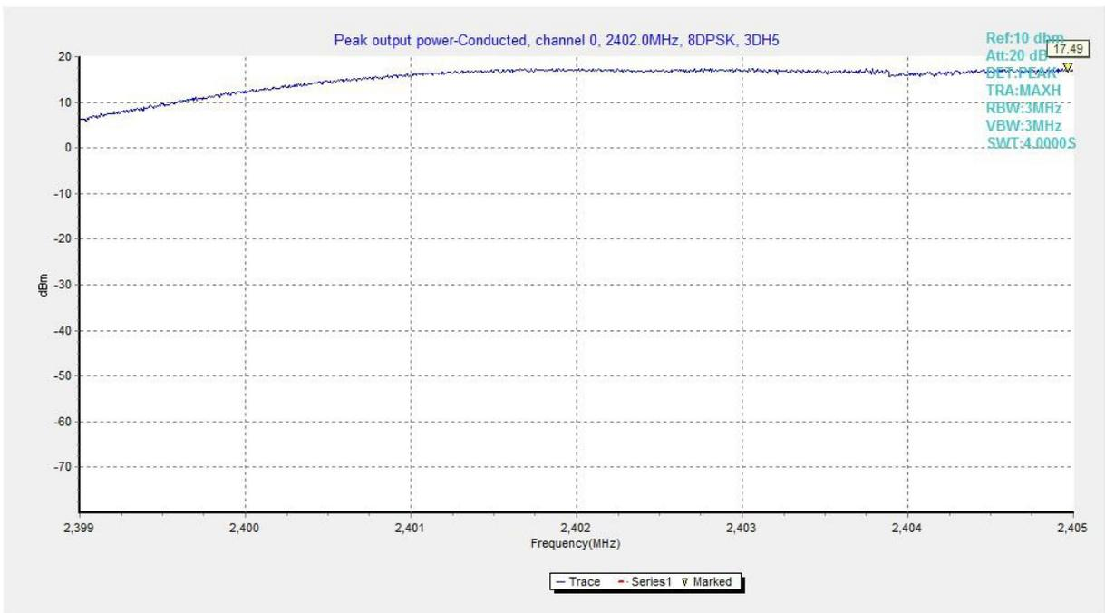
Fig.7. Peak Output Power -Conducted: Antenna 3, 8DPSK, Channel 0,
