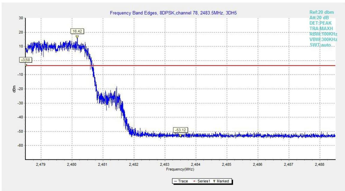
Fig.21. Frequency Band Edges: 8DPSK, Channel 78, Hopping On
