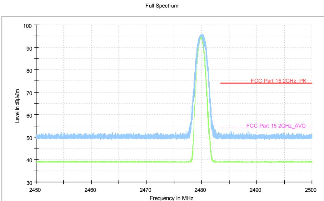
**Fig.25. Frequency Band Edges: EUT3 ANT3  $\pi/4$  DQPSK, Channel 78, Hopping Off, 2.38 GHz - 2.45GHz**
