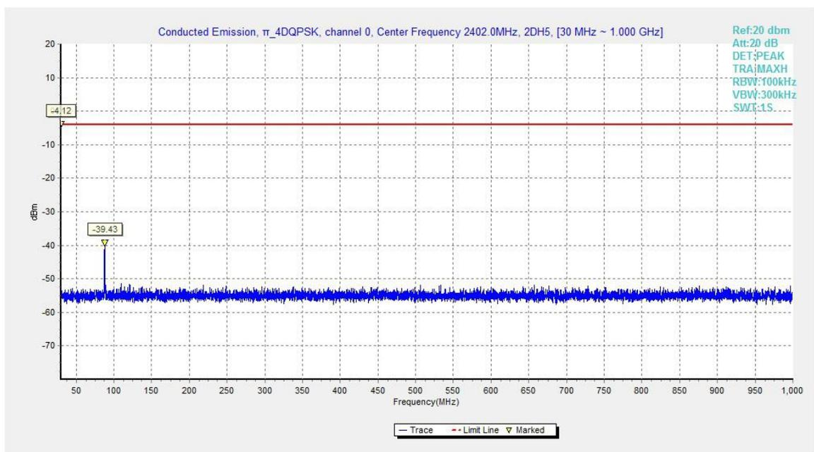
Fig.50. Conducted spurious emission:  $\pi/4$  DQPSK, Channel 0, 30MHz - 1GHz
