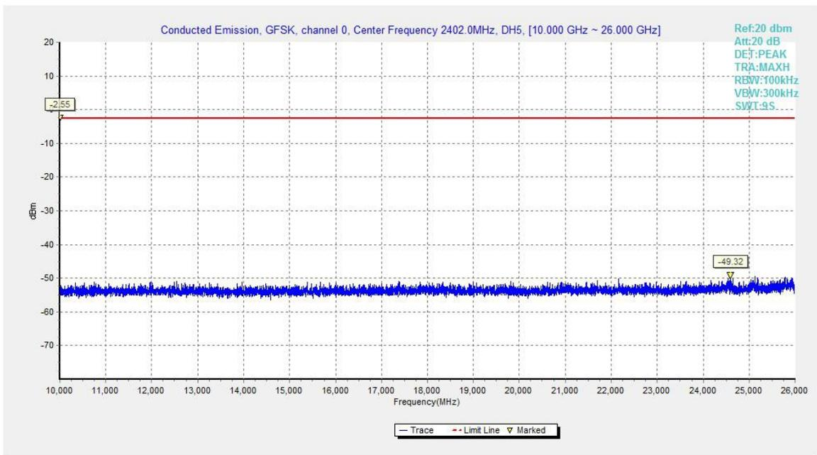
Fig.38. Conducted spurious emission: GFSK, Channel 0, 10GHz - 26GHz
