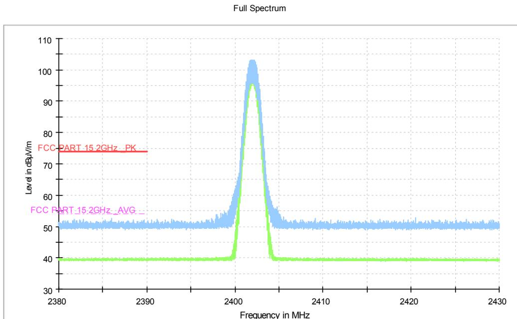
**Fig.28. Frequency Band Edges: EUT4 ANT4 GFSK, Channel 0, Hopping Off, 2.38 GHz – 2.45GHz**
