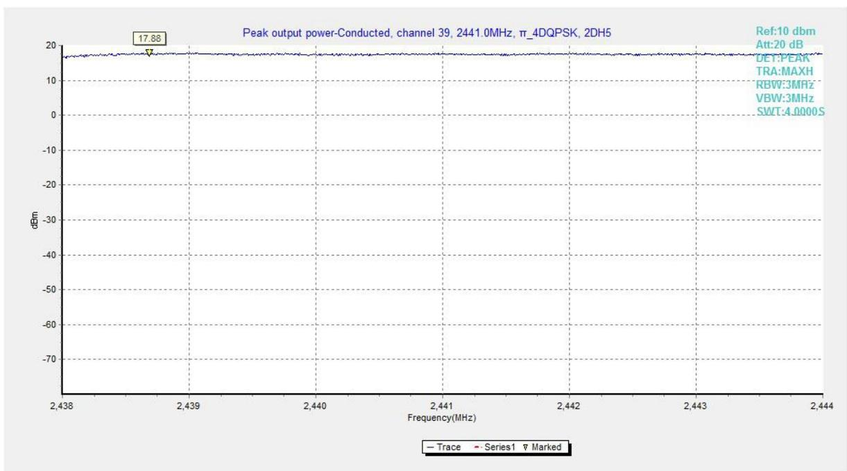
Fig.5. Peak Output Power -Conducted: Antenna 3,  $\pi/4$  DQPSK, Channel 39,
