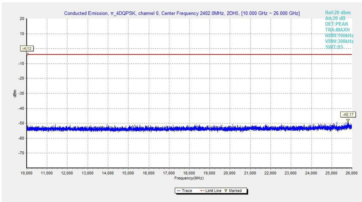
Fig.53. Conducted spurious emission:  $\pi/4$  DQPSK, Channel 0, 10GHz - 26GHz
