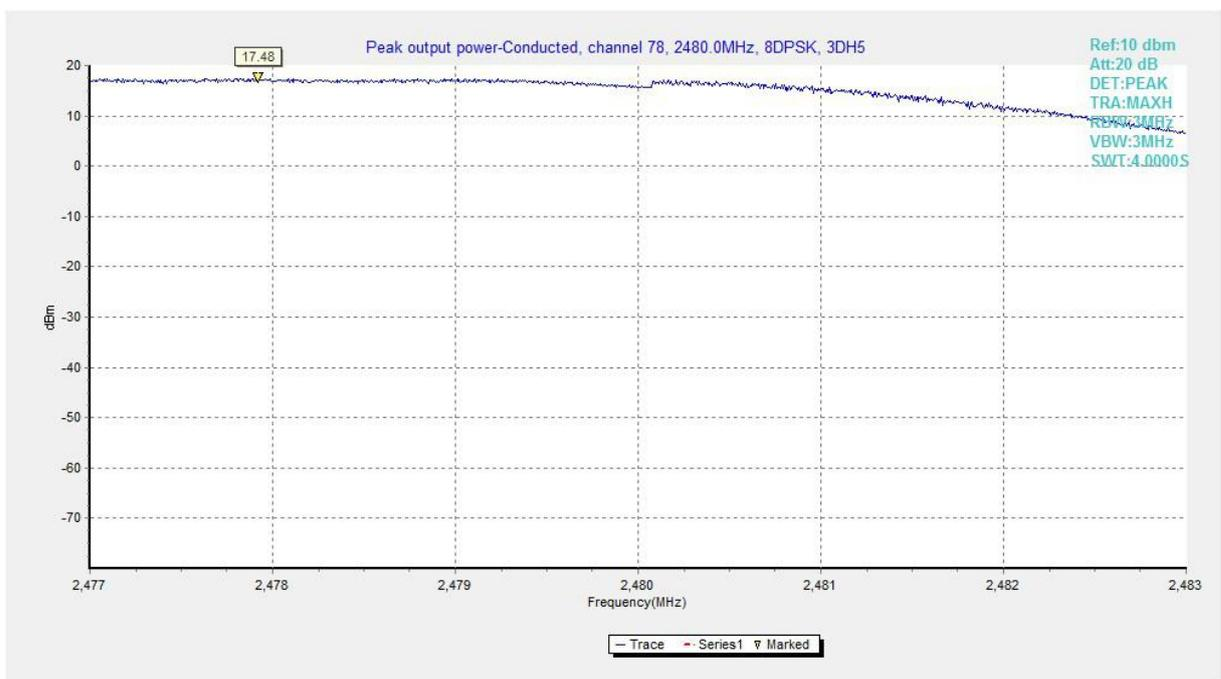
Fig.9. Peak Output Power -Conducted: Antenna 3, 8DPSK, Channel 78,
