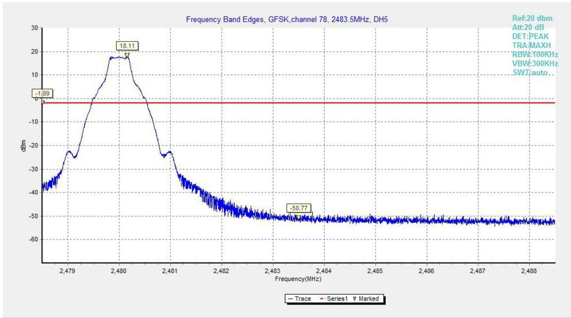
Fig.12. Frequency Band Edges: GFSK, Channel 78, Hopping Off
