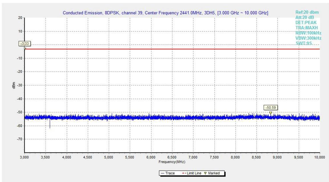
Fig.72. Conducted spurious emission: 8DPSK, Channel 39, 3GHz - 10GHz
