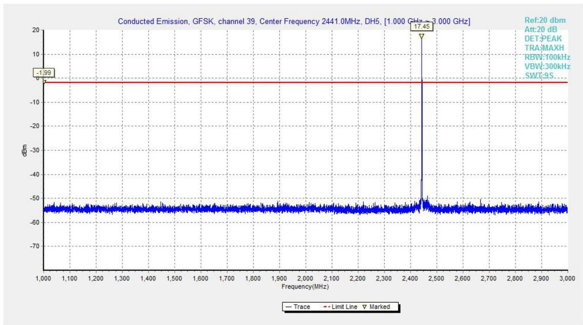
Fig.41. Conducted spurious emission: GFSK, Channel 39, 1GHz – 3GHz
