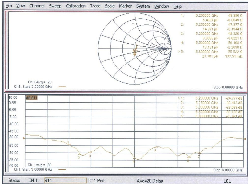
Impedance Measurement Plot for Body TSL (5750, 5800 MHz)
