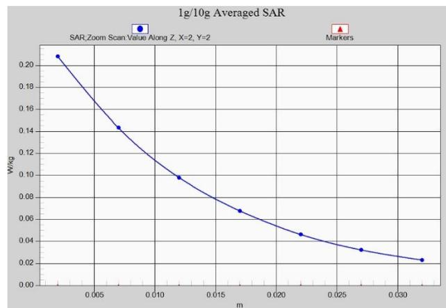
**Fig. 1-24 Z-Scan at power reference point (WCDMA1900)**
