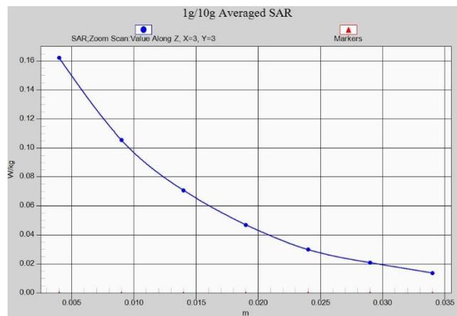
**Fig. 1-27 Z-Scan at power reference point (WCDMA1700)**
