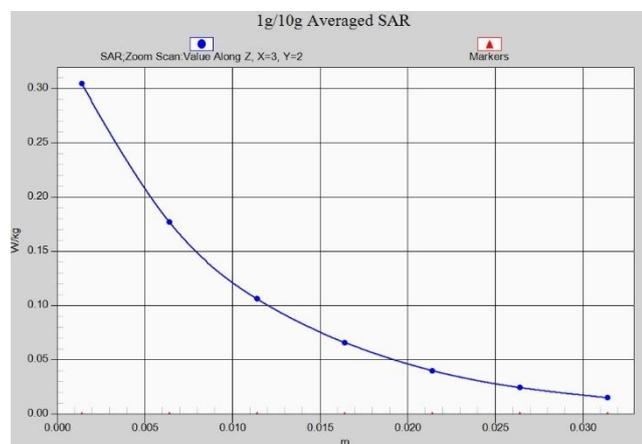
**Fig. 1-23 Z-Scan at power reference point (PCS1900)**
