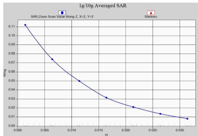
**Fig. 1-21 Z-Scan at power reference point (PCS1900)**
