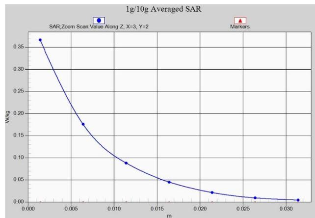
**Fig. 1-45 Z-Scan at power reference point (LTE Band38)**
