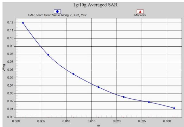
**Fig. 1-40 Z-Scan at power reference point (LTE Band 7)**
