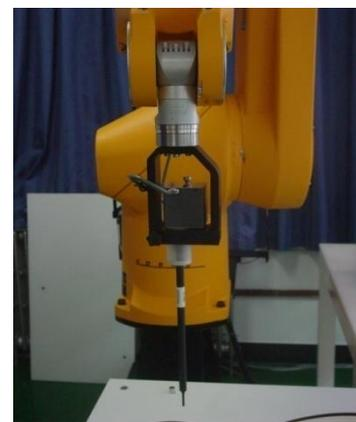
Picture C.3 E-field Probe
