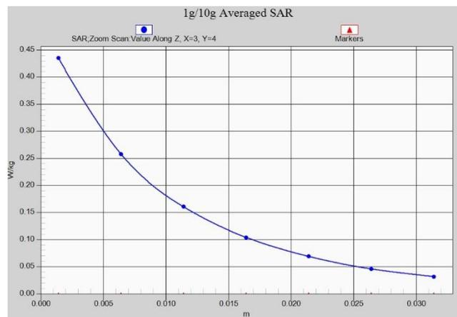
**Fig. 1-39 Z-Scan at power reference point (LTE Band5)**
