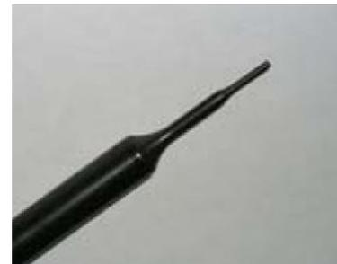
Picture C.2 Near-field Probe
