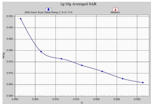
**Fig. 1-25 Z-Scan at power reference point (WCDMA1900)**
