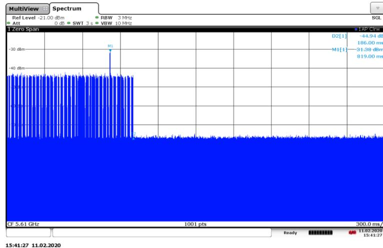
**Fig.A.5 channel closing transmission time**
