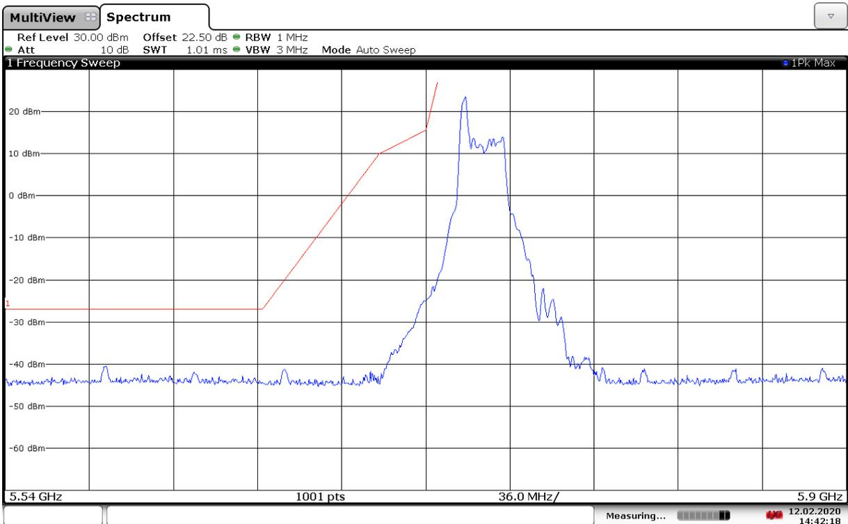
**Fig. 151 Band Edges (802.11ax-HE20-RU26-left, 5745MHz)**
