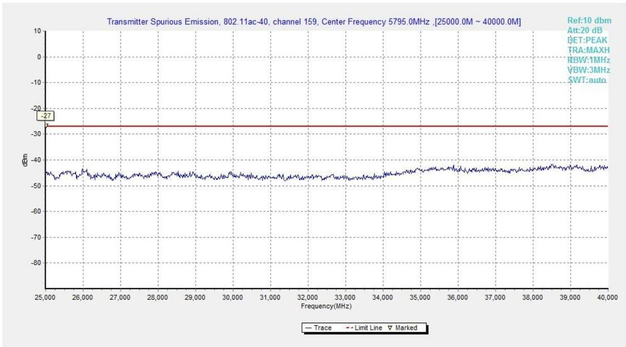
**Fig. 54 Conducted Spurious Emission (802.11ac-HT40, Ch159, 25 GHz-40 GHz)**
