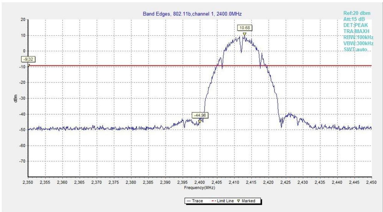
**Fig.A.5.17 Band Edges (802.11b, Ch 1)**
