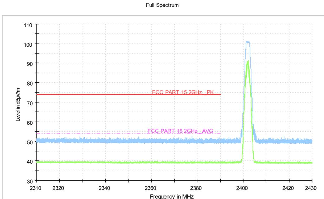
**Fig.9. Frequency Band Edges: EUT4 ANT4 BLE 5.0 GFSK, 2402 MHz, Hopping Off, 2.38 GHz – 2.45GHz**
