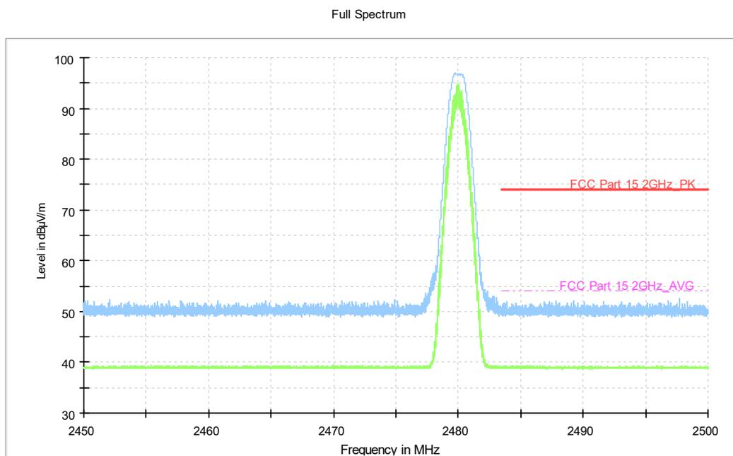
**Fig.8. Frequency Band Edges: EUT4 ANT4 BLE 4.0 GFSK, 2480 MHz, Hopping Off , 2.45 GHz - 2.50GHz**
