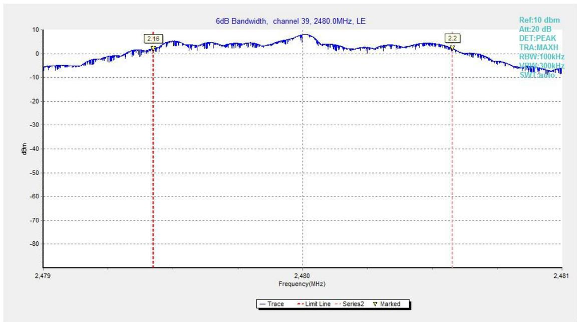
**Fig.28.** 6dB Bandwidth: GFSK, 2480 MHz
