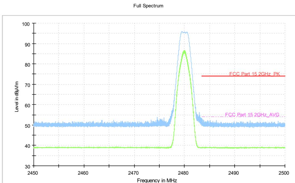
**Fig.6. Frequency Band Edges: EUT3 ANT3 BLE 5.0 GFSK, 2480 MHz, Hopping Off , 2.45 GHz - 2.50GHz**
