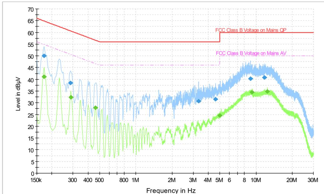
**Fig.A.9.2 AC Powerline Conducted Emission-Idle EUT3(M2001J2G)+AE1+AE3+AE6**
