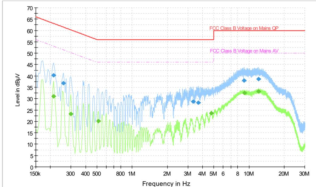
**Fig.A.9.1 AC Powerline Conducted Emission- Bluetooth EUT3(M2001J2G)+AE1+AE3+AE6**
