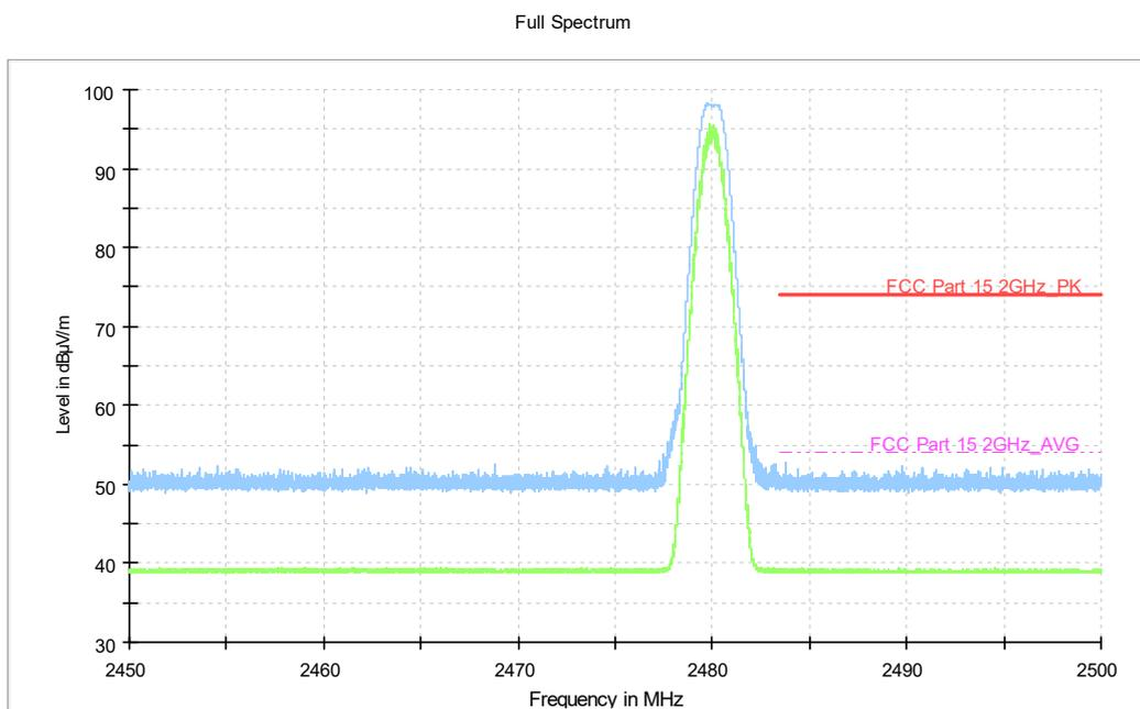
**Fig.4. Frequency Band Edges: EUT3 ANT3 BLE 4.0GFSK, 2480 MHz, Hopping Off , 2.45 GHz - 2.50GHz**
