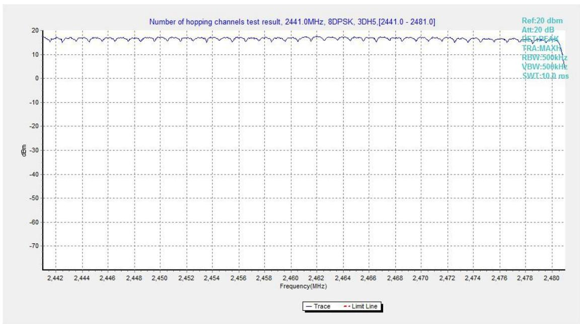
Fig.114. Number of hopping frequencies: 8DPSK, Channel 40 - 78
