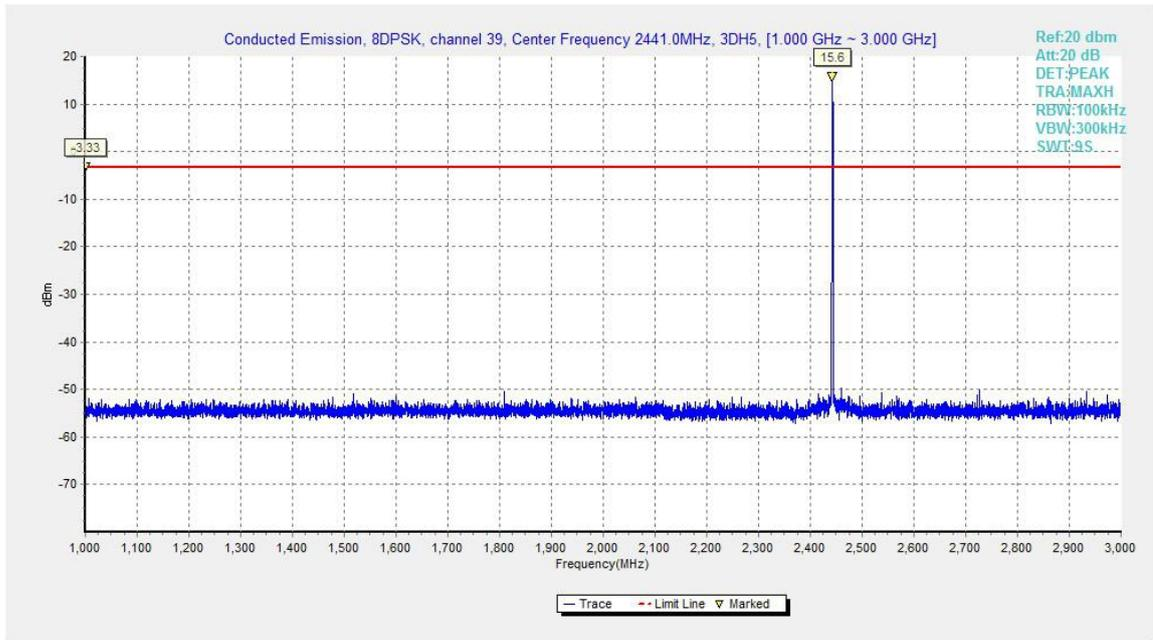
Fig.71. Conducted spurious emission: 8DPSK, Channel 39, 1GHz - 3GHz
