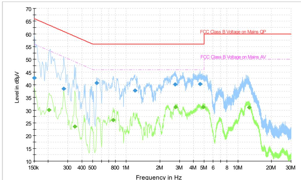
**Fig.A.11.3 AC Powerline Conducted Emission- Bluetooth
