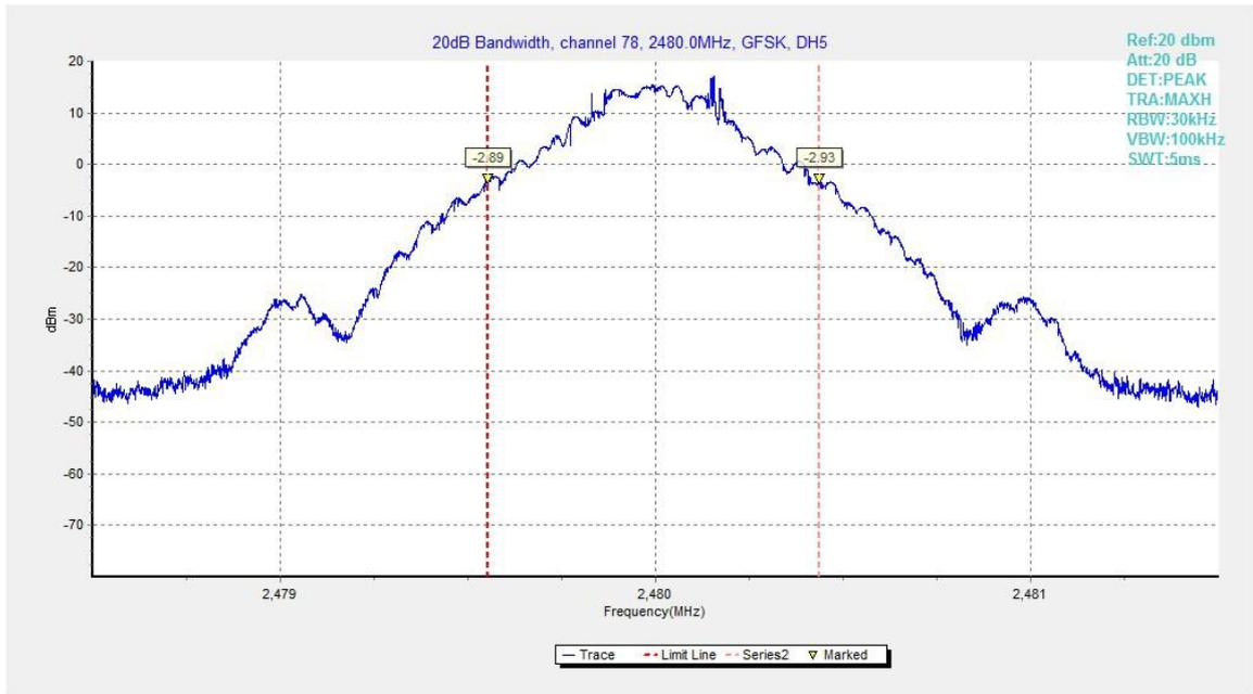
Fig.99. 20dB Bandwidth: GFSK, Channel 78
