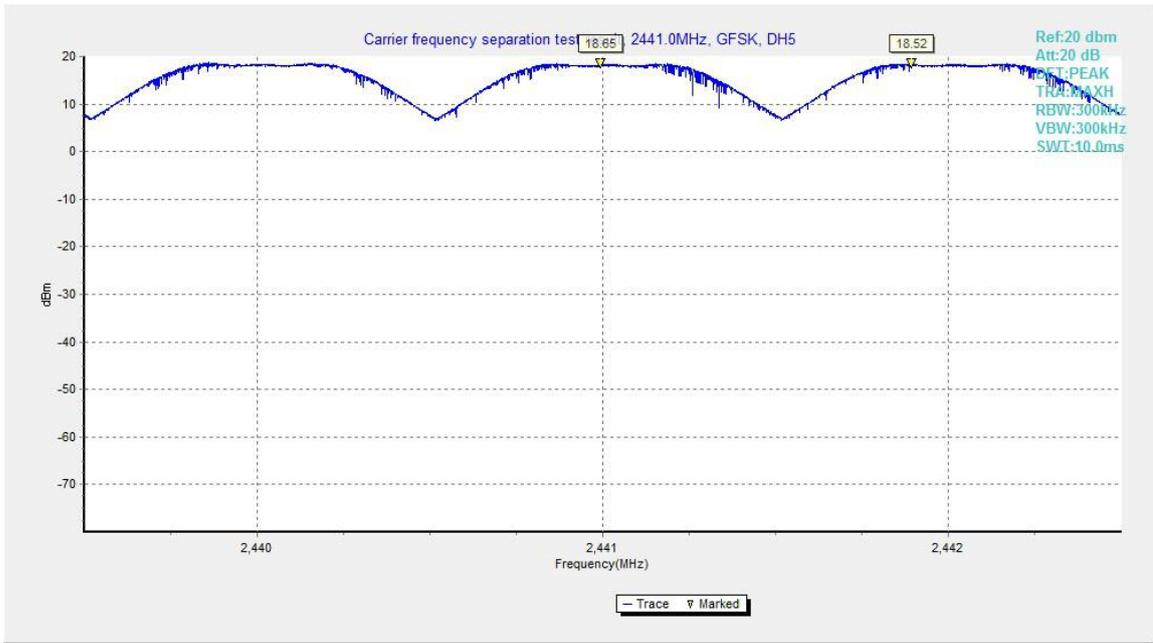
Fig.106. Carrier frequency separation measurement: GFSK, Channel 39
