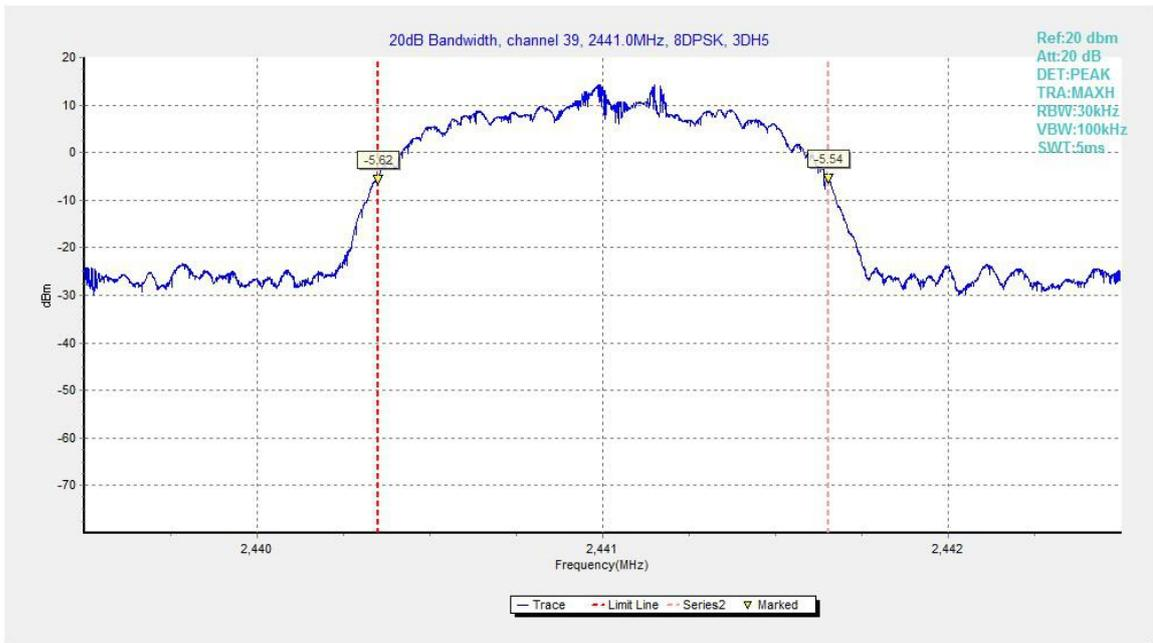
Fig.104. 20dB Bandwidth: 8DPSK, Channel 39
