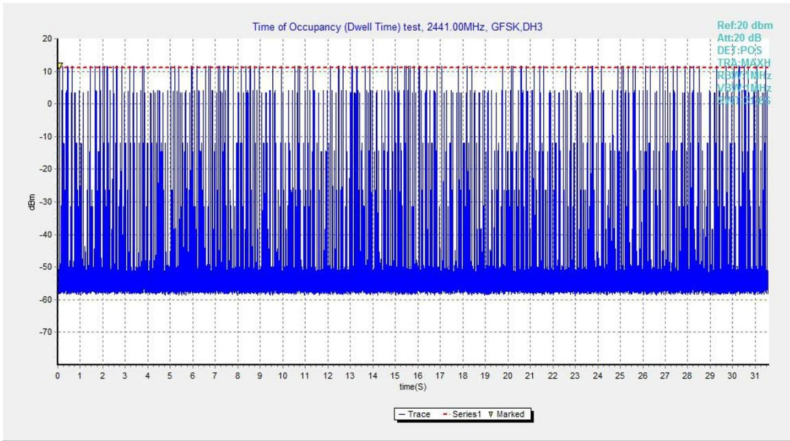
Fig.82. Number of Transmissions Measurement: Channel 39,Packet DH3
