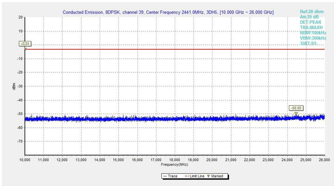
Fig.73. Conducted spurious emission: 8DPSK, Channel 39, 10GHz – 26GHz
