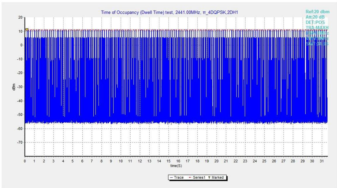
Fig.86. Number of Transmissions Measurement: Channel 39,Packet 2-DH1
