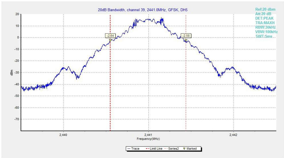
Fig.98. 20dB Bandwidth: GFSK, Channel 39
