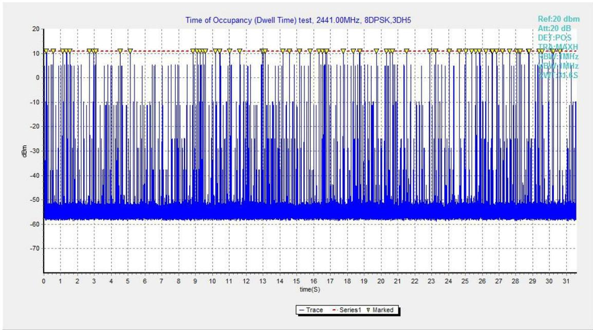
Fig.96. Number of Transmissions Measurement: Channel 39,Packet 3-DH5
