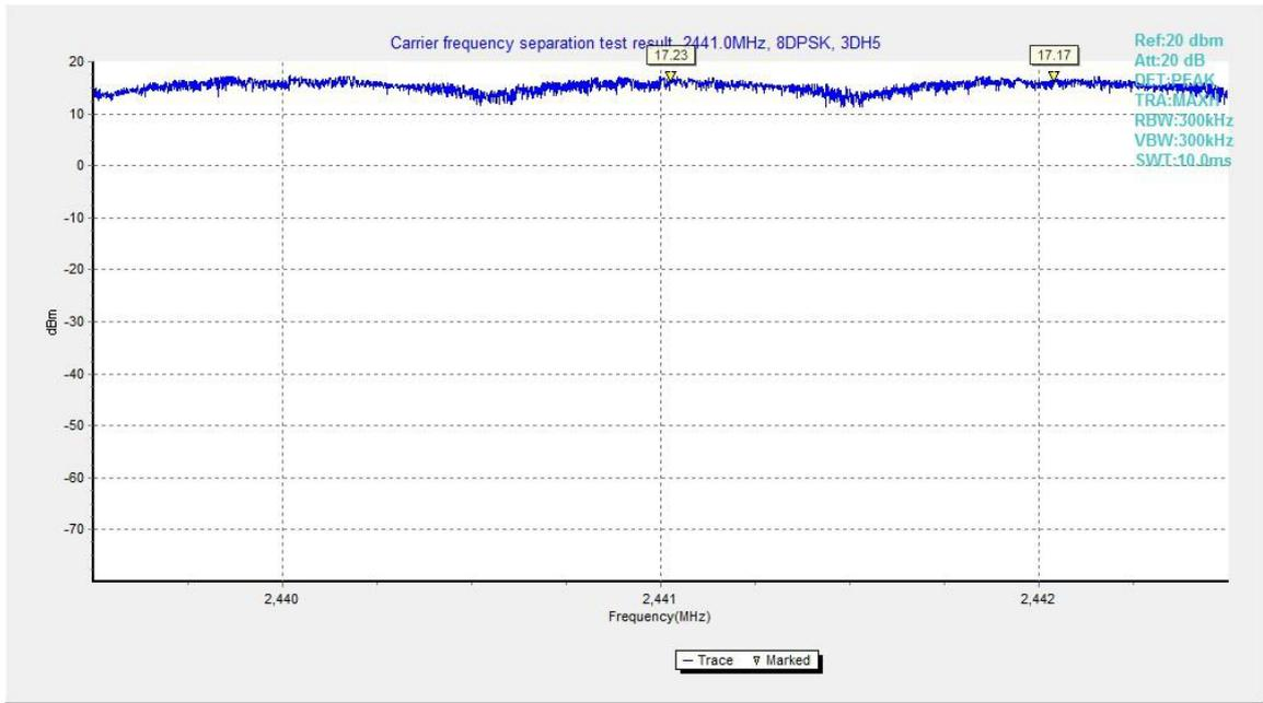
Fig.108. Carrier frequency separation measurement: 8DPSK, Channel 39
