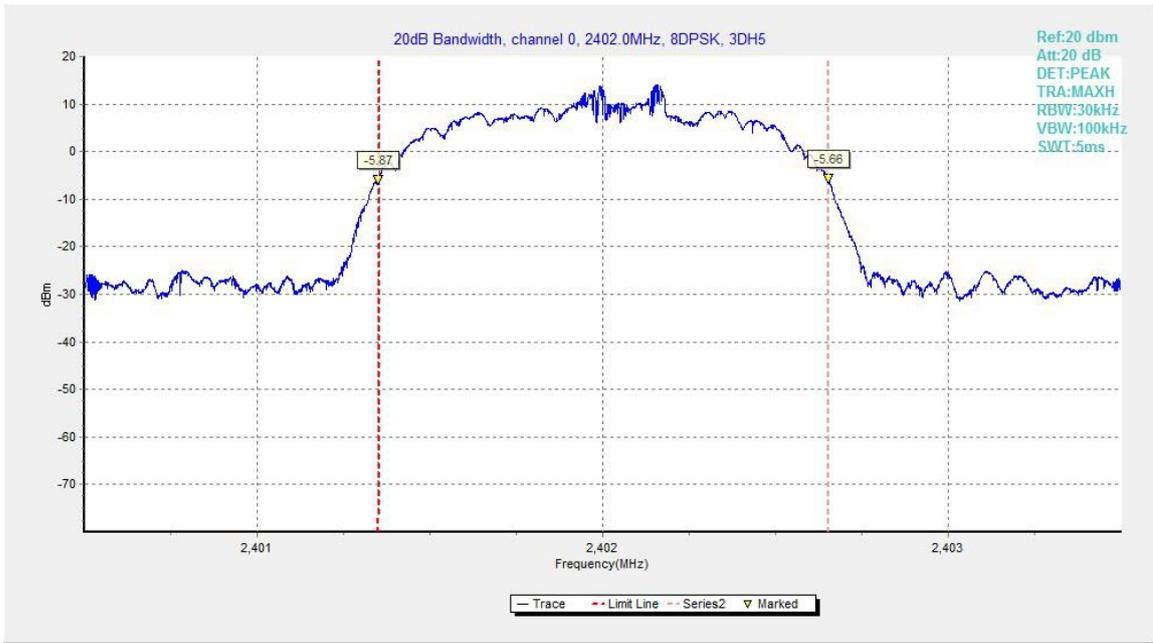
Fig.103. 20dB Bandwidth: 8DPSK, Channel 0
