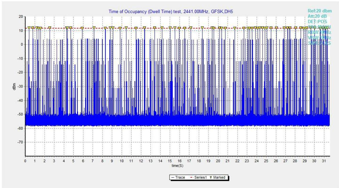
Fig.84. Number of Transmissions Measurement: Channel 39,Packet DH5
