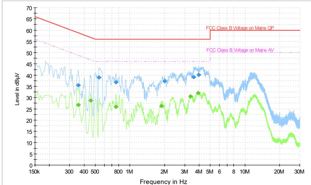
**Fig.A.11.4 AC Powerline Conducted Emission-Idle
