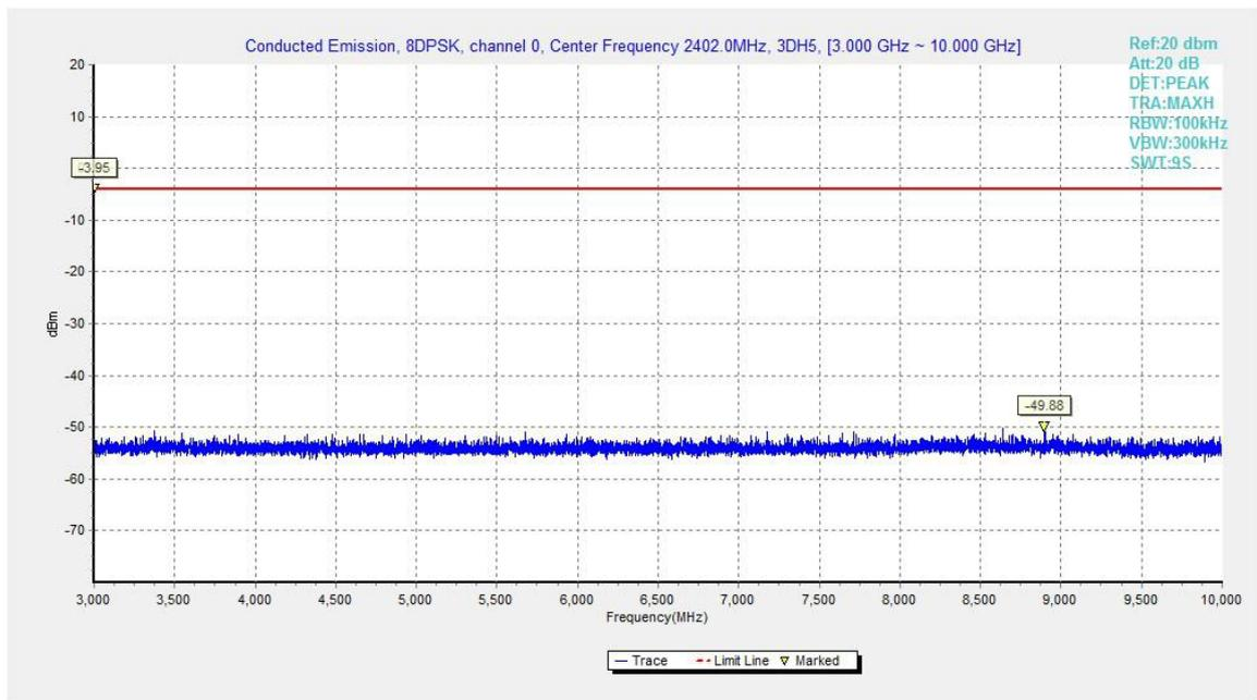
Fig.67. Conducted spurious emission: 8DPSK, Channel 0, 3GHz - 10GHz
