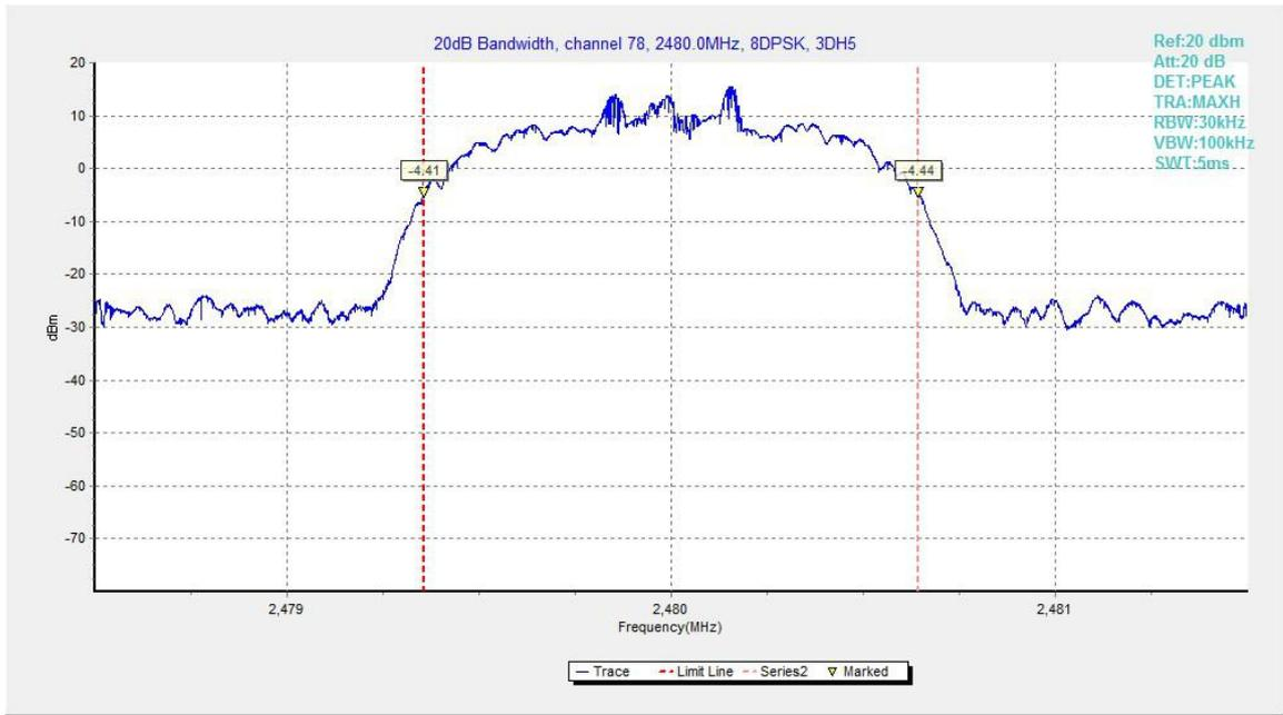
Fig.105. 20dB Bandwidth: 8DPSK, Channel 78
