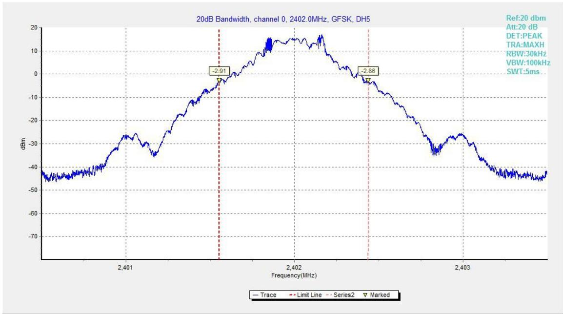
Fig.97. 20dB Bandwidth: GFSK, Channel 0
