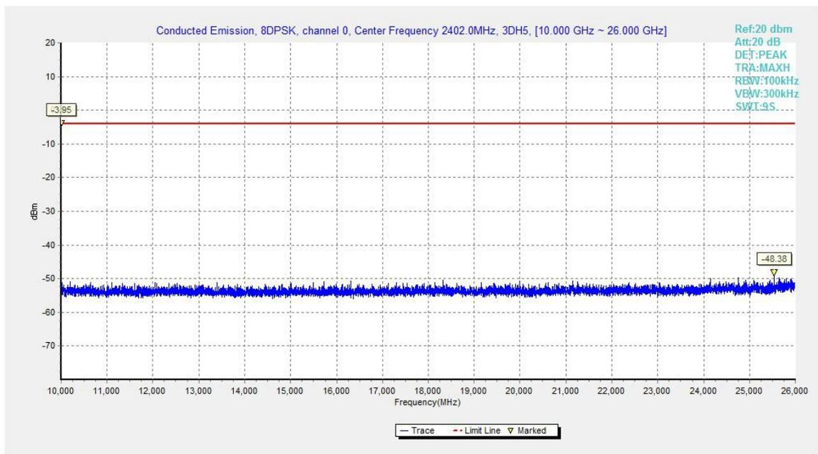
Fig.68. Conducted spurious emission: 8DPSK, Channel 0, 10GHz - 26GHz
