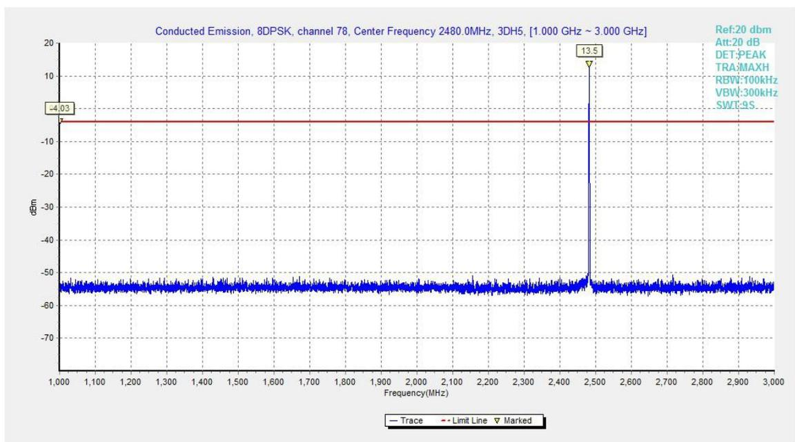
Fig.76. Conducted spurious emission: 8DPSK, Channel 78, 1GHz - 3GHz
