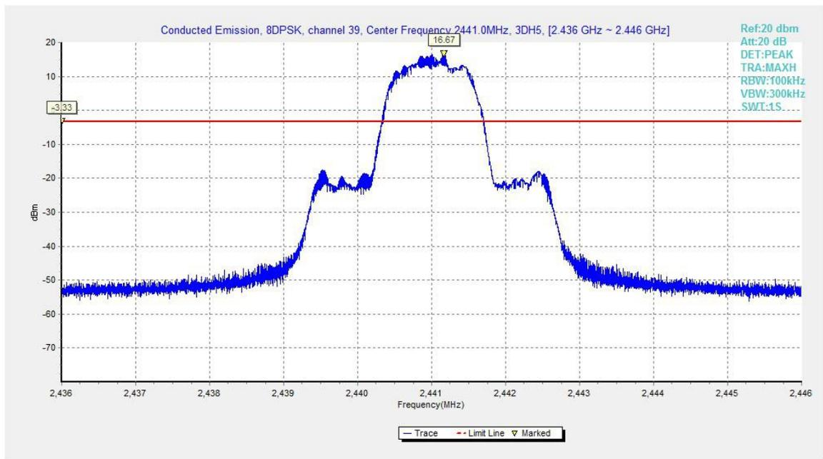
Fig.69. Conducted spurious emission: 8DPSK, Channel 39, 2441MHz
