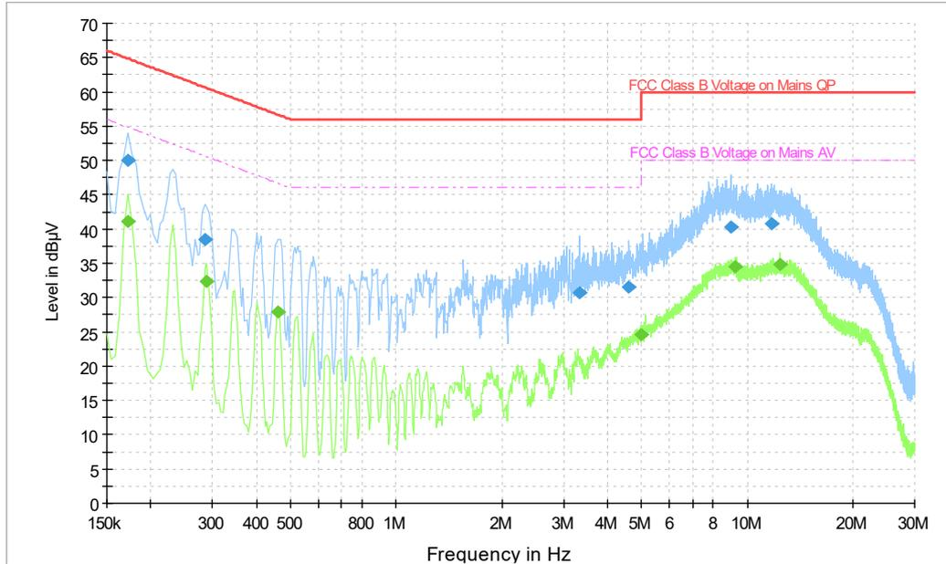
**Fig.A.11.2 AC Powerline Conducted Emission-Idle EUT3(M2001J2G)+AE1+AE3+AE6**
