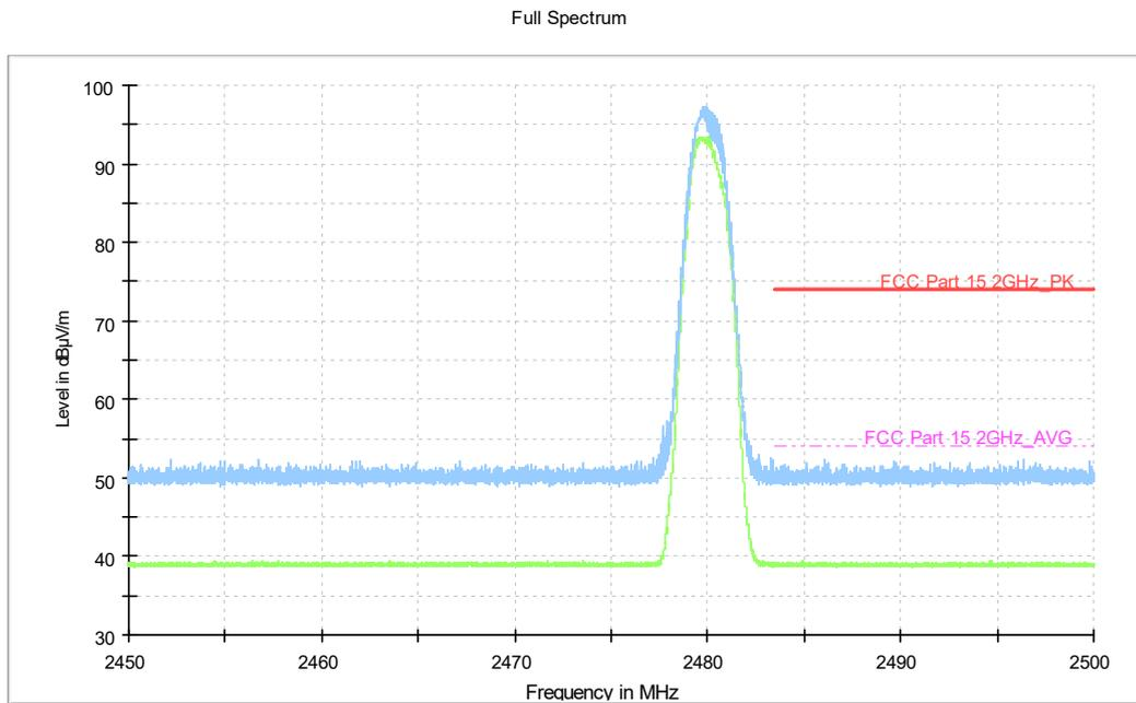
**Fig.33. Frequency Band Edges: EUT4 ANT4 8DPSK, Channel 78, 2.38 GHz - 2.45GHz**
