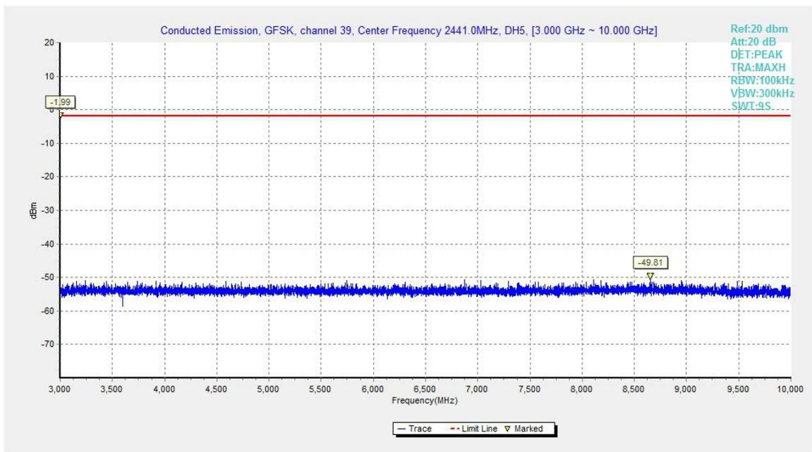
Fig.42. Conducted spurious emission: GFSK, Channel 39, 3GHz – 10GHz
