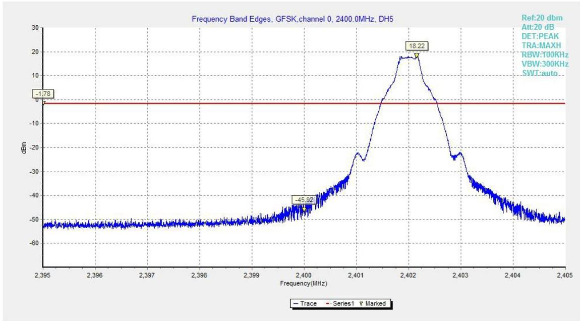
Fig.10. Frequency Band Edges: GFSK, Channel 0, Hopping Off
