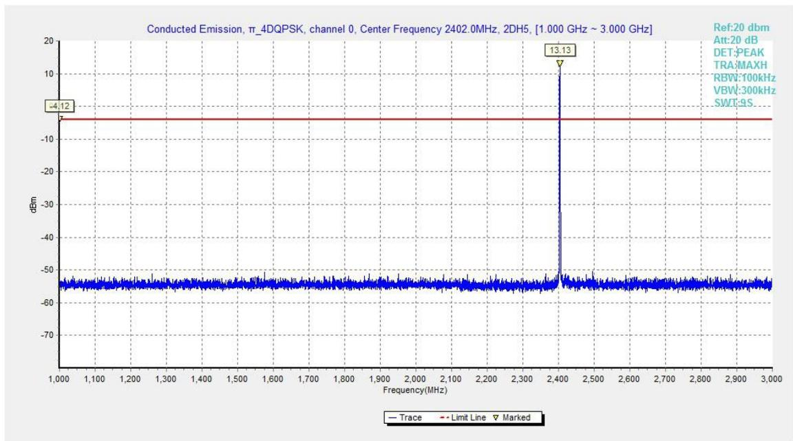
Fig.51. Conducted spurious emission:  $\pi/4$  DQPSK, Channel 0, 1GHz - 3GHz
