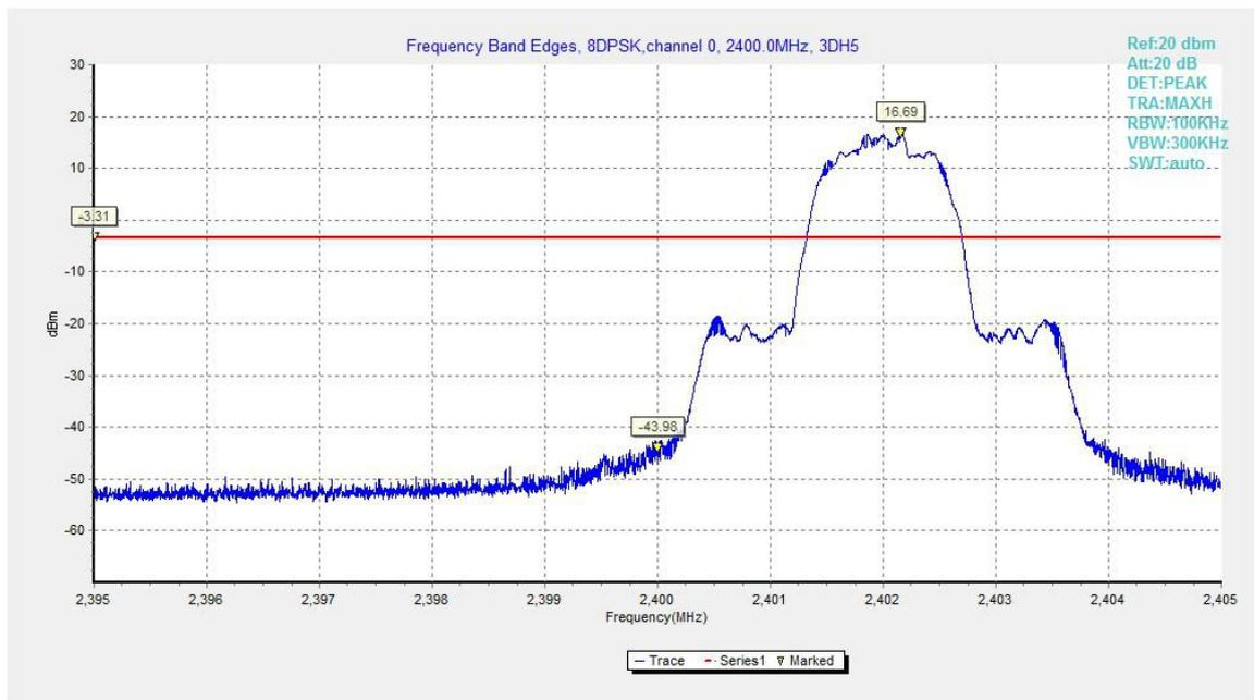
Fig.18. Frequency Band Edges: 8DPSK, Channel 0, Hopping Off
