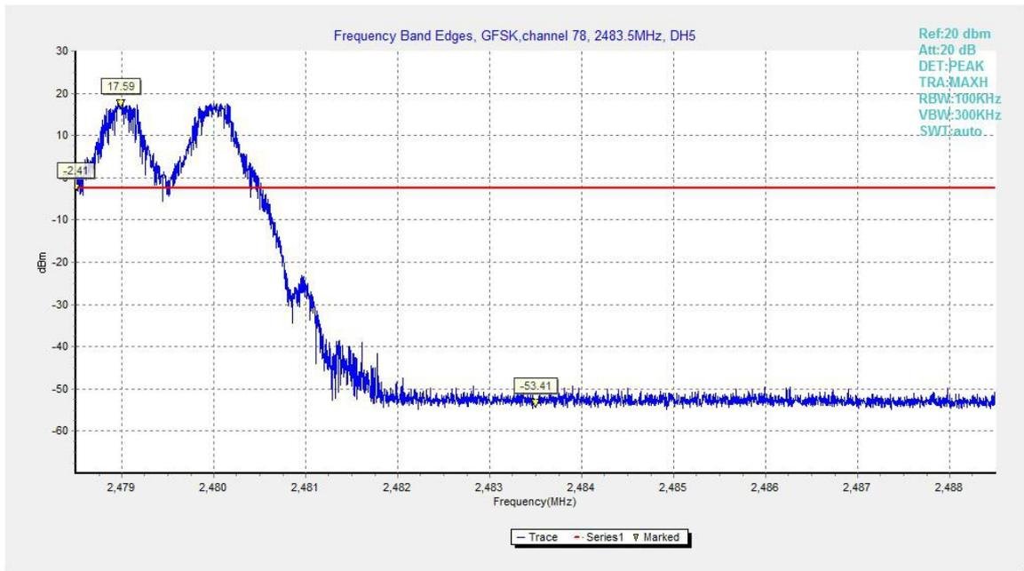
Fig.13. Frequency Band Edges: GFSK, Channel 78, Hopping On
