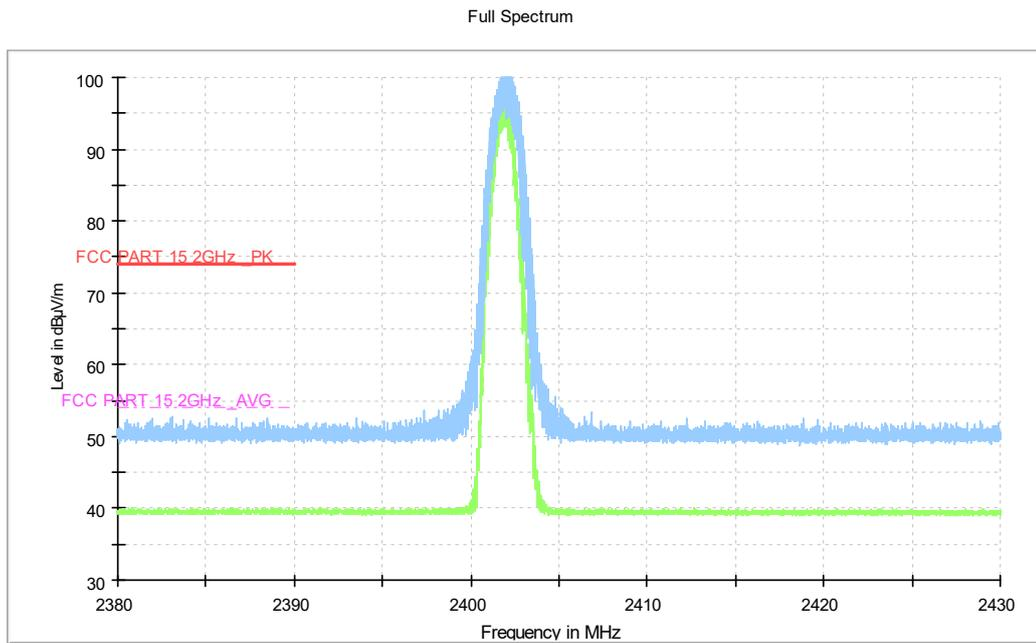
**Fig.24. Frequency Band Edges: EUT3 ANT3  $\pi/4$  DQPSK, Channel 0, Hopping Off, 2.38 GHz - 2.45GHz**
