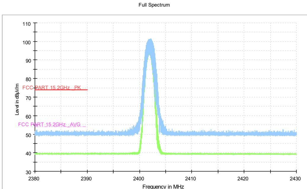
**Fig.30. Frequency Band Edges: EUT4 ANT4  $\pi/4$  DQPSK, Channel 0, Hopping Off, 2.38 GHz - 2.45GHz**
