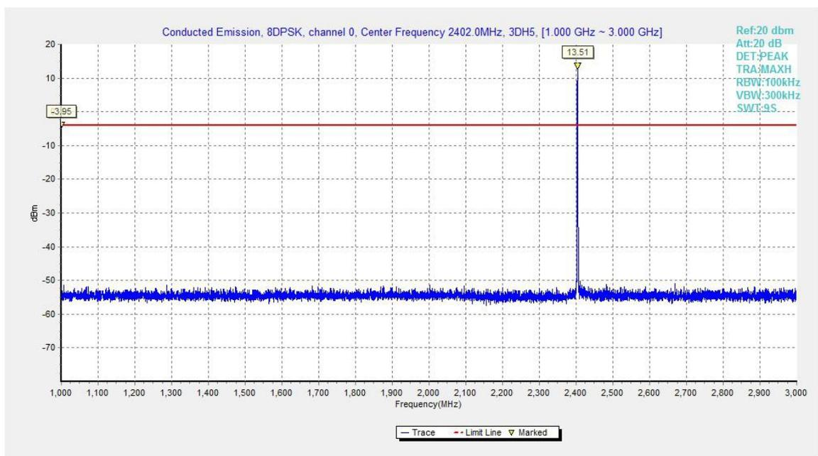
Fig.66. Conducted spurious emission: 8DPSK, Channel 0, 1GHz - 3GHz
