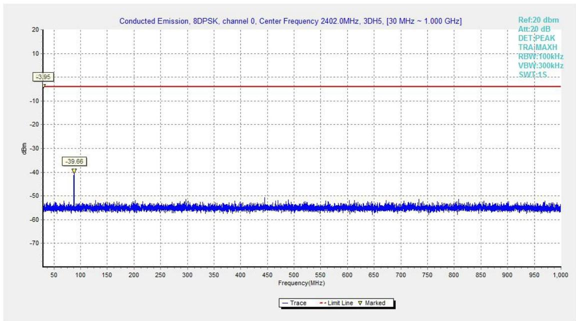
Fig.65. Conducted spurious emission: 8DPSK, Channel 0, 30MHz - 1GHz
