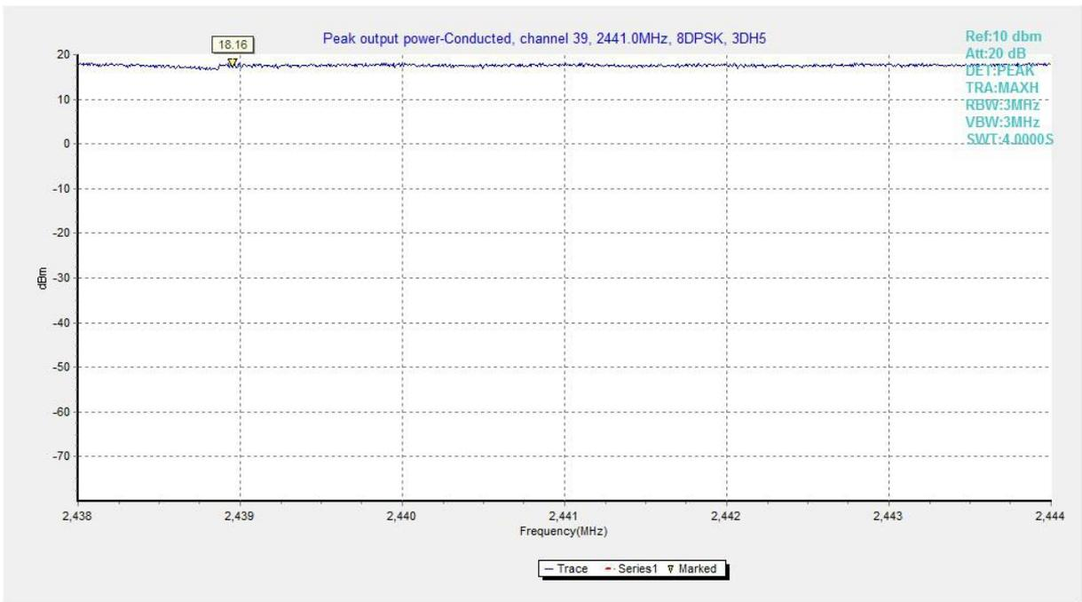
Fig.8. Peak Output Power -Conducted: Antenna 3, 8DPSK, Channel 39,
