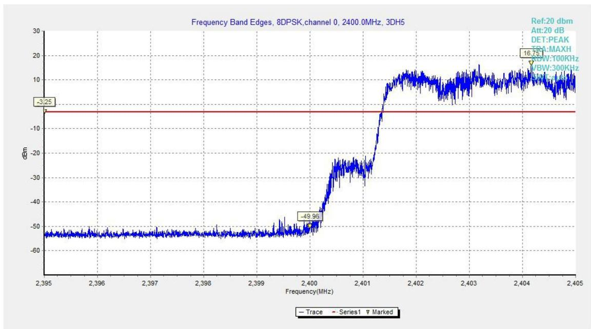
Fig.19. Frequency Band Edges: 8DPSK, Channel 0, Hopping On
