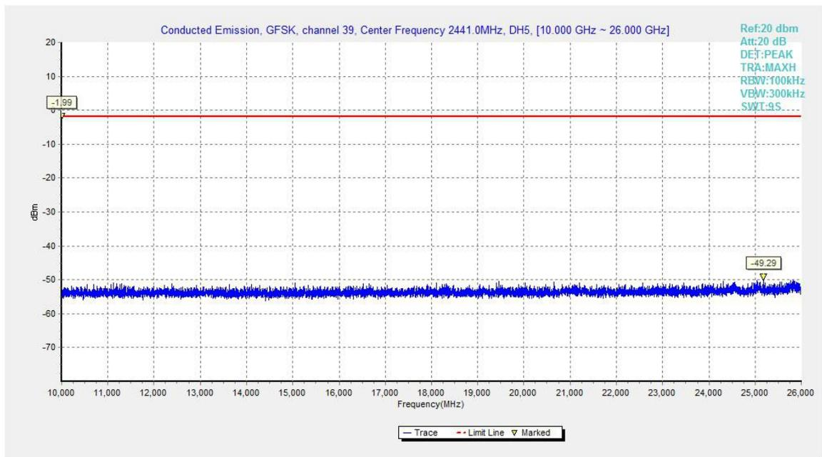
Fig.43. Conducted spurious emission: GFSK, Channel 39, 10GHz – 26GHz
