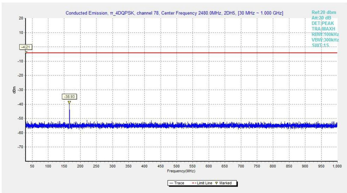
Fig.60. Conducted spurious emission:  $\pi/4$  DQPSK, Channel 78, 30MHz - 1GHz
