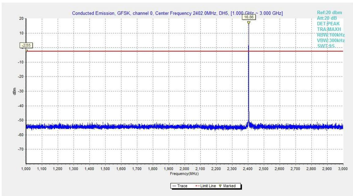
Fig.36. Conducted spurious emission: GFSK, Channel 0, 1GHz - 3GHz
