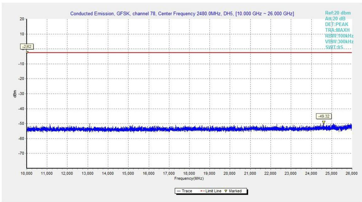
Fig.48. Conducted spurious emission: GFSK, Channel 78, 10GHz - 26GHz
