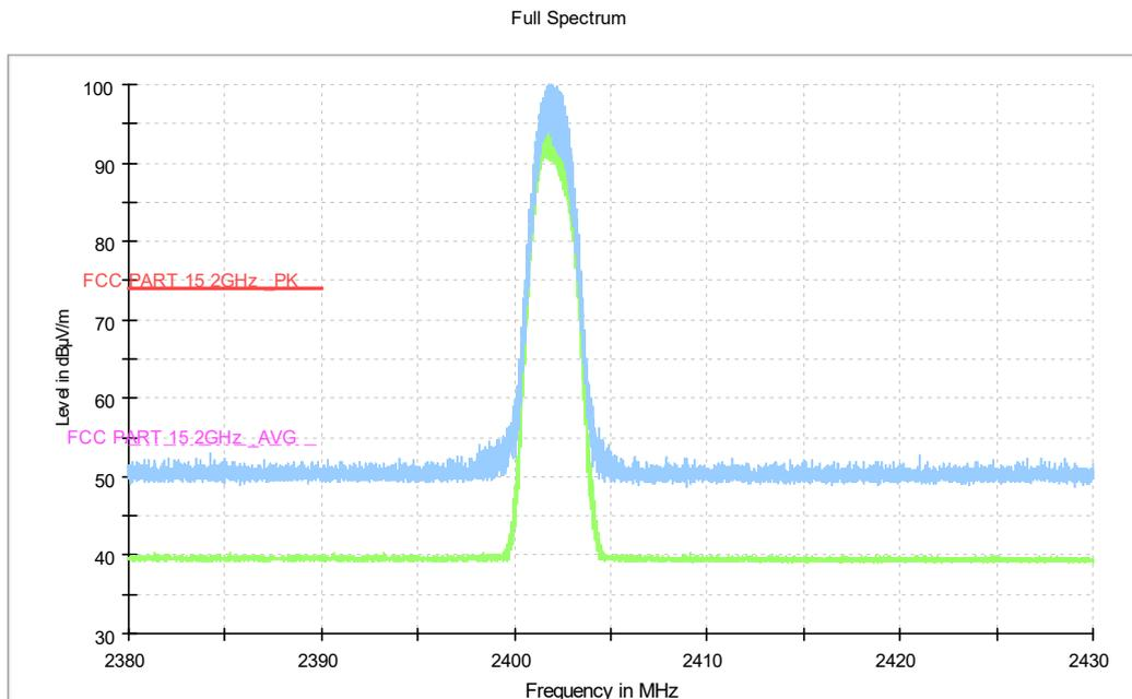
**Fig.26. Frequency Band Edges: EUT3 ANT3 DPSK, Channel 0, 2.38 GHz - 2.45GHz**
