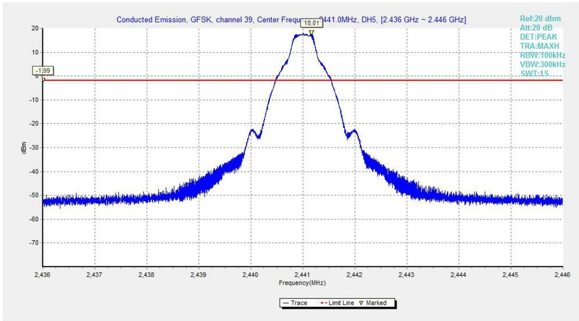
Fig.39. Conducted spurious emission: GFSK, Channel 39, 2441MHz
