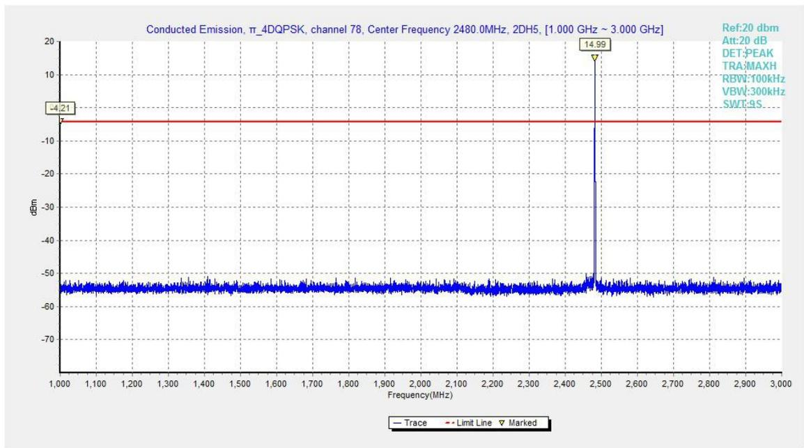
Fig.61. Conducted spurious emission:  $\pi/4$  DQPSK, Channel 78, 1GHz - 3GHz
