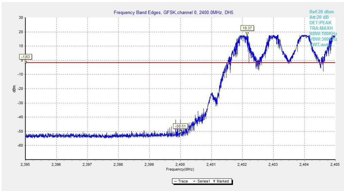
Fig.11. Frequency Band Edges: GFSK, Channel 0, Hopping On
