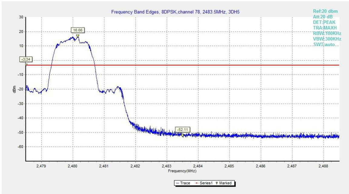
Fig.20. Frequency Band Edges: 8DPSK, Channel 78, Hopping Off
