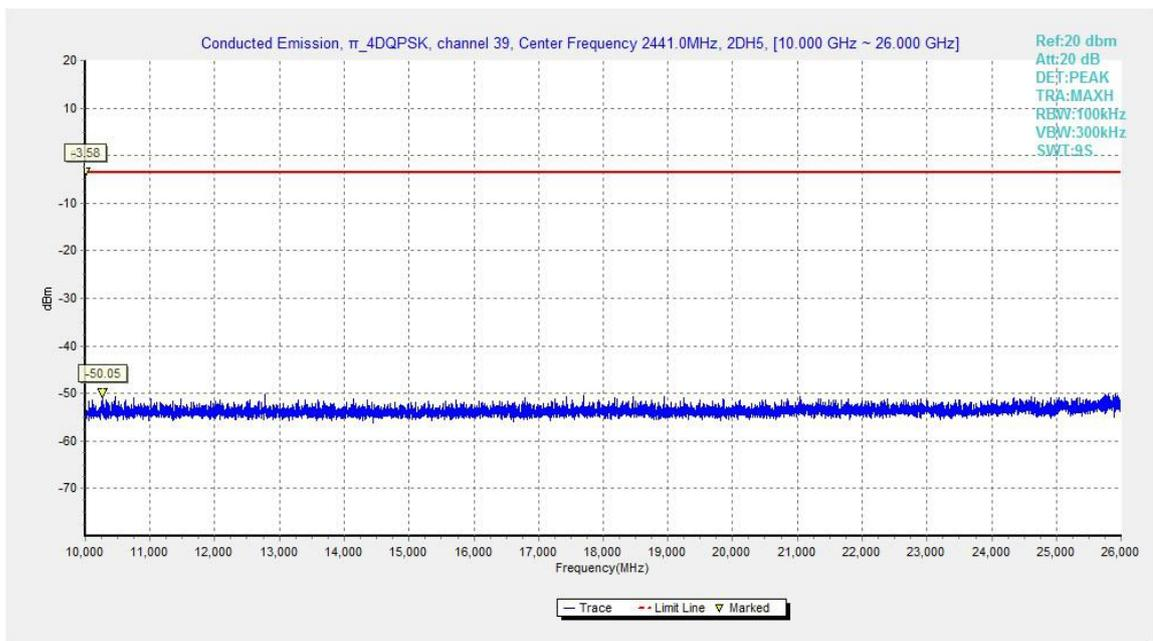
Fig.58. Conducted spurious emission:  $\pi/4$  DQPSK, Channel 39, 10GHz – 26GHz
