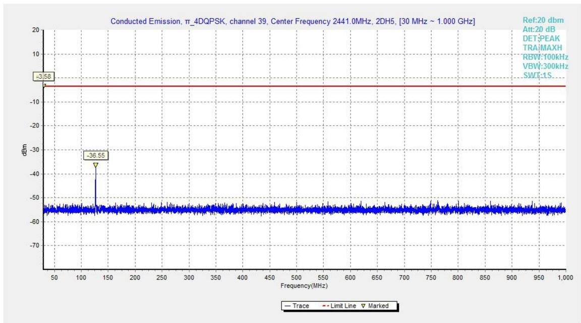
Fig.55. Conducted spurious emission:  $\pi/4$  DQPSK, Channel 39, 30MHz - 1GHz
