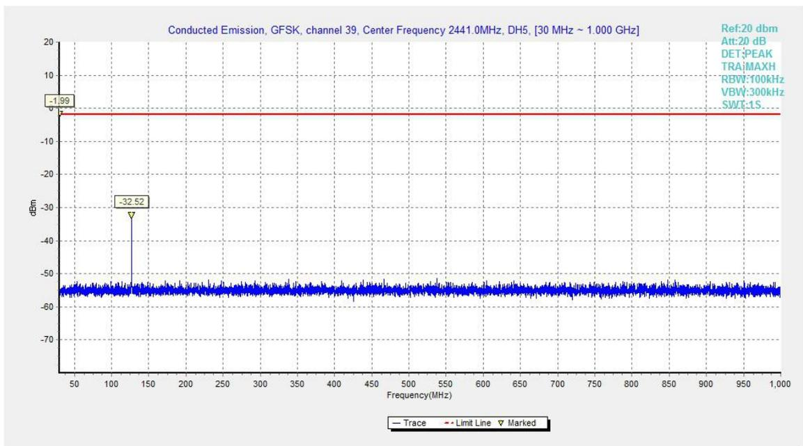
Fig.40. Conducted spurious emission: GFSK, Channel 39, 30MHz - 1GHz
