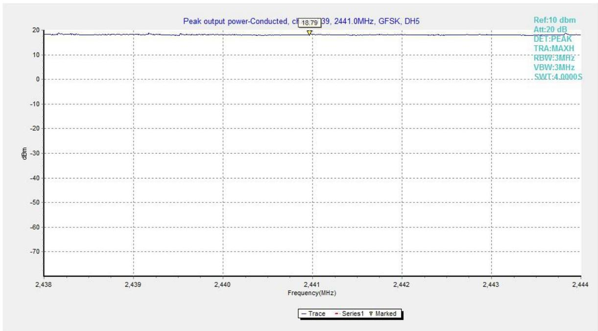
Fig.2. Peak Output Power -Conducted: Antenna 3, GFSK, Channel 39,
