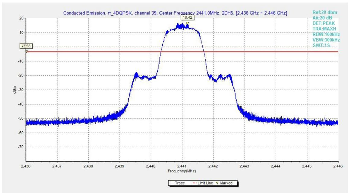
Fig.54. Conducted spurious emission:  $\pi/4$  DQPSK, Channel 39, 2441MHz
