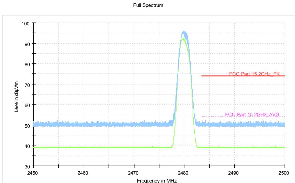
**Fig.27. Frequency Band Edges: EUT3 ANT3 8DPSK, Channel 78, 2.38 GHz - 2.45GHz**
