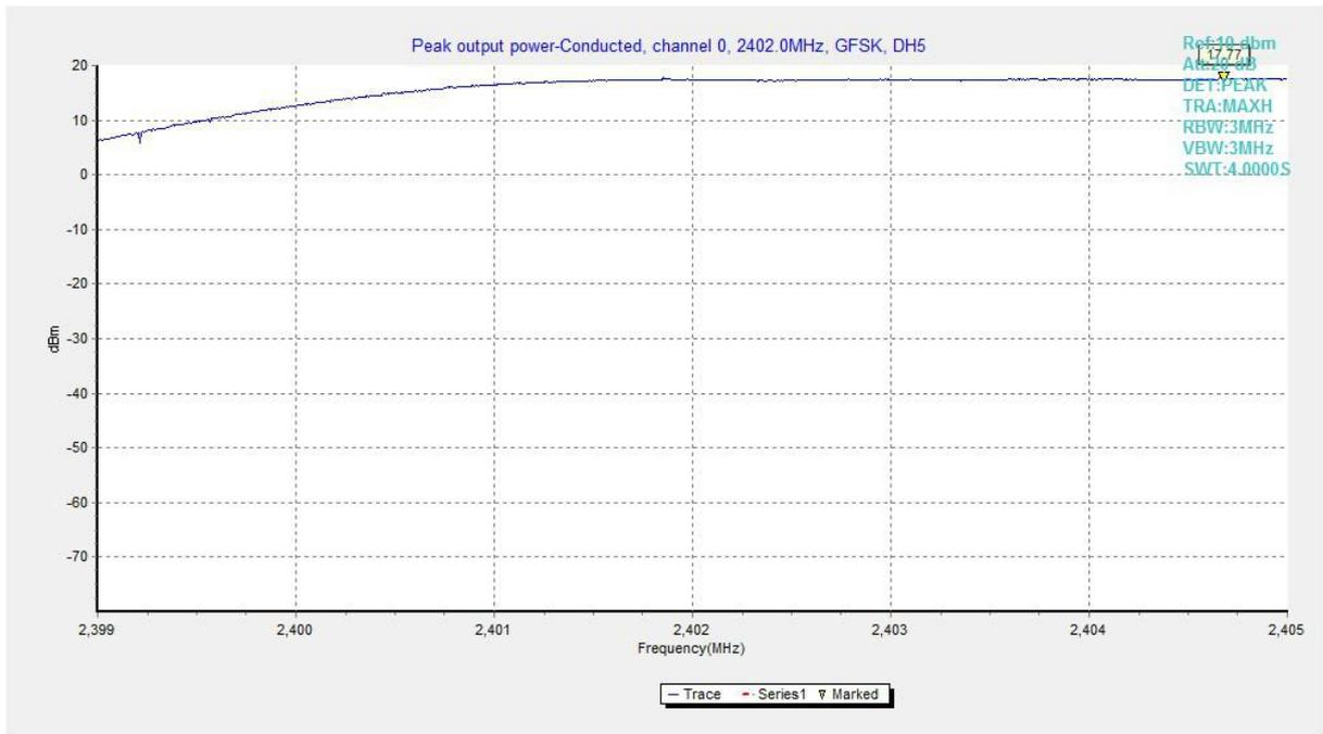
Fig.1. Peak Output Power -Conducted: Antenna 3, GFSK, Channel 0,
