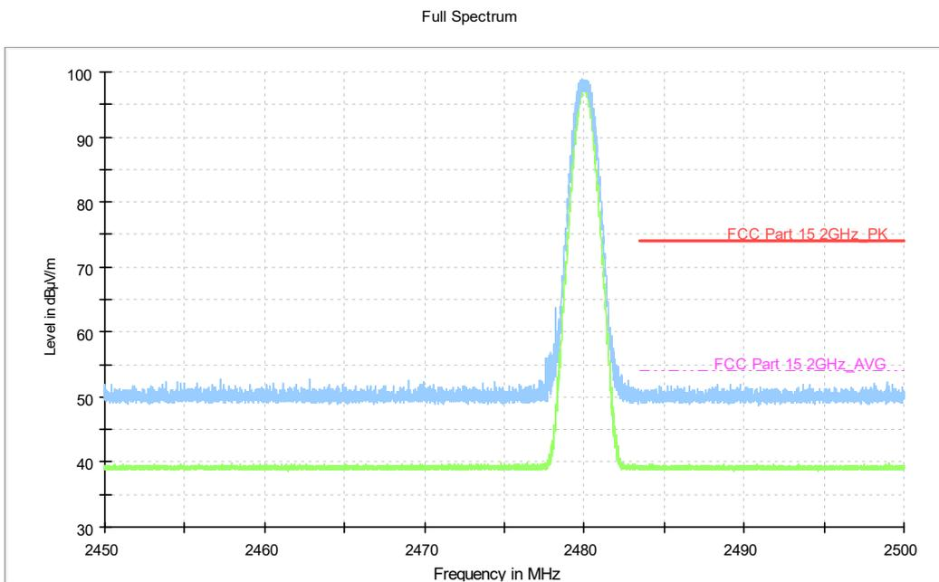
**Fig.29. Frequency Band Edges: EUT4 ANT4 GFSK, Channel 78, Hopping Off, ch11, 2.45 GHz - 2.50GHz**
