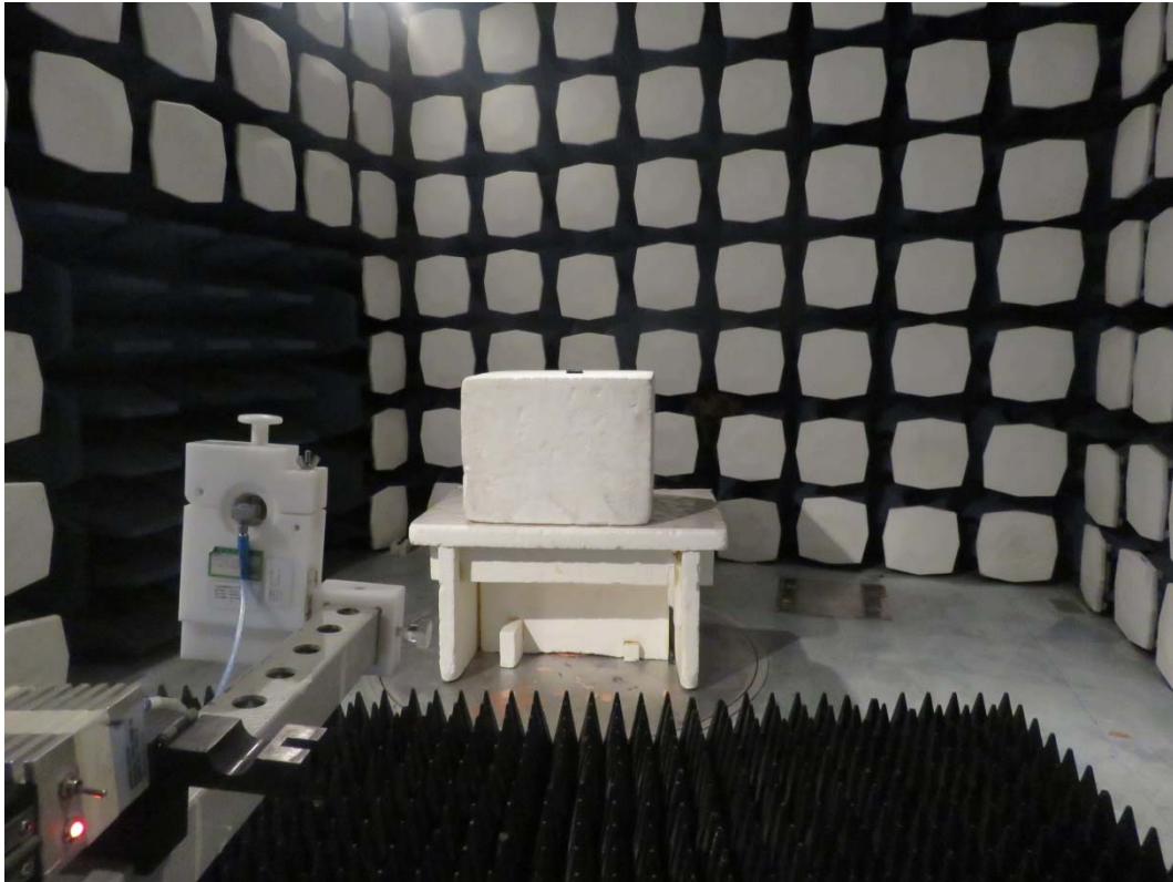
Picture 1 Radiated Emission Test Setup
