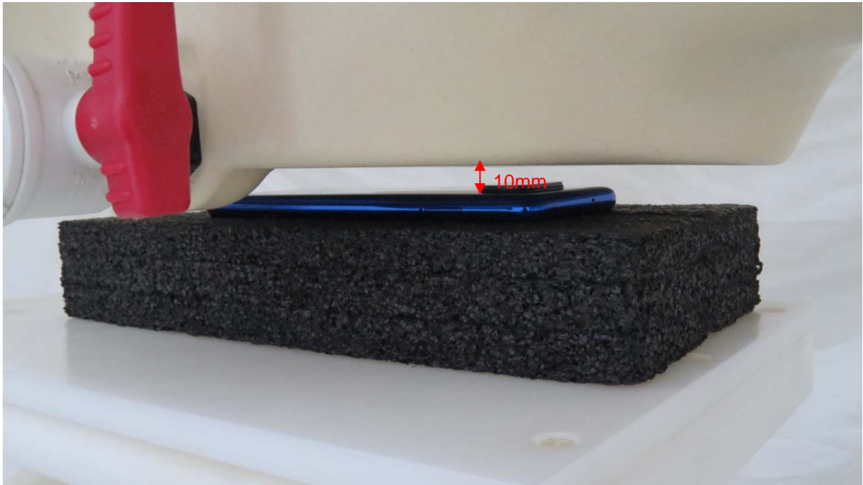
Picture 5: Back Side, the distance from handset to the bottom of the Phantom is 10mm
