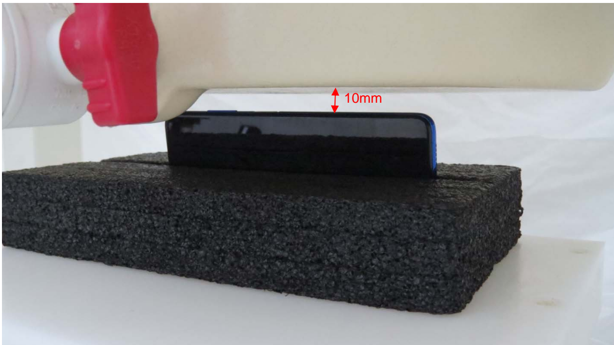
Picture 8: Right Side, the distance from handset to the bottom of the Phantom is 10mm
