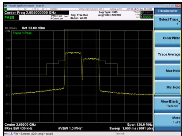
CA-38C 64QAM 15+15MHz CH- High, 100%RB
