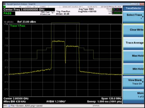
CA-38C 64QAM 15+15MHz CH- High, RB 1
