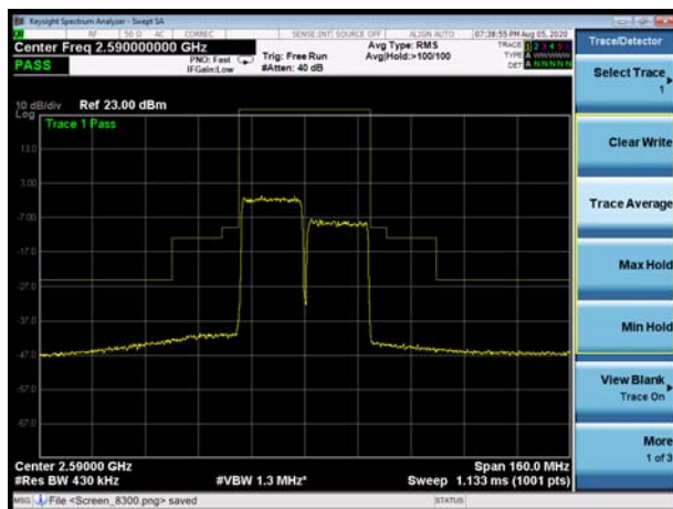
CA-38C 64QAM 20+20MHz CH-Low, 100%RB
