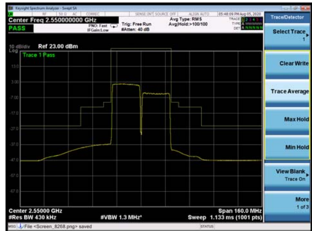
CA-7C 64QAM 20+20MHz CH- High, RB 1
