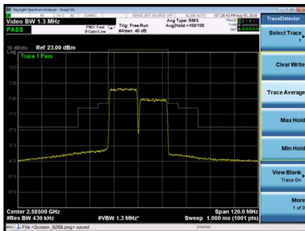
CA-38C 64QAM 15+15MHz CH-Low, 100%RB
