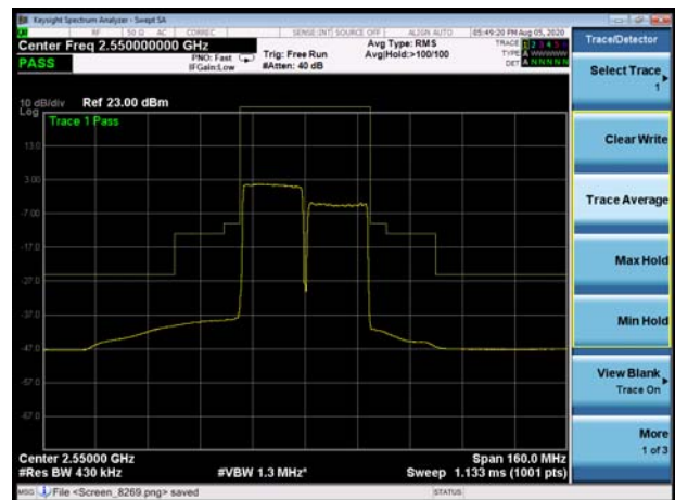
CA-7C 64QAM 20+20MHz CH- High, 100%RB
