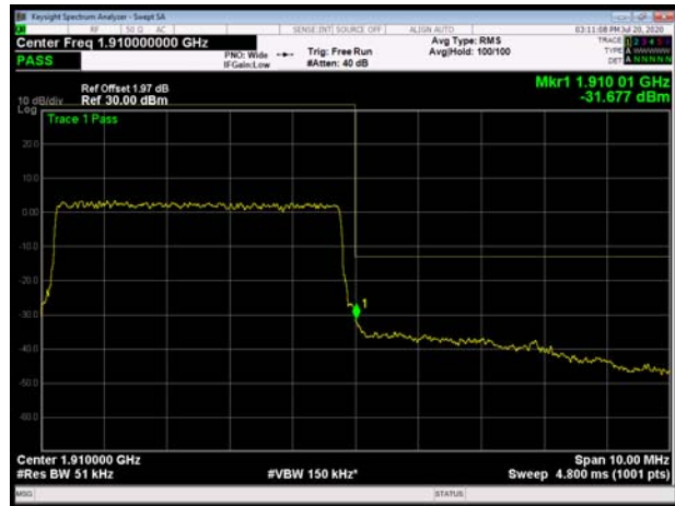
LTE Band 2 10MHz 64QAM 1RB CH-High
