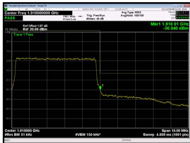
LTE Band 2 10MHz 16QAM 1RB CH-High
