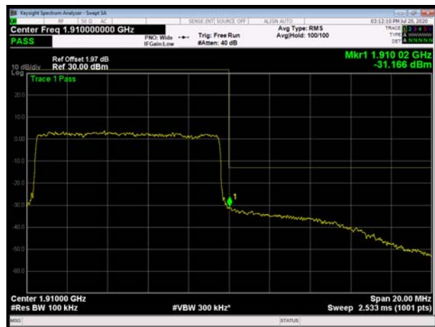
LTE Band 2 10MHz 64QAM 100%RB CH-High
