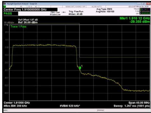
LTE Band 2 1.4MHz 16QAM 1RB CH-High
