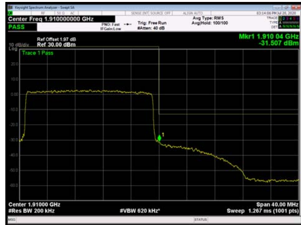
LTE Band 2 1.4MHz 64QAM 1RB CH-High
