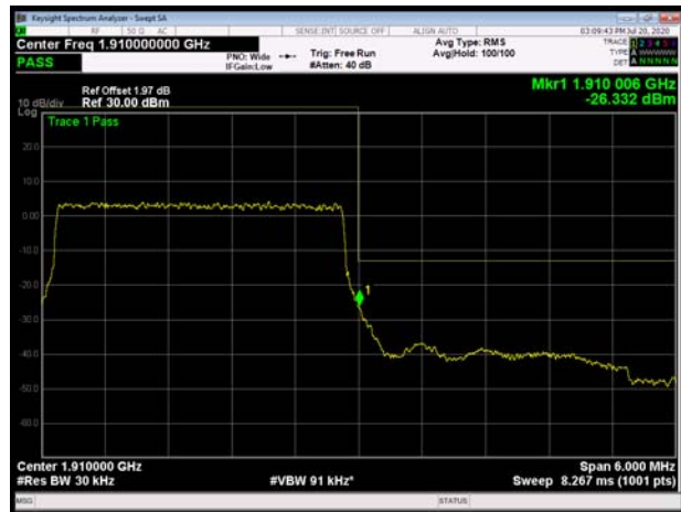
LTE Band 2 5MHz QPSK 1RB CH-High
