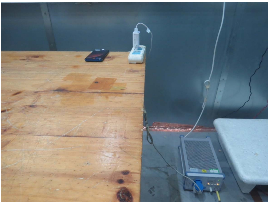
Picture 2 Conducted Emission Test Setup
