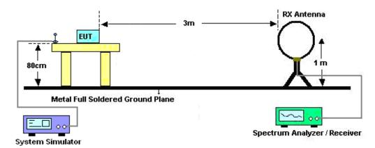
For radiated emissions from 30MHz to 1GHz
