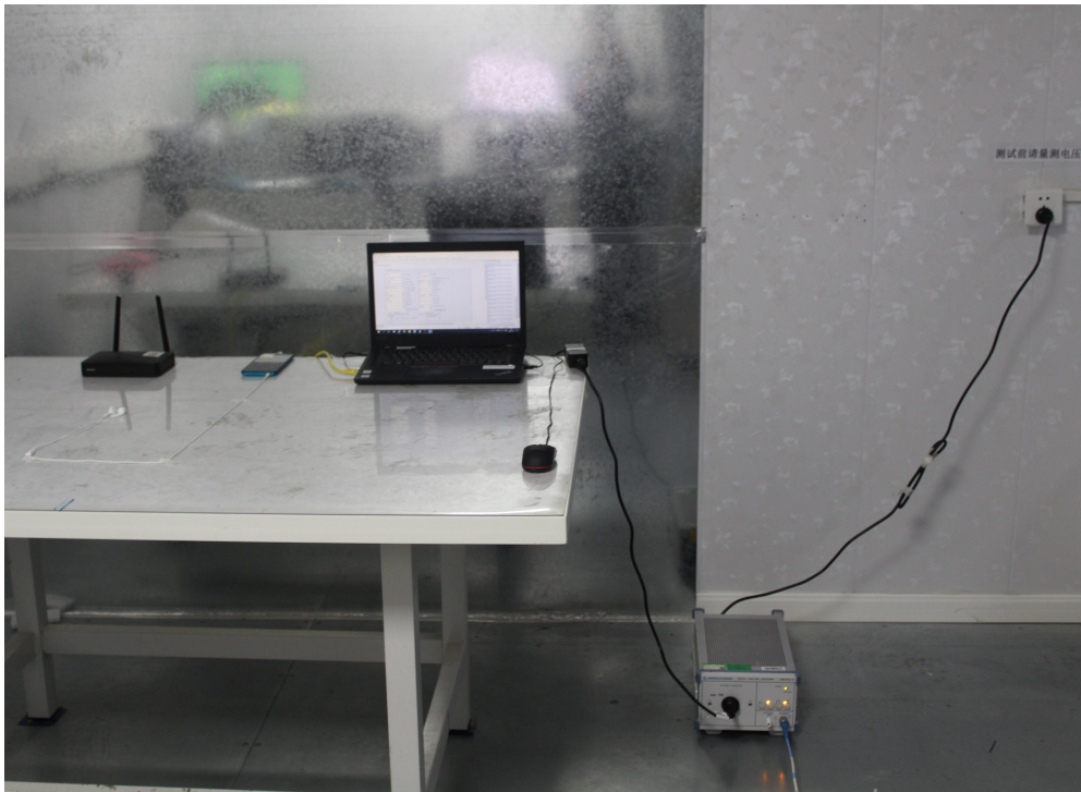
1.2 Setup for Unwanted Emissions that fall Outside of the Restricted Bands(Radiated) and Unwanted Emissions in the Restricted Bands (Radiated) below 1GHz ( Test Location: SGS-CSTC STANDARDS TECHNICAL SERVICES (XI 'AN) CO., LTD.)
