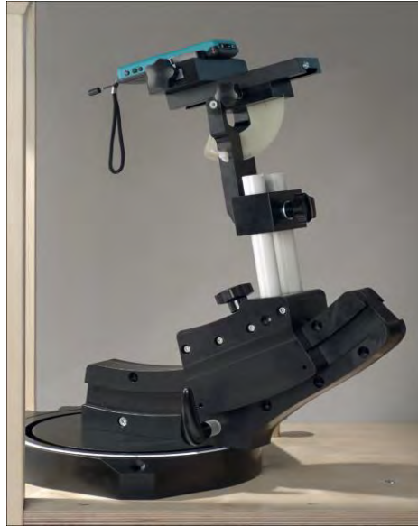
F-2. Device Holder for Transmitters
