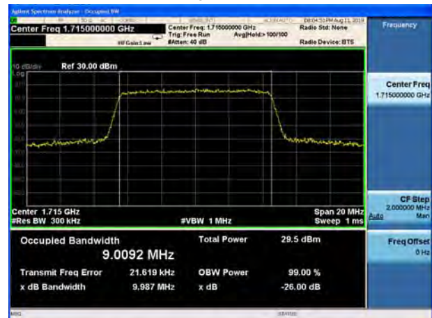
LTE Band 4 64QAM 10MHz CH-Middle
