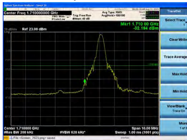
LTE Band 4 64QAM 20MHz CH-Low, 1 RB
