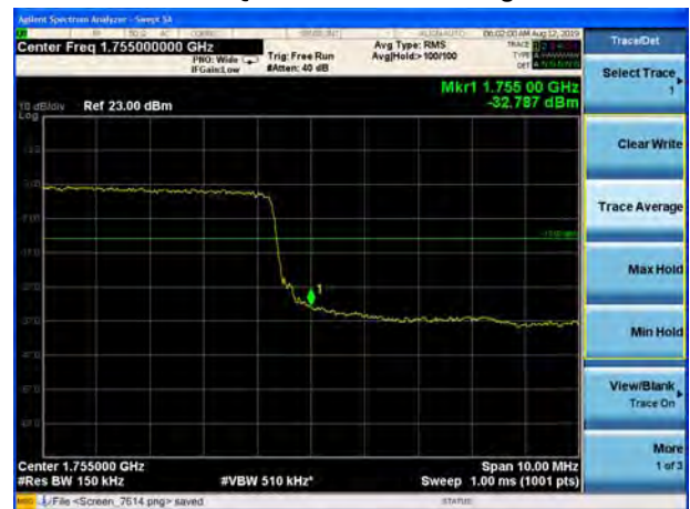
LTE Band 4 64QAM 20MHz CH-High, 1 RB
