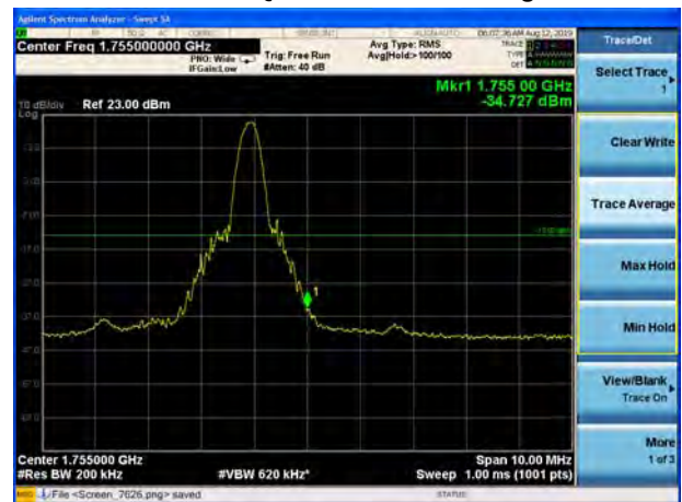
LTE Band 4 64QAM 20MHz CH-High, 1 RB
