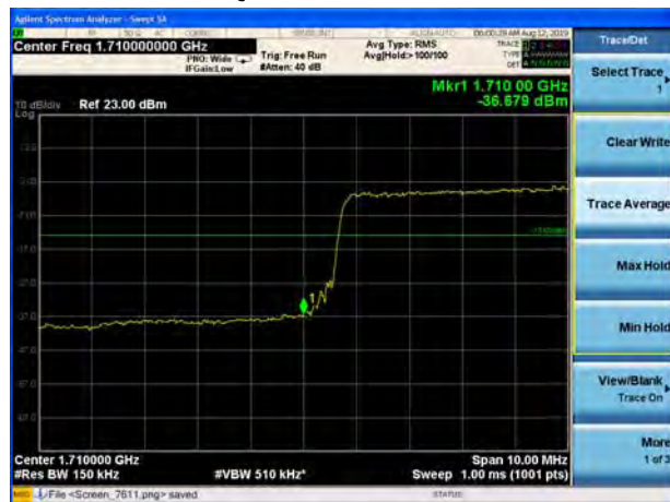
LTE Band 4 64QAM 20MHz CH-Low, 1 RB
