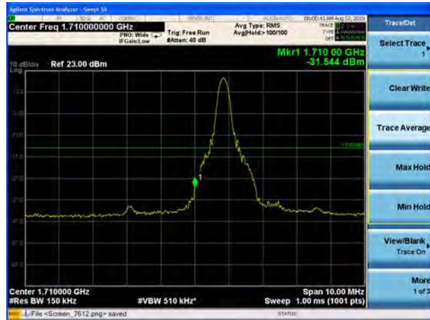
LTE Band 4 64QAM 15MHz CH-Low, 100%RB
