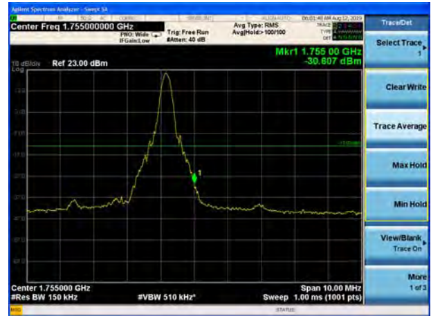
LTE Band 4 64QAM 15MHz CH-High, 100%RB
