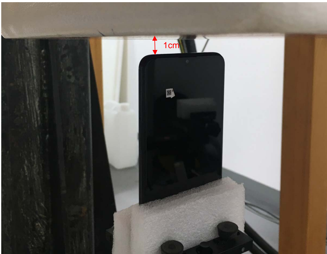
Picture 10: Top Side, the distance from handset to the bottom of the Phantom is 1.0cm
