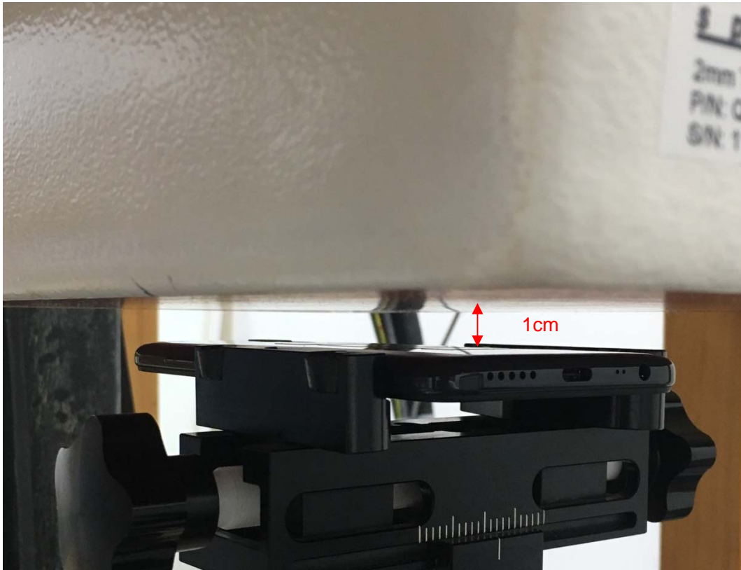
Picture 5: Back Side, the distance from handset to the bottom of the Phantom is 1.0cm
