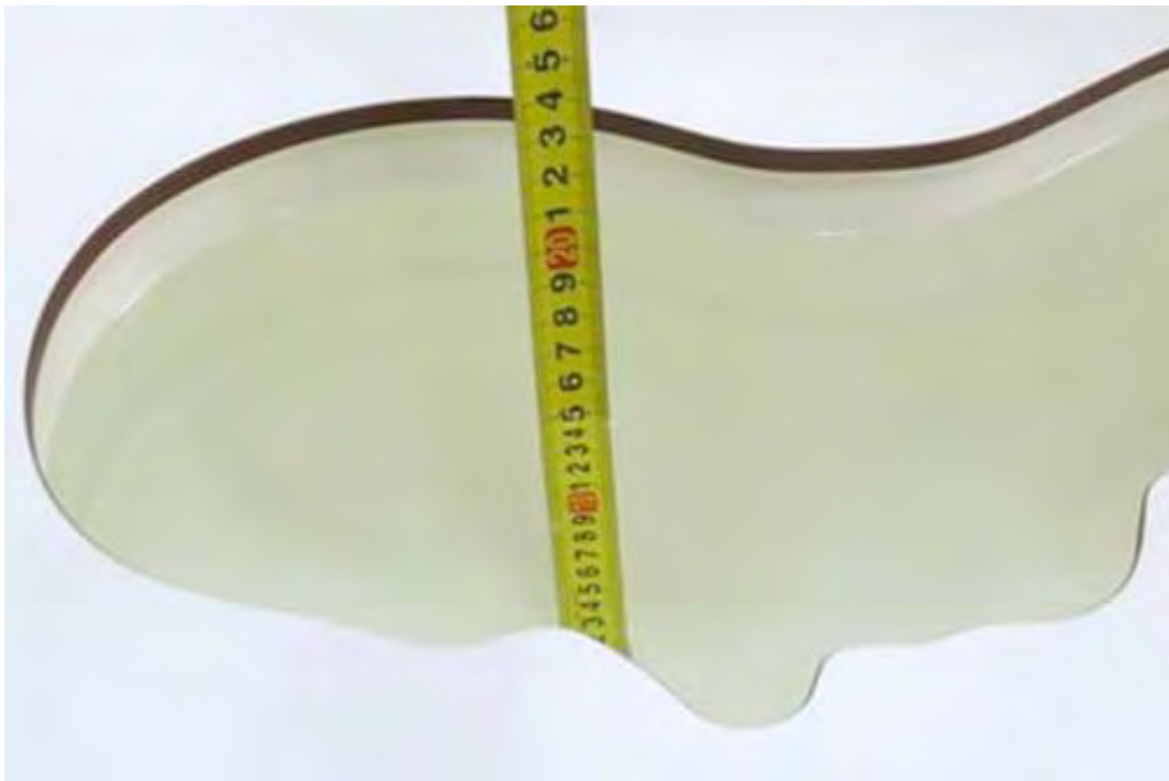
Picture 3: liquid depth in the head Phantom
