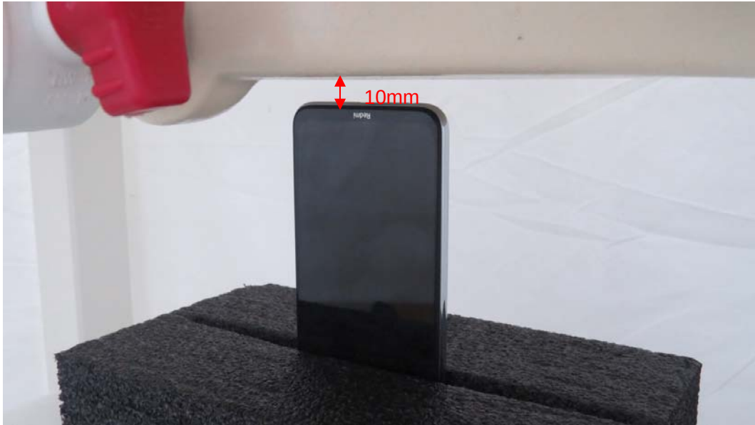
Picture 11: Bottom Side, the distance from handset to the bottom of the Phantom is 10mm
