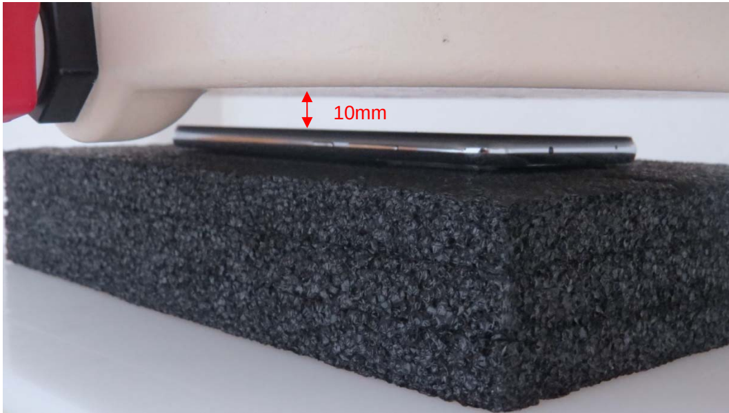
Picture 7: Front Side, the distance from handset to the bottom of the Phantom is 10mm
