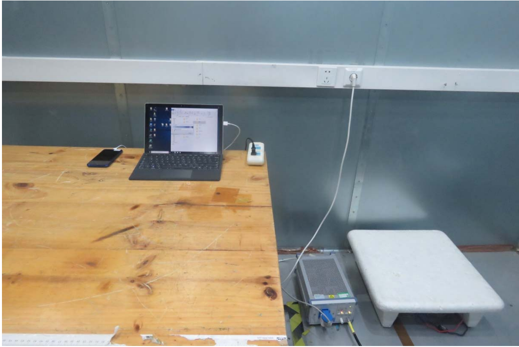
Picture 2 Conducted Emission Test Setup
