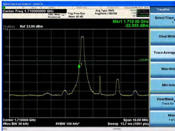
LTE Band 4 64QAM 3MHz CH-High, 1 RB
