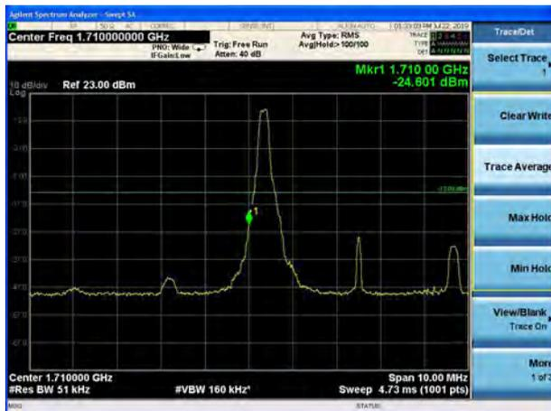
LTE Band 4 64QAM 5MHz CH-High, 1 RB
