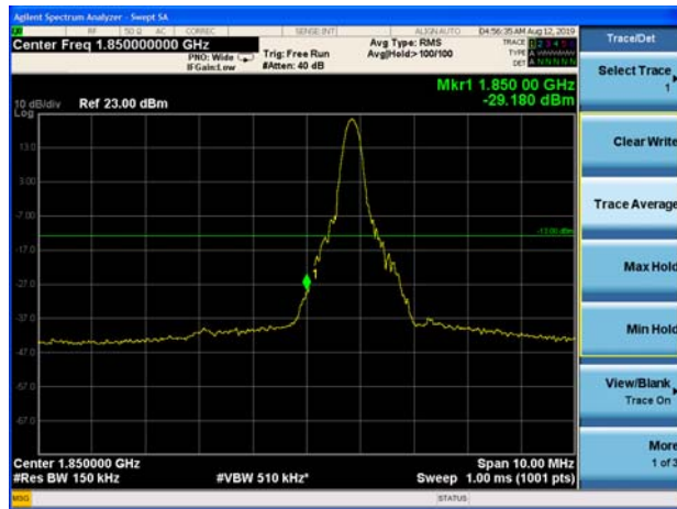
LTE Band 2 15MHz QPSK 100%RB CH-Low
