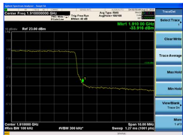
LTE Band 2 10MHz 16QAM 100%RB CH-High
