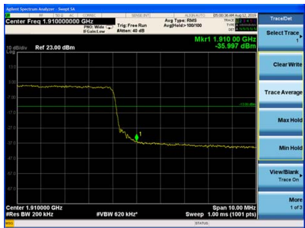
LTE Band 2 20MHz 64QAM 100%RB CH-High
