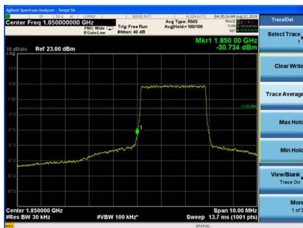
LTE Band 2 5MHz 64QAM 1RB CH-Low
