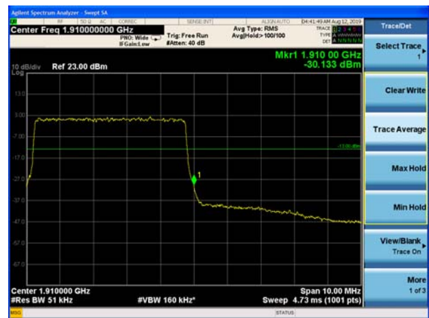
LTE Band 2 10MHz 16QAM 1RB CH-High
