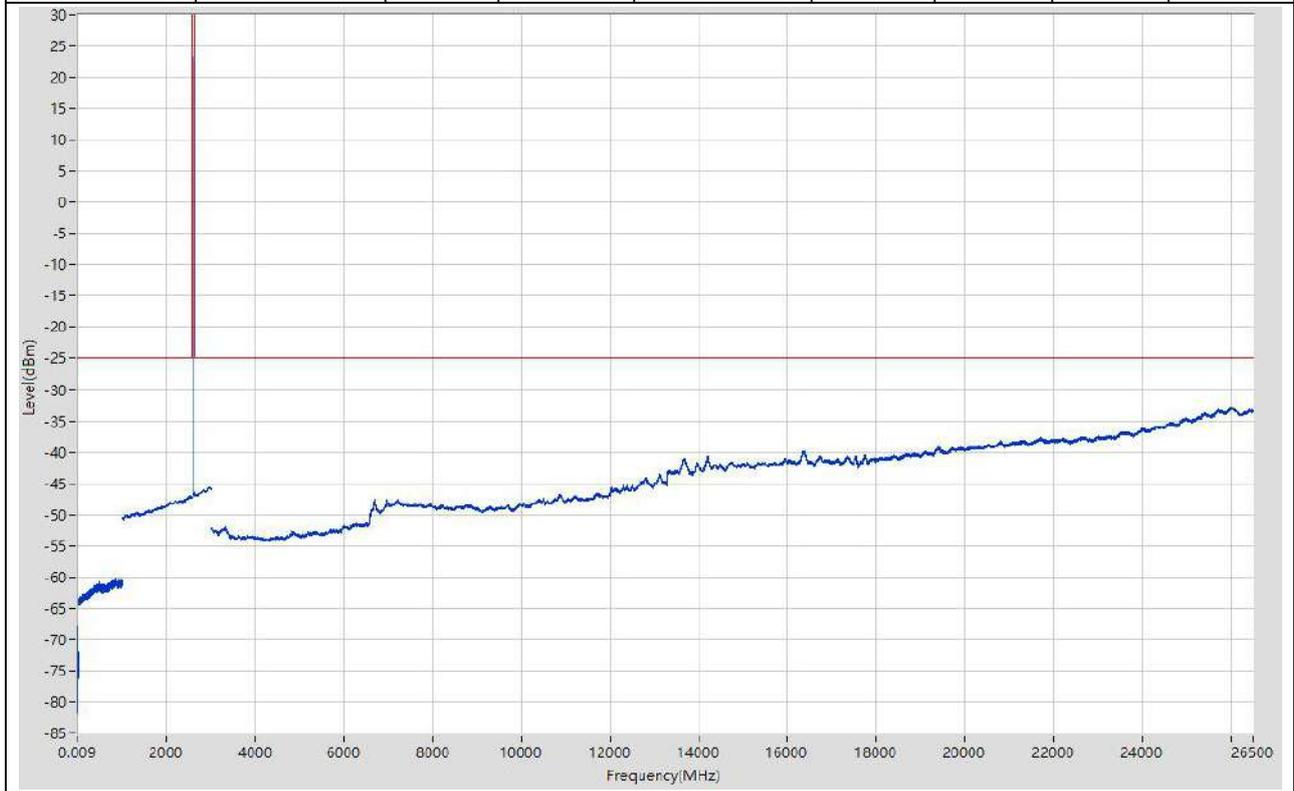
**17.6. LTE Spurious Emission at Antenna Terminals\_Part22-24-27(NTNV)(Subtest:6, Channel:38225, Bandwidth:5, Modulation:Q16, RB Number: 1, RB Position:LOW)**
