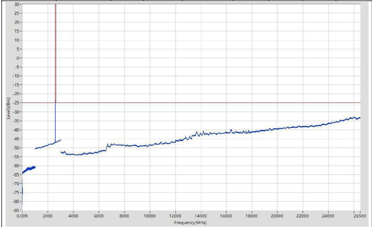
**17.3. LTE Spurious Emission at Antenna Terminals\_Part22-24-27(NTNV)(Subtest:3, Channel:38000, Bandwidth:5, Modulation:QPSK, RB Number: 1, RB Position:LOW)**
