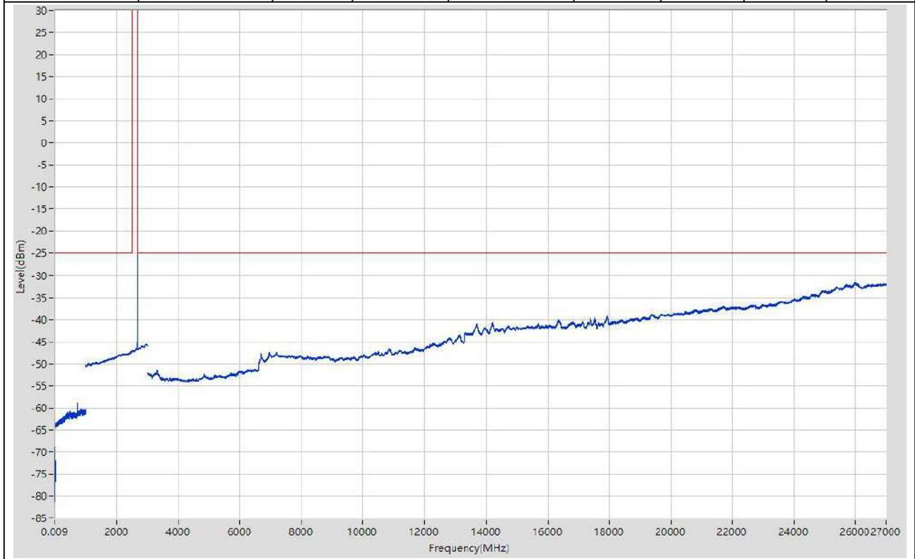
**18.6. LTE Spurious Emission at Antenna Terminals\_Part22-24-27(NTNV)(Subtest:6, Channel:41565, Bandwidth:5, Modulation:Q16, RB Number: 1, RB Position:LOW)**
