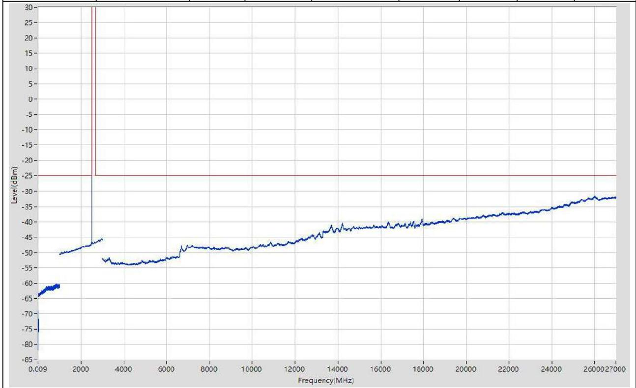
**18.3. LTE Spurious Emission at Antenna Terminals\_Part22-24-27(NTNV)(Subtest:3, Channel:40620, Bandwidth:5, Modulation:QPSK, RB Number: 1, RB Position:LOW)**
