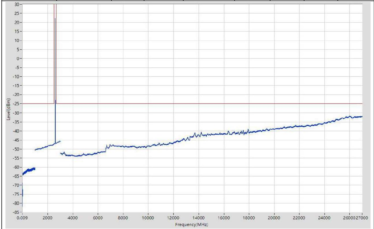
**18.5. LTE Spurious Emission at Antenna Terminals\_Part22-24-27(NTNV)(Subtest:5, Channel:41565, Bandwidth:5, Modulation:QPSK, RB Number: 1, RB Position:LOW)**
