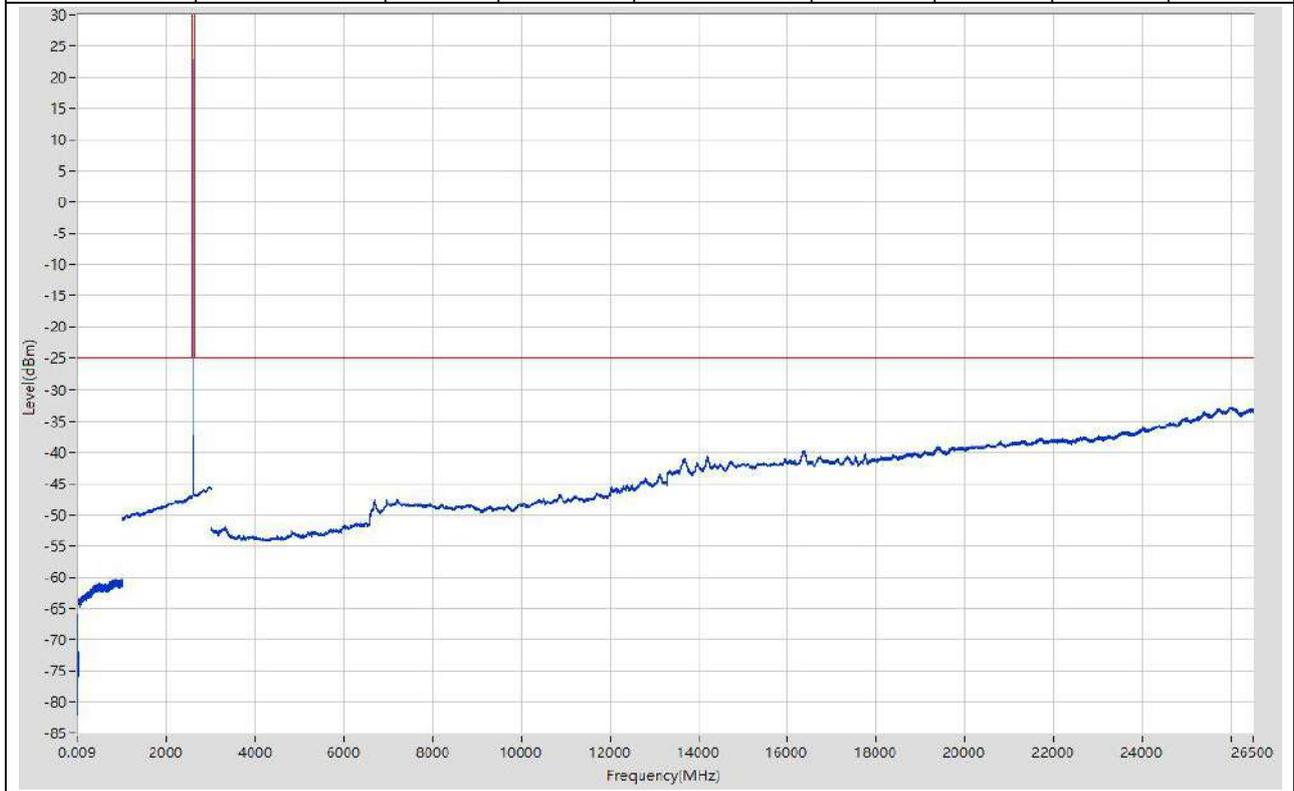
**17.5. LTE Spurious Emission at Antenna Terminals\_Part22-24-27(NTNV)(Subtest:5, Channel:38225, Bandwidth:5, Modulation:QPSK, RB Number: 1, RB Position:LOW)**
