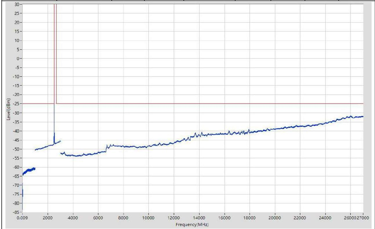
**18.9. LTE Spurious Emission at Antenna Terminals\_Part22-24-27(NTNV)(Subtest:9, Channel:40620, Bandwidth:10, Modulation:QPSK, RB Number: 1, RB Position:LOW)**
