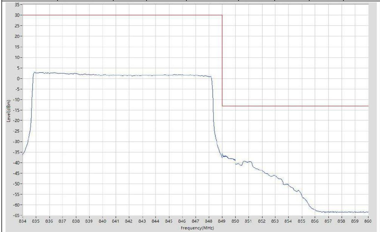
**15.39. LTE Band Edge\_Part22-24-27(NTNV)(Subtest:39, Channel:26965, Bandwidth:15, Modulation:Q16, RB Number: 1, RB Position:HIGH)**
