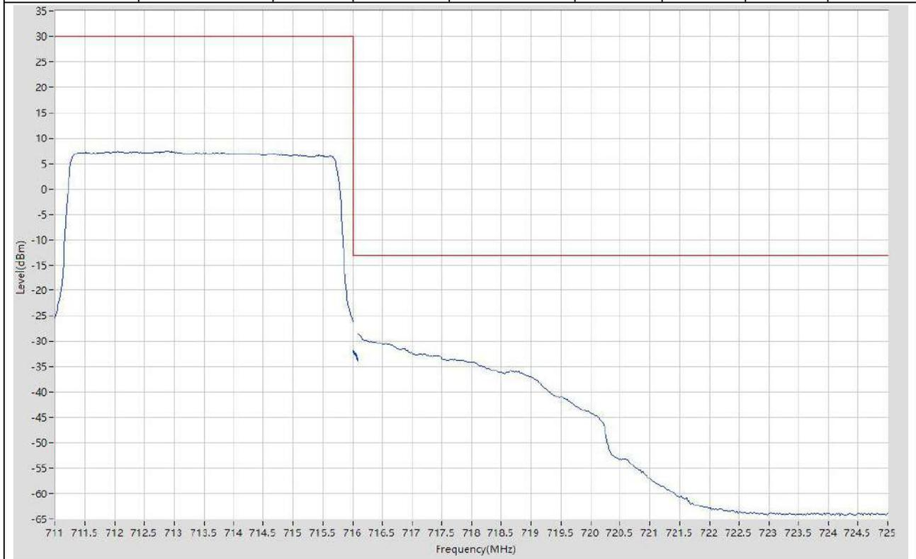
**12.23. LTE Band Edge\_Part22-24-27(NTNV)(Subtest:23, Channel:23155, Bandwidth:5, Modulation:Q16, RB Number: 1, RB Position:HIGH)**
