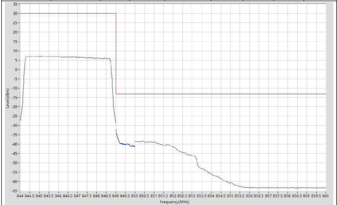
**15.23. LTE Band Edge\_Part22-24-27(NTNV)(Subtest:23, Channel:27015, Bandwidth:5, Modulation:Q16, RB Number: 1, RB Position:HIGH)**
