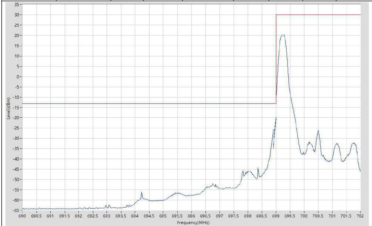
**12.12. LTE Band Edge\_Part22-24-27(NTNV)(Subtest:12, Channel:23025, Bandwidth:3, Modulation:Q16, RB Number: 15, RB Position:LOW)**
