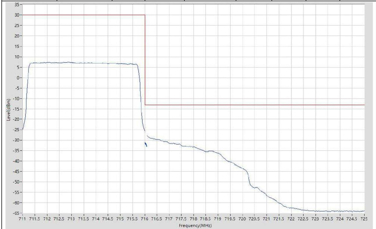
**14.7. LTE Band Edge\_Part22-24-27(NTNV)(Subtest:7, Channel:23825, Bandwidth:5, Modulation:Q16, RB Number: 1, RB Position:HIGH)**
