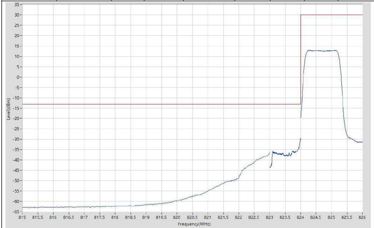
**15.3. LTE Band Edge\_Part22-24-27(NTNV)(Subtest:3, Channel:26797, Bandwidth:1.4, Modulation:Q16, RB Number: 1, RB Position:LOW)**
