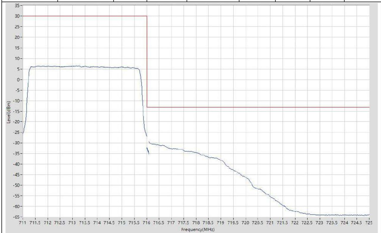
**14.9. LTE Band Edge\_Part22-24-27(NTNV)(Subtest:9, Channel:23780, Bandwidth:10, Modulation:QPSK, RB Number: 1, RB Position:LOW)**
