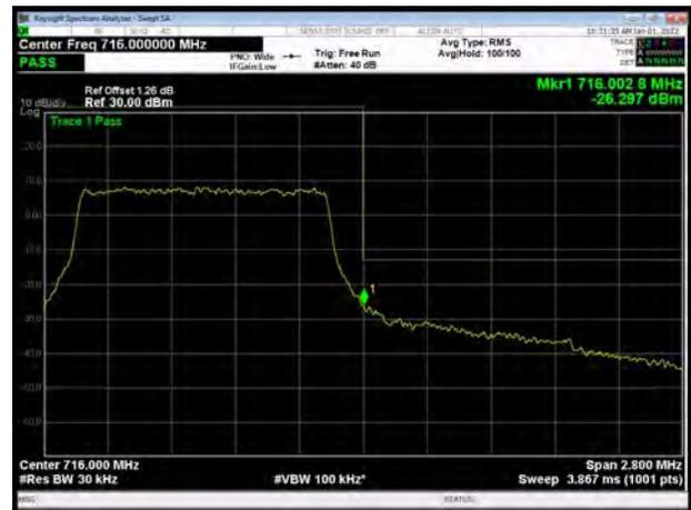
LTE Band 12 16QAM 3MHz CH-Low, 1 RB
