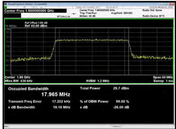
LTE Band 2 15MHz 16QAM CH-Middle
