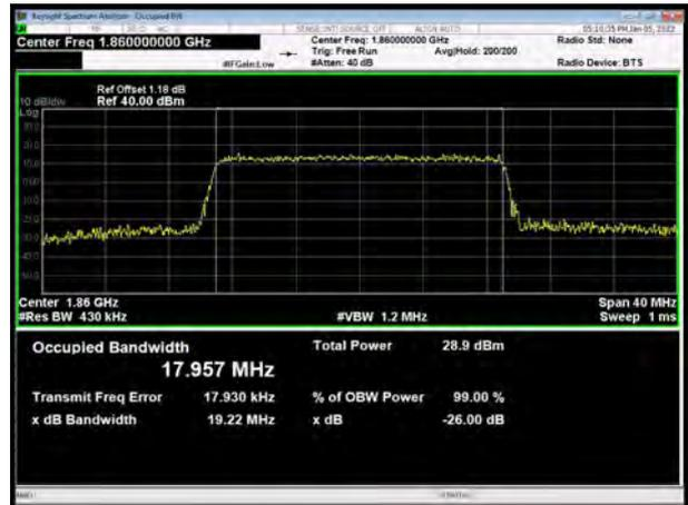
LTE Band 2 15MHz 64QAM CH-Middle
