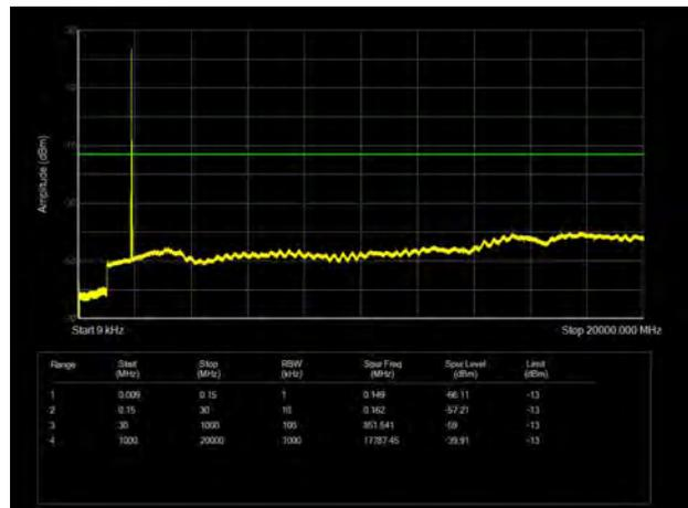
LTE Band 2 15MHz CH-High 9kHz~20GHz
