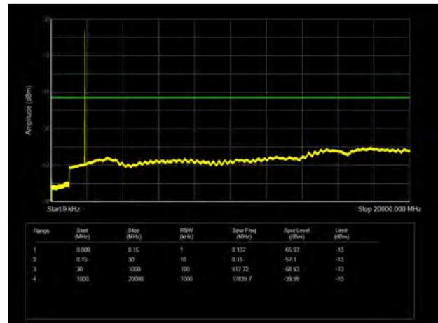
LTE Band 2 5MHz CH-High 9kHz~20GHz
