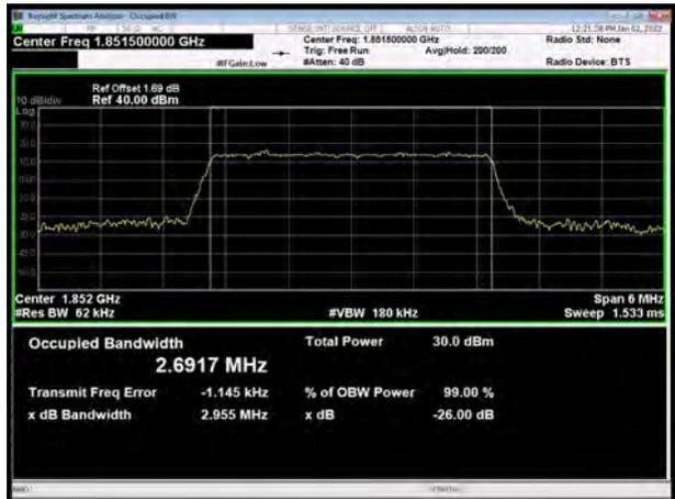
LTE Band 2 1.4MHz 16QAM CH-Middle
