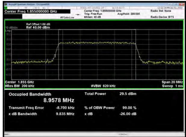
LTE Band 2 5MHz 16QAM CH-Middle
