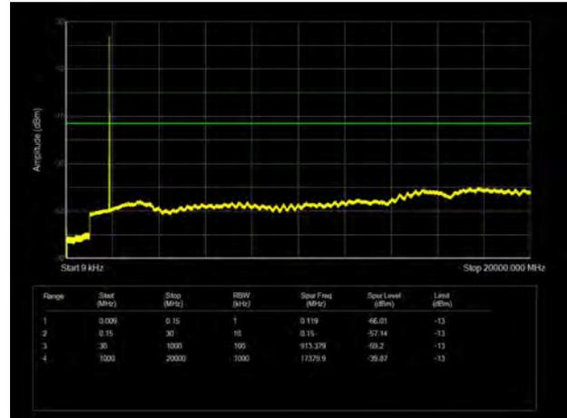
LTE Band 2 5MHz CH-Middle 9kHz~20GHz
