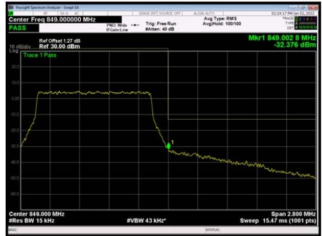
LTE Band 5 16QAM 3MHz CH-Low 1RB
