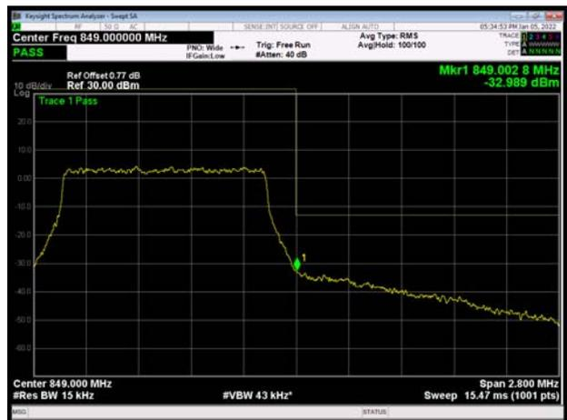
LTE Band 5 64QAM 3MHz CH-Low 1RB
