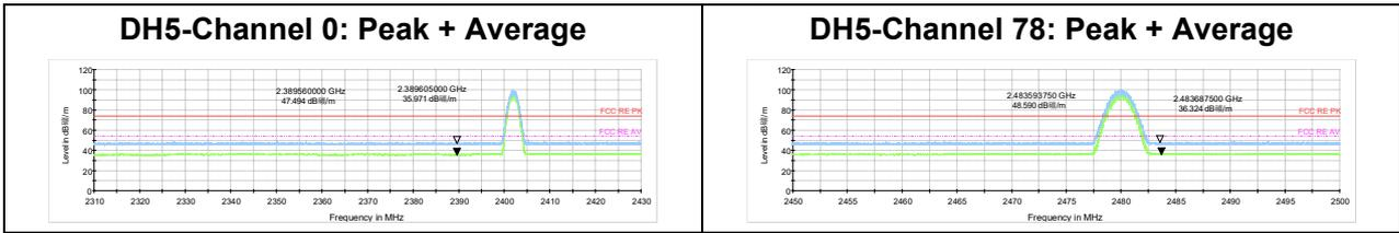
The bandage was performed in all EDR modes (2DH5 and 3DH5), 3DH5 was selected as the worse condition. The test data of the worst-case condition was recorded in this report.
