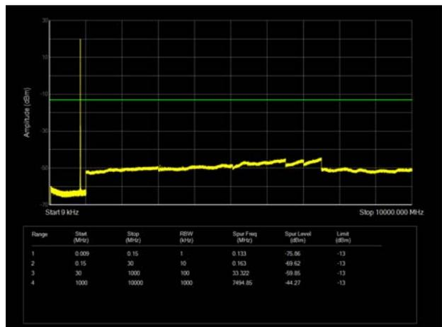
LTE Band 5 5MHz CH-Low 9kHz~10GHz
