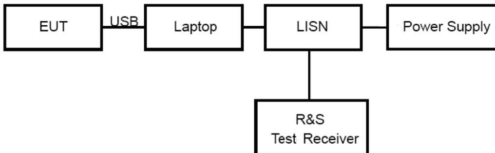
Note: Power Supply is AC Power source and it is used to change the voltage 120V/60Hz.
