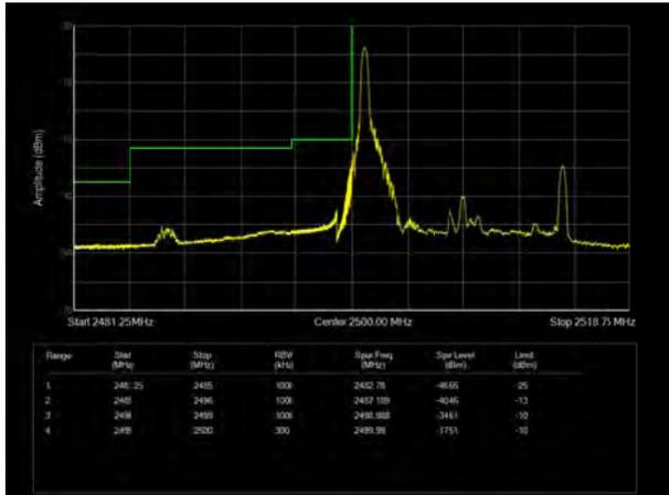
LTE Band 7 16QAM 15MHz CH-High, 1 RB
