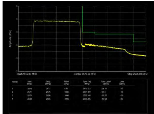
LTE Band 7 16QAM 5MHz CH-Low, 1 RB
