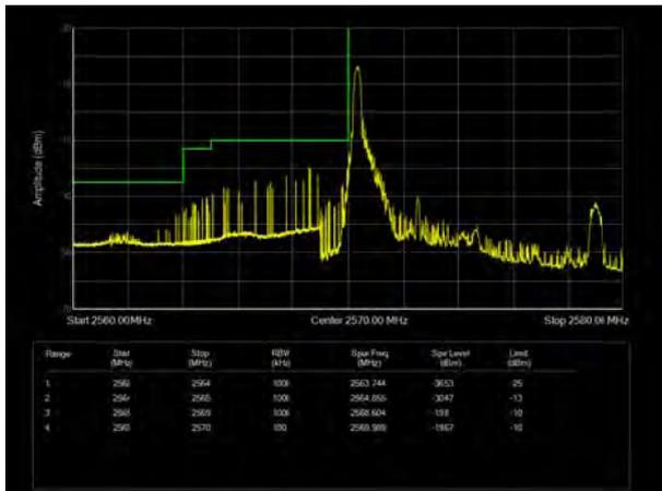
LTE Band 38 16QAM 5MHz CH-High, 1 RB
