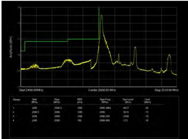
LTE Band 7 16QAM 5MHz CH-High, 1 RB
