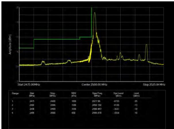
LTE Band 7 16QAM 20MHz CH-High, 1 RB
