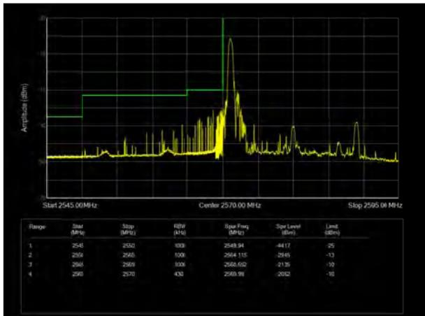
LTE Band 38 16QAM 20MHz CH-High, 1 RB
