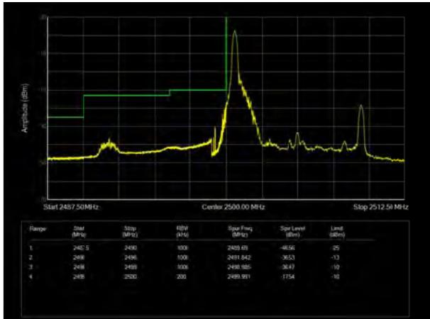
LTE Band 7 16QAM 10MHz CH-High, 1 RB
