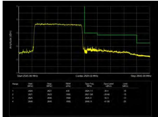
LTE Band 38 16QAM 5MHz CH-Low, 1 RB
