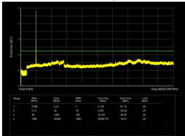
LTE Band 41 5MHz CH-Low 9kHz~30GHz
