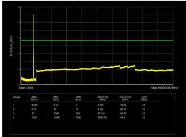
LTE Band 5 5MHz CH-Middle 9kHz~10GHz
