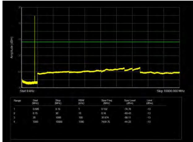
LTE Band 5 1.4MHz CH-Middle 9kHz~10GHz
