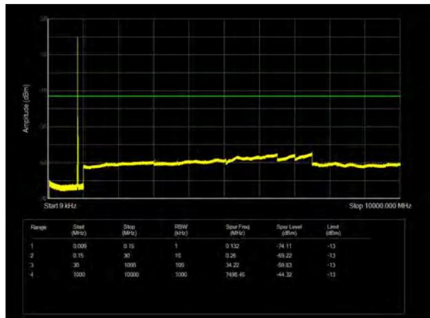
LTE Band 5 5MHz CH-High 9kHz~10GHz
