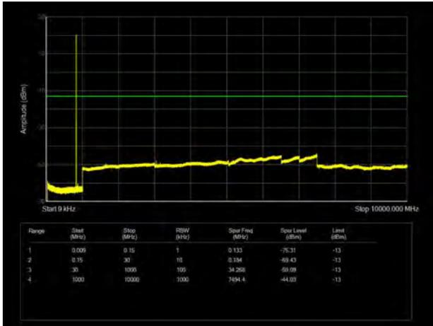
LTE Band 5 3MHz CH-Low 9kHz~10GHz
