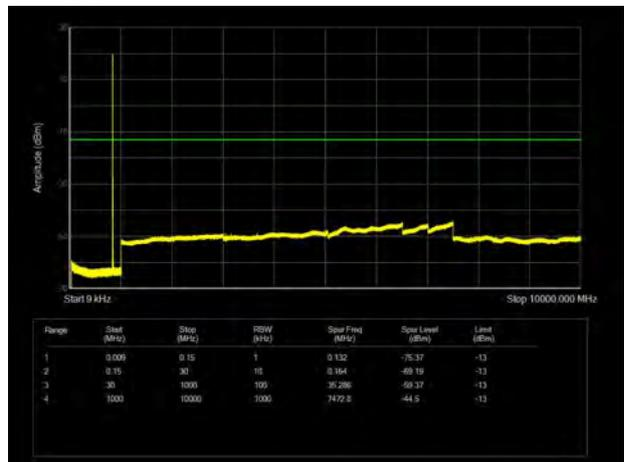
LTE Band 5 1.4MHz CH-High 9kHz~10GHz
