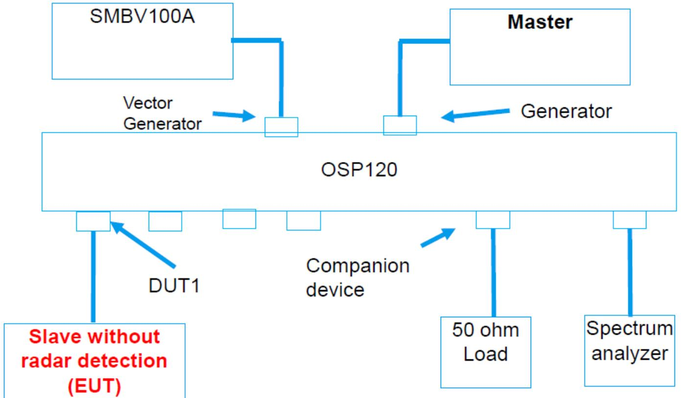
The UUT is a U-NII Device operating in Client mode without radar detection. The radar test signals are injected into the Master Device.
