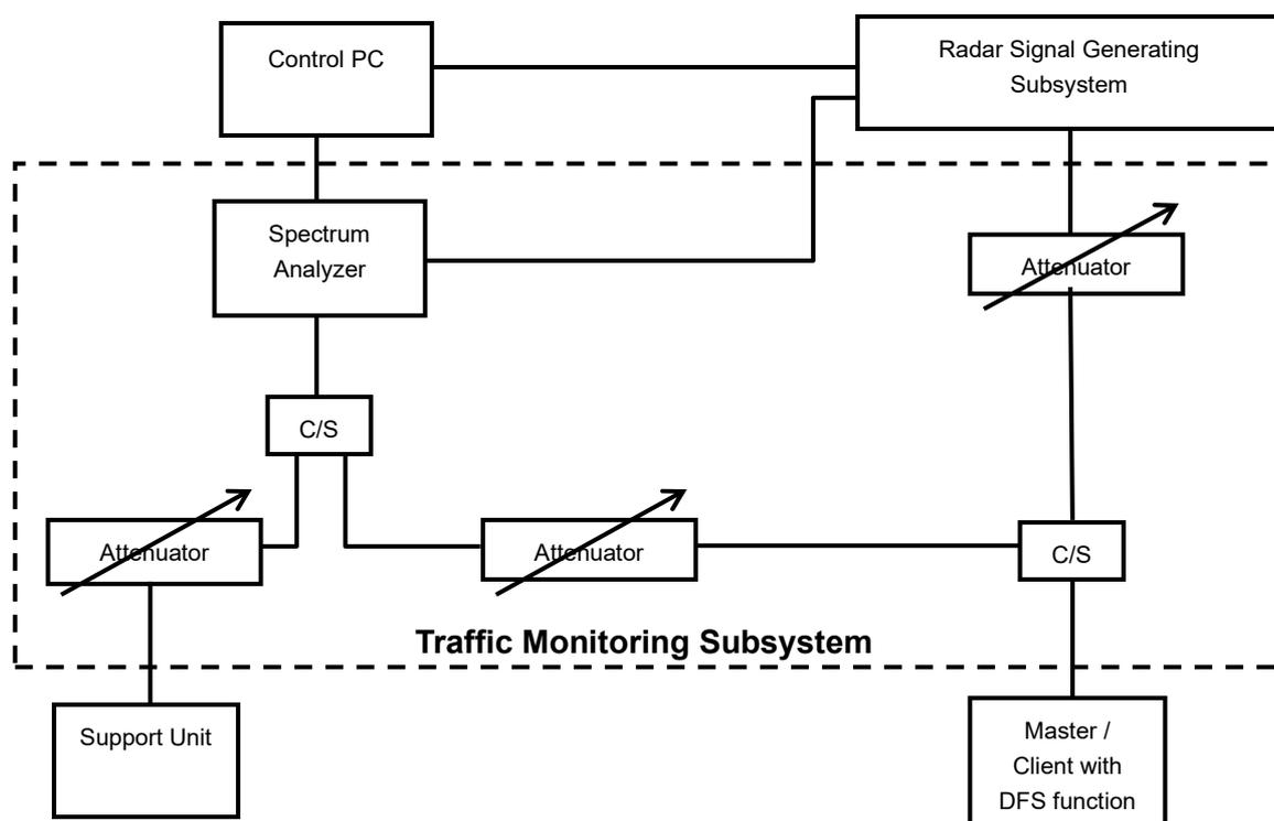
The test transmission will always be from the Master Device to the Client Device. While the Client device is set up to associate with the Master device and play the MPEG file (6 ψ Magic Hours) from Master device, the designated MPEG test file and instructions are located at: <http://ntiacsd.ntia.doc.gov/dfs/>.
