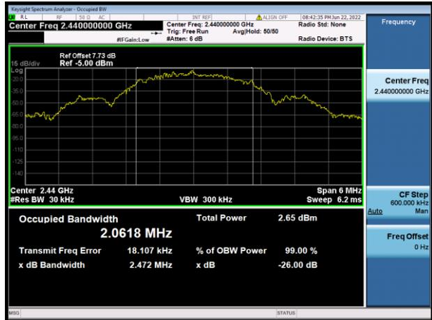
GFSK (BLE 2Mbps) HIGH CHANNEL
