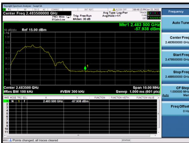
GFSK (BLE 2Mbps) HIGH CHANNEL, BAND EDGE
