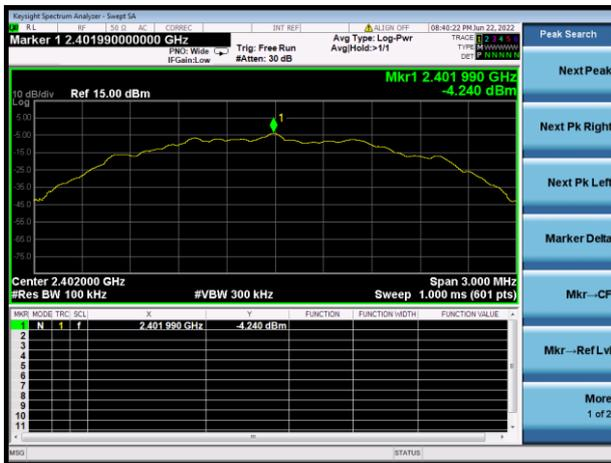
GFSK (BLE 2Mbps) LOW CHANNEL, REFERENCE LEVEL
