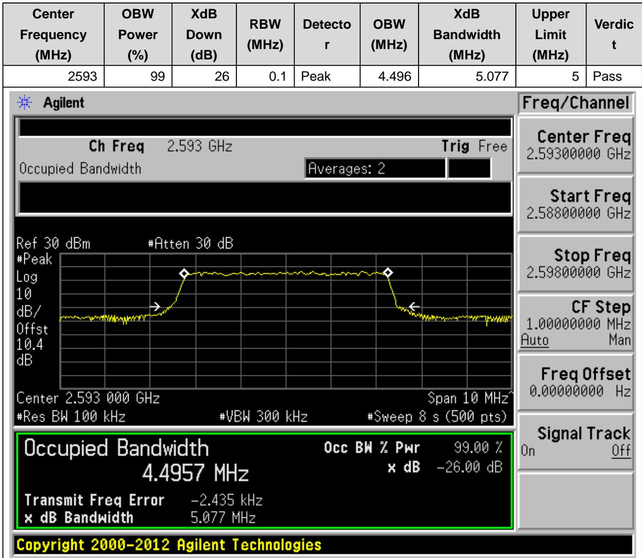
**13.5. LTE Occupied Bandwidth(NTNV)(Subtest:5, Channel:41565, Bandwidth:5, Modulation:QPSK, RB Number: 25, RB Position:LOW)**
