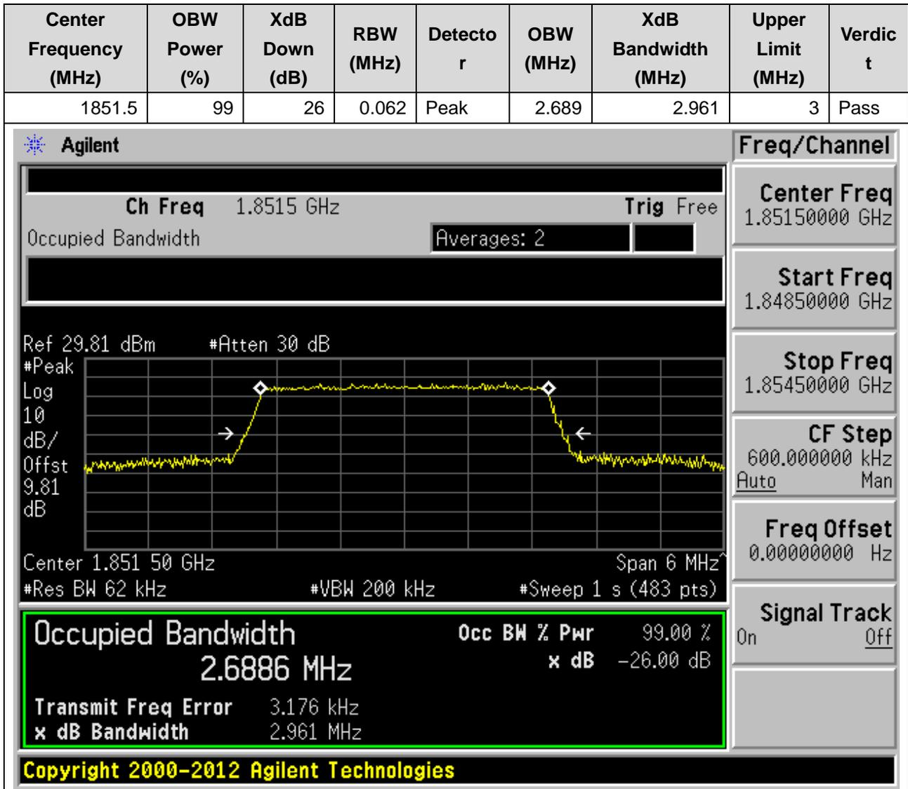
**8.9. LTE Occupied Bandwidth(NTNV)(Subtest:9, Channel:18900, Bandwidth:3, Modulation:QPSK, RB Number: 15, RB Position:LOW)**
