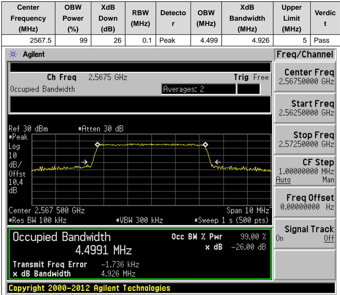
**11.7. LTE Occupied Bandwidth(NTNV)(Subtest:7, Channel:20800, Bandwidth:10, Modulation:QPSK, RB Number: 50, RB Position:LOW)**
