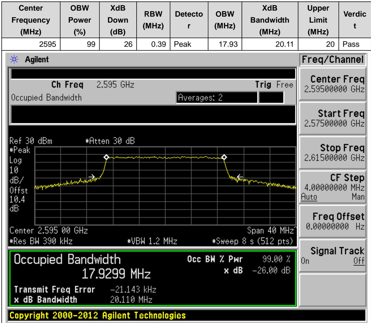
**12.23. LTE Occupied Bandwidth(NTNV)(Subtest:23, Channel:38150, Bandwidth:20, Modulation:QPSK, RB Number: 100, RB Position:LOW)**
