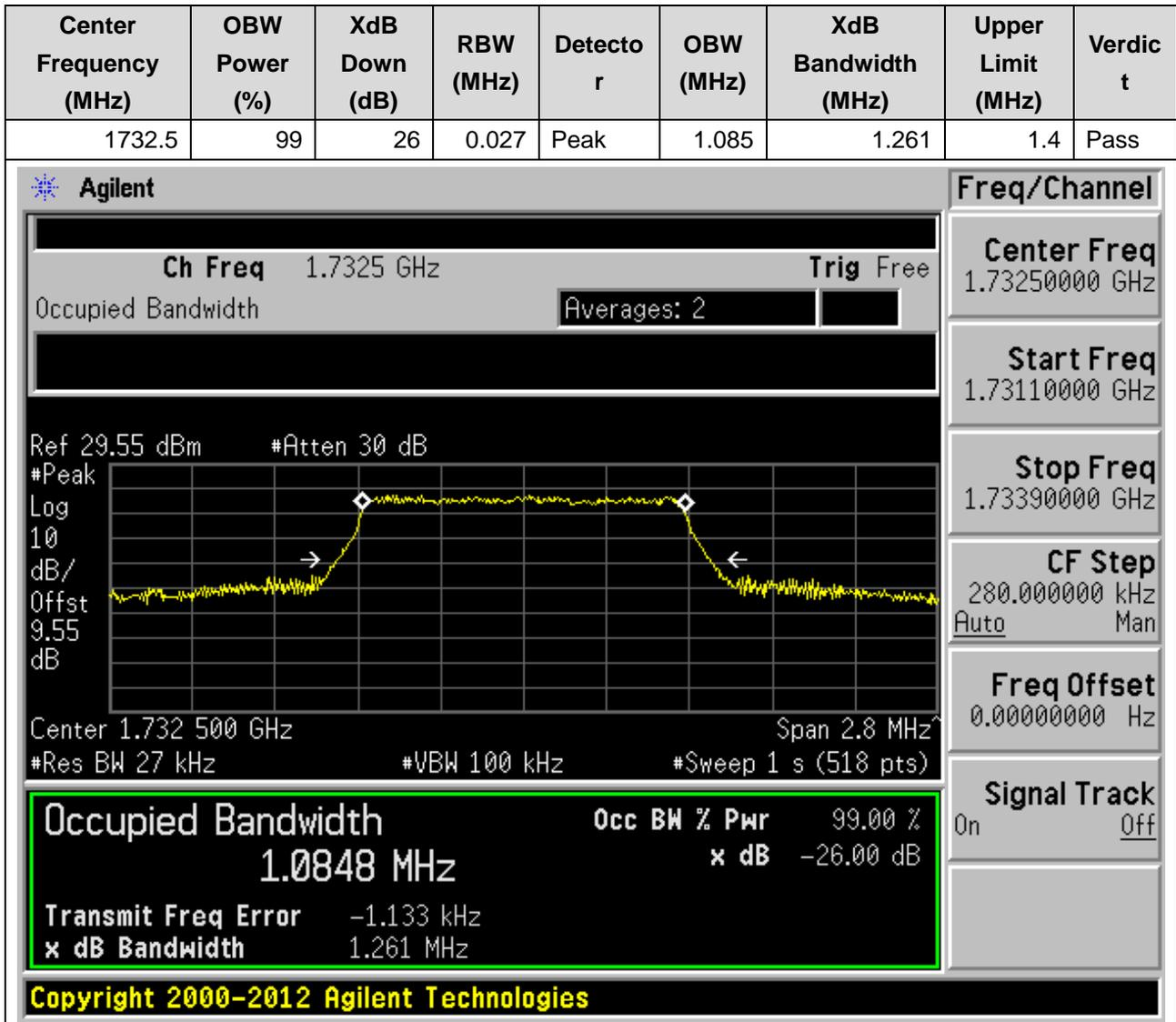
**9.5. LTE Occupied Bandwidth(NTNV)(Subtest:5, Channel:20393, Bandwidth:1.4, Modulation:QPSK, RB Number: 6, RB Position:LOW)**
