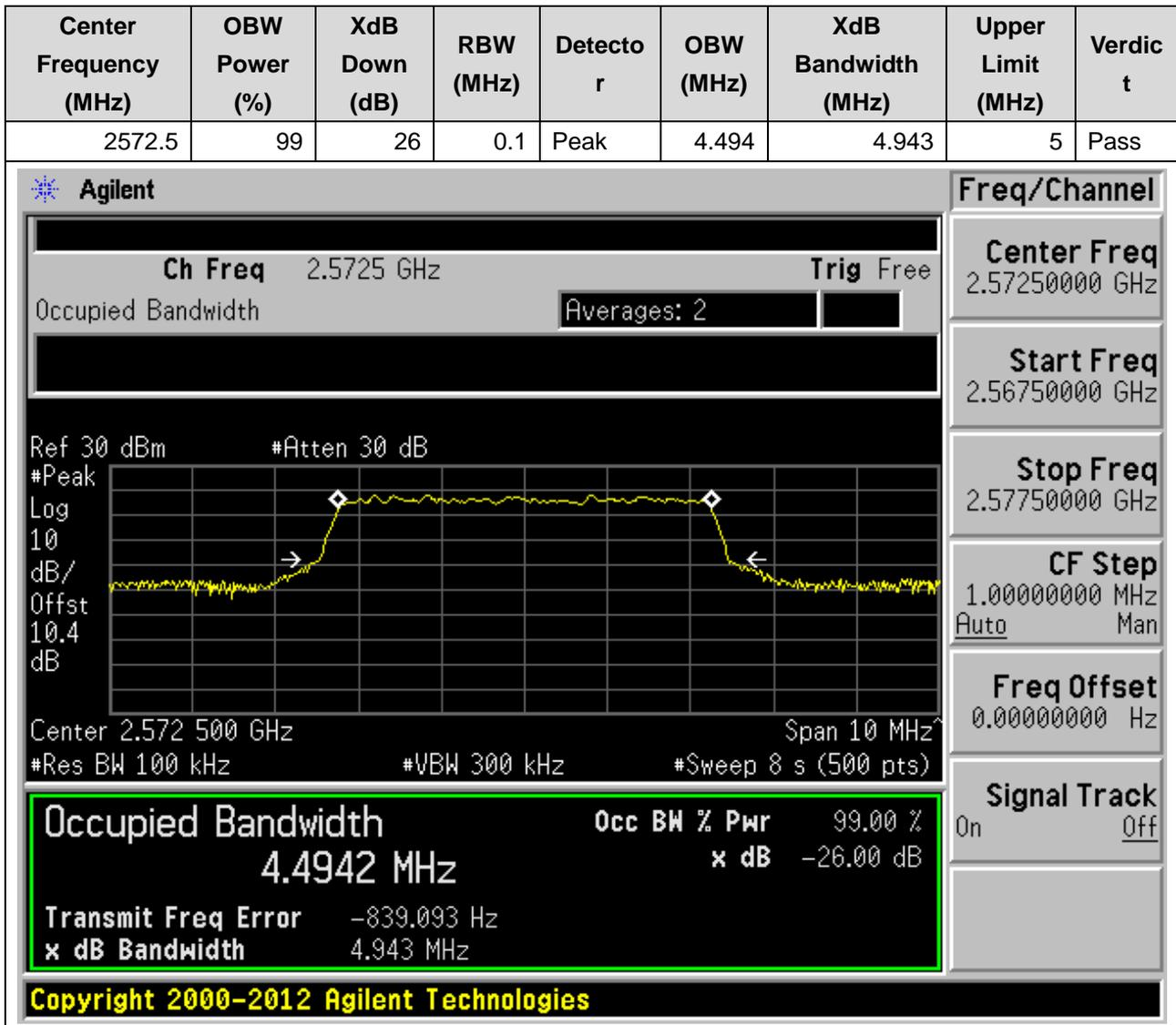
**12.2. LTE Occupied Bandwidth(NTNV)(Subtest:2, Channel:37775, Bandwidth:5, Modulation:Q16, RB Number: 25, RB Position:LOW)**
