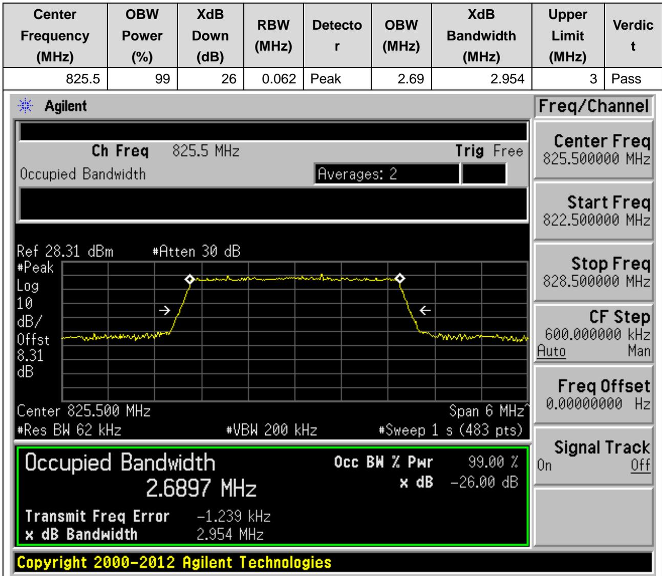
**10.8. LTE Occupied Bandwidth(NTNV)(Subtest:8, Channel:20415, Bandwidth:3, Modulation:Q16, RB Number: 15, RB Position:LOW)**
