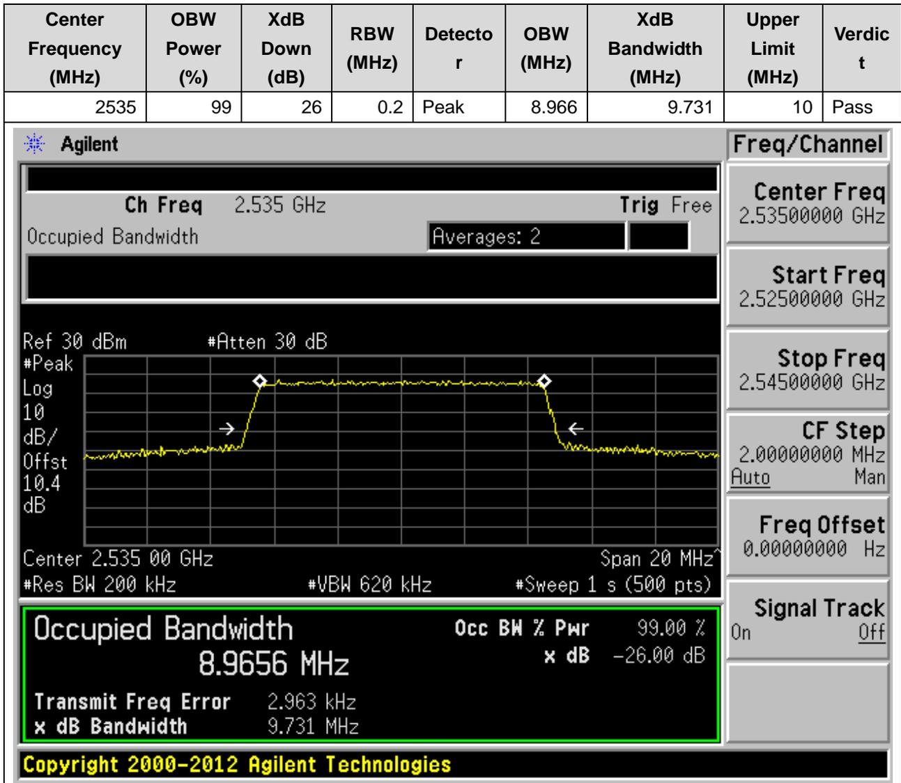
**11.11. LTE Occupied Bandwidth(NTNV)(Subtest:11, Channel:21400, Bandwidth:10, Modulation:QPSK, RB Number: 50, RB Position:LOW)**
