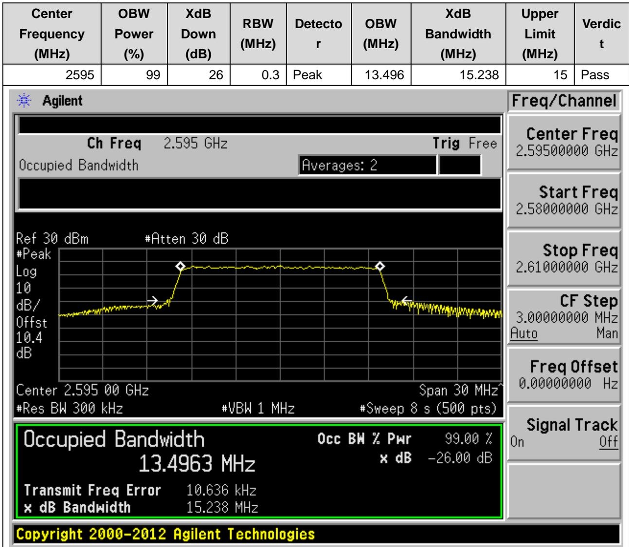
**12.17. LTE Occupied Bandwidth(NTNV)(Subtest:17, Channel:38175, Bandwidth:15, Modulation:QPSK, RB Number: 75, RB Position:LOW)**
