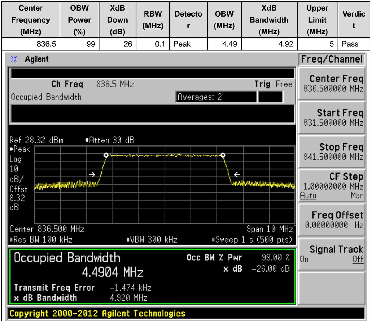
**10.16. LTE Occupied Bandwidth(NTNV)(Subtest:16, Channel:20525, Bandwidth:5, Modulation:Q16, RB Number: 25, RB Position:LOW)**
