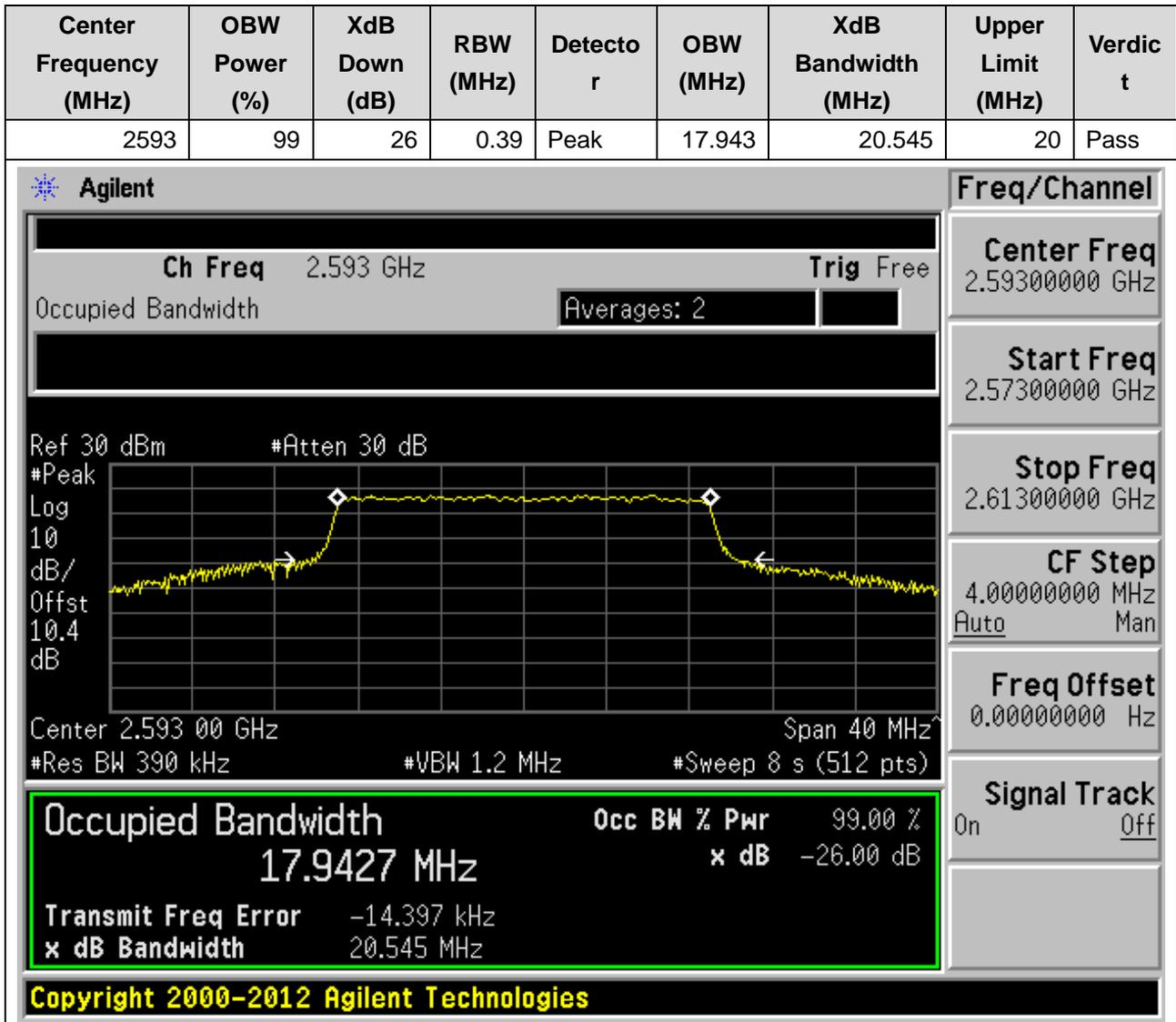
**13.23. LTE Occupied Bandwidth(NTNV)(Subtest:23, Channel:41490, Bandwidth:20, Modulation:QPSK, RB Number: 100, RB Position:LOW)**
