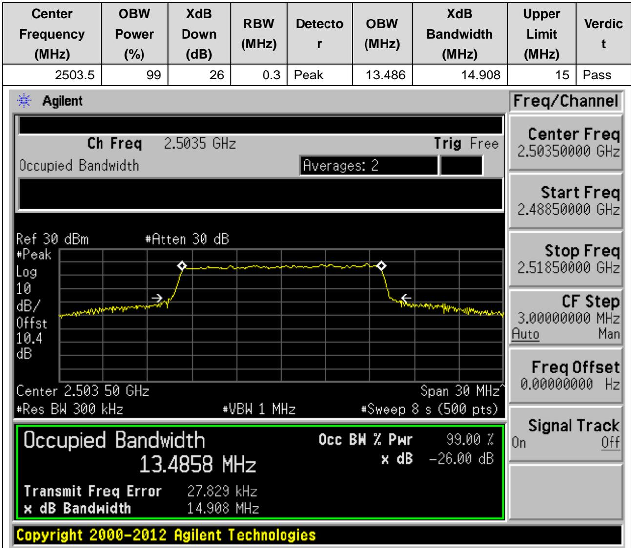
**13.14. LTE Occupied Bandwidth(NTNV)(Subtest:14, Channel:39725, Bandwidth:15, Modulation:Q16, RB Number: 75, RB Position:LOW)**
