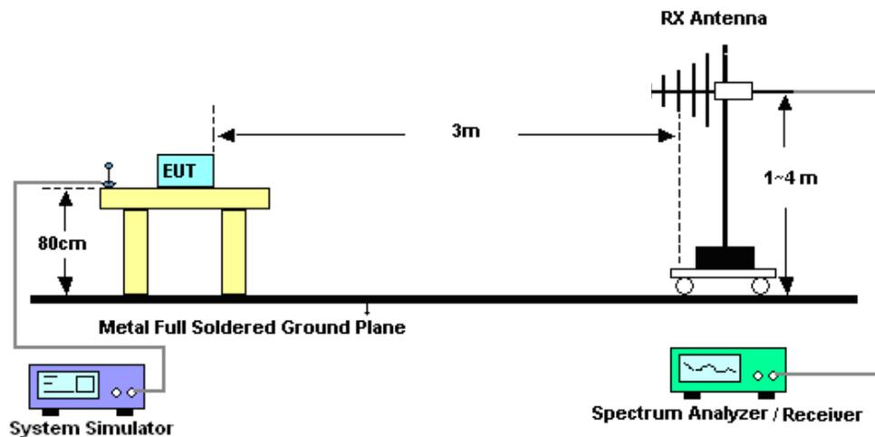
**4.2.3 For radiated test above 1GHz**
