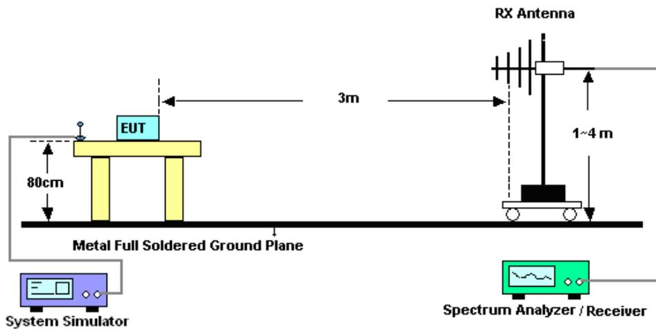
For radiated test above 1GHz
