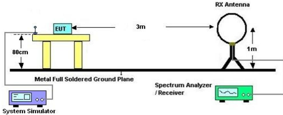
For radiated test from 30MHz to 1GHz
