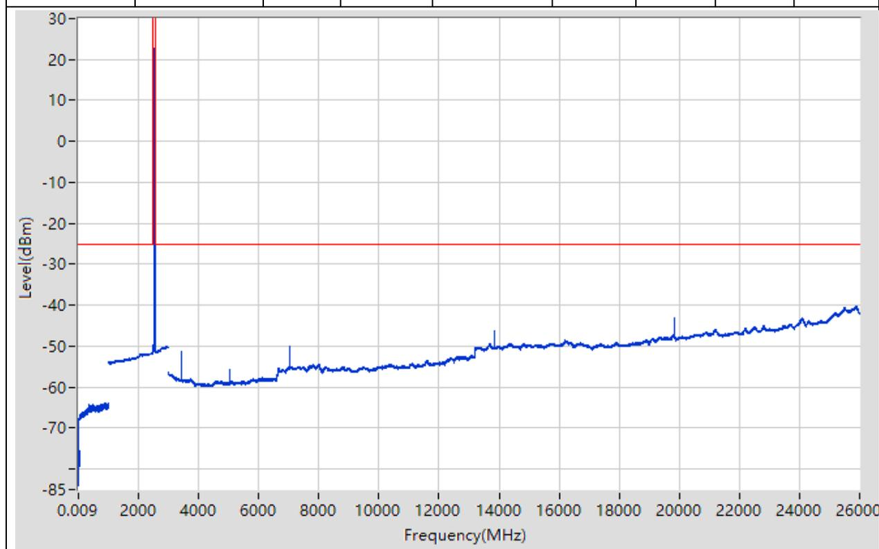
**11.22. LTE Spurious Emission at Antenna Terminals(NTNV)(Subtest:22,
