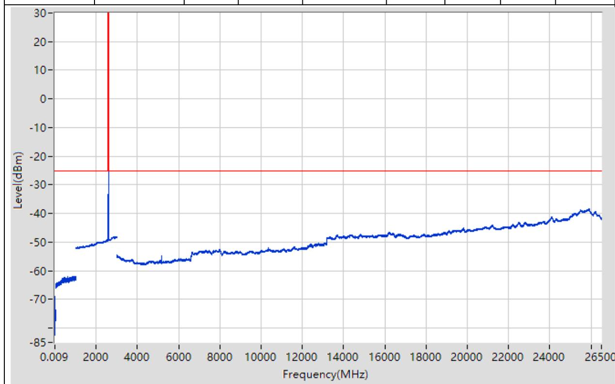
**17.10. LTE Spurious Emission at Antenna Terminals(NTNV)(Subtest:10,
