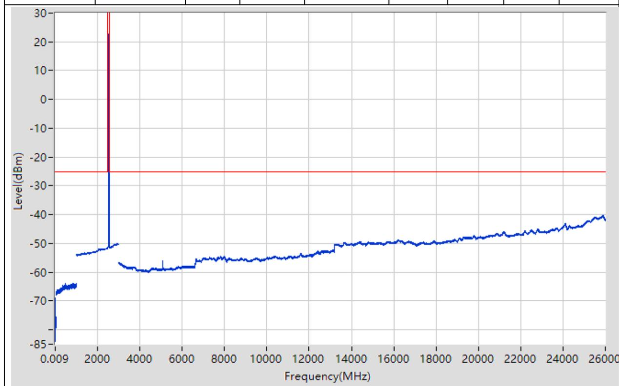
**11.10. LTE Spurious Emission at Antenna Terminals(NTNV)(Subtest:10,
