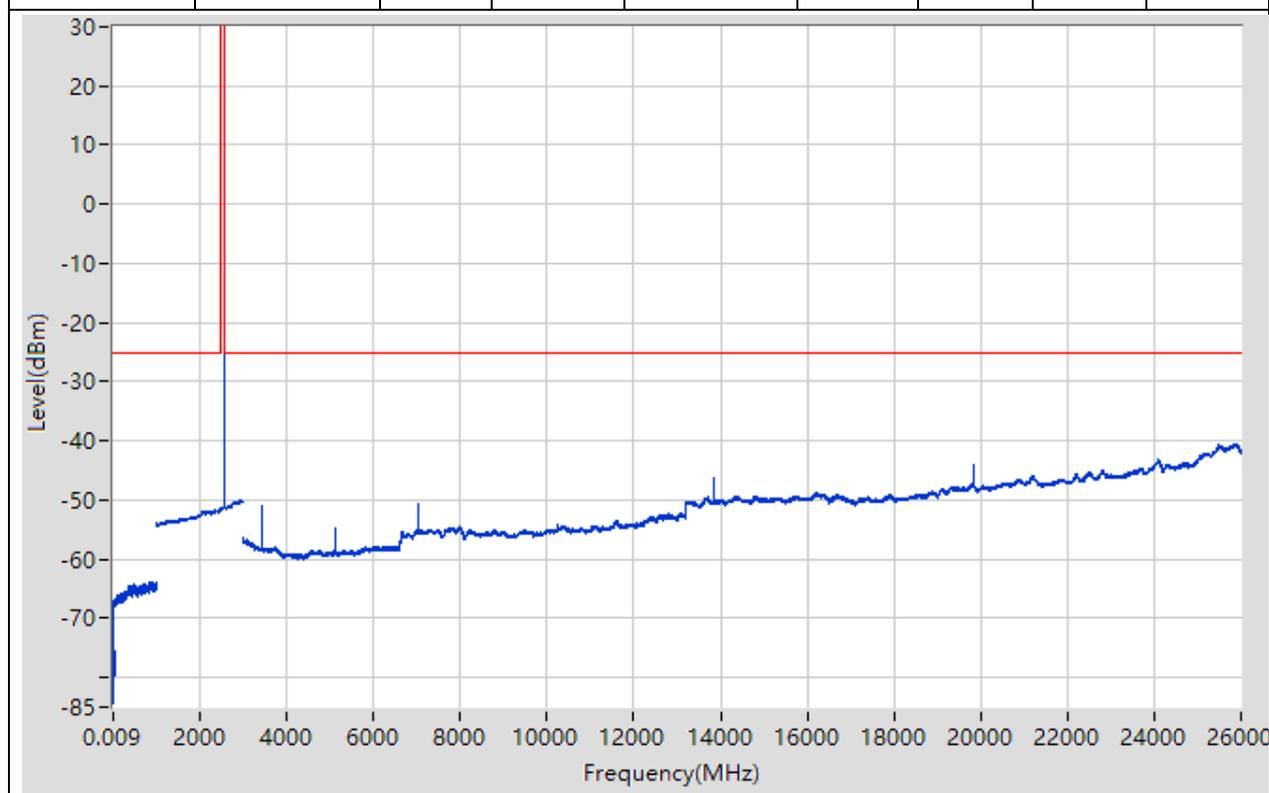
**11.12. LTE Spurious Emission at Antenna Terminals(NTNV)(Subtest:12,
