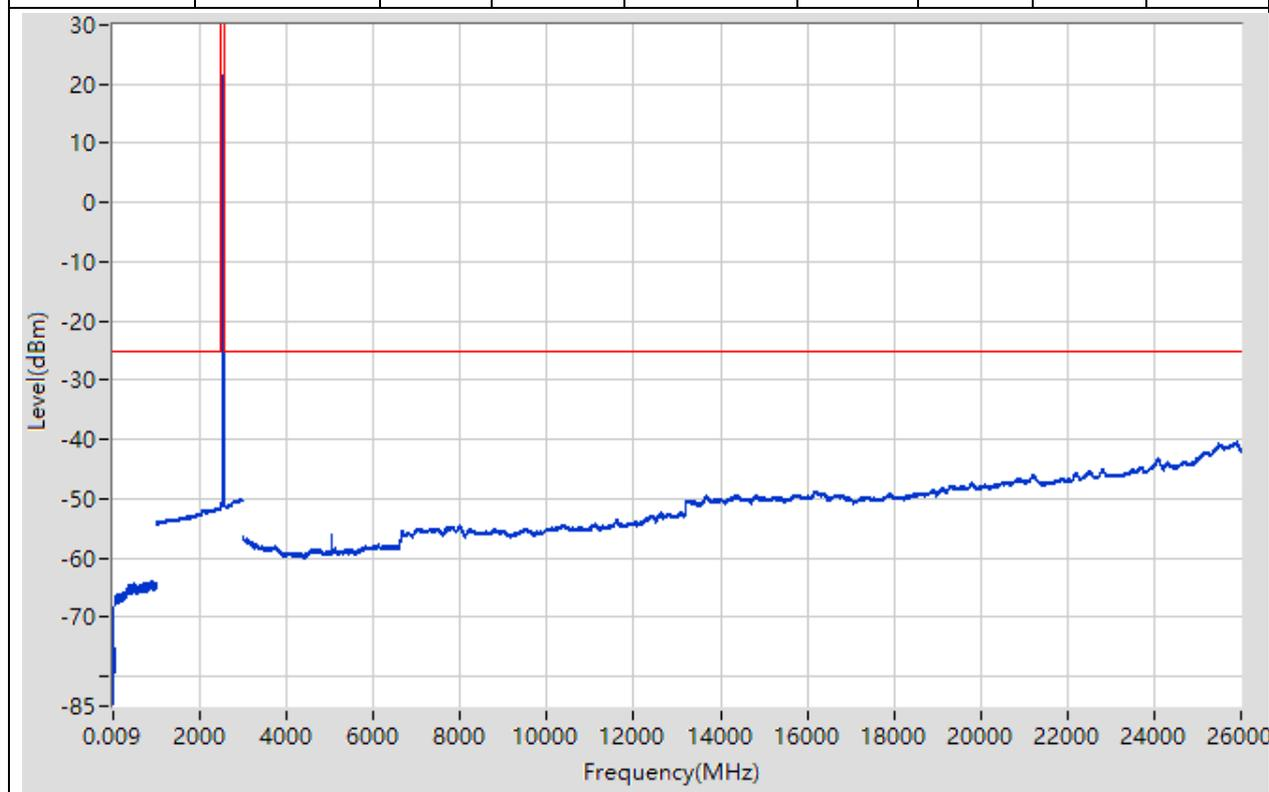
**11.23. LTE Spurious Emission at Antenna Terminals(NTNV)(Subtest:23, Channel:21350, Bandwidth:20, Modulation:QPSK, RB Number: 1, RB Position:LOW)**
