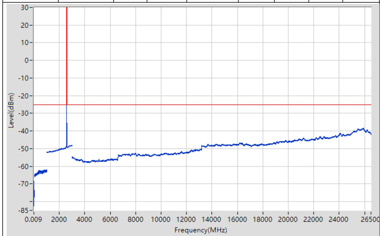
**17.15. LTE Spurious Emission at Antenna Terminals(NTNV)(Subtest:15, Channel:38000, Bandwidth:15, Modulation:QPSK, RB Number: 1, RB Position:LOW)**
