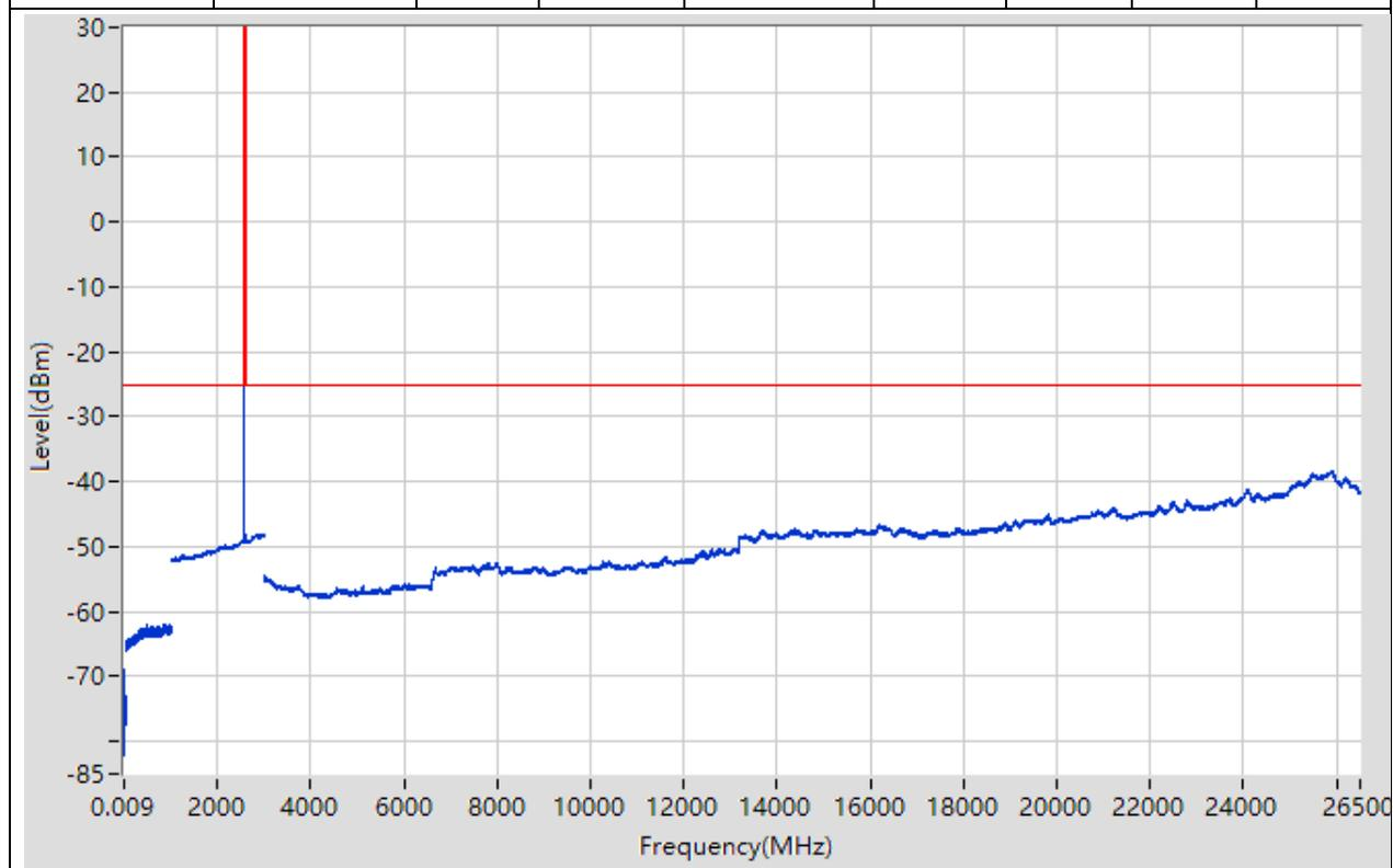
**17.3. LTE Spurious Emission at Antenna Terminals(NTNV)(Subtest:3,
