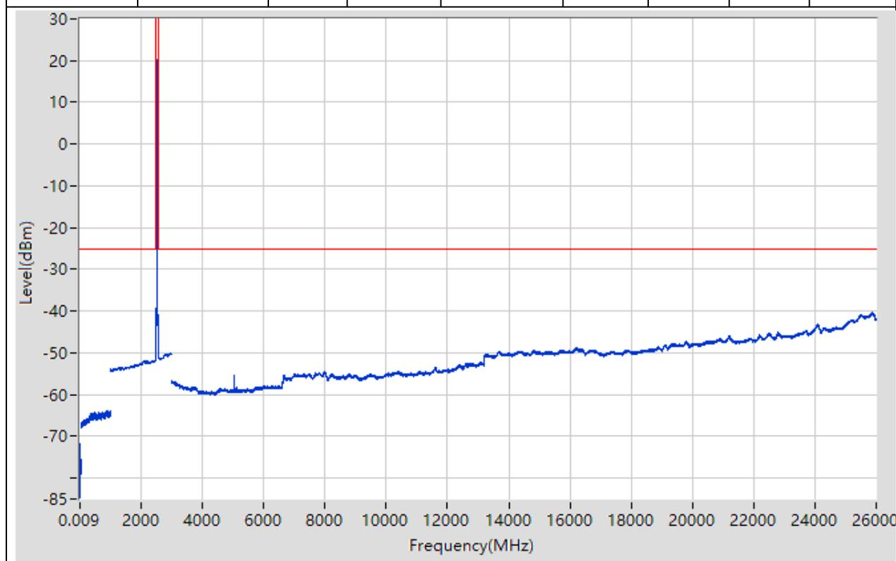
**20.3. CA Spurious Emission at Antenna Terminals(NTNV)(Subtest:3,
