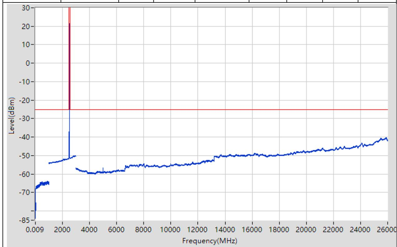
**11.15. LTE Spurious Emission at Antenna Terminals(NTNV)(Subtest:15, Channel:21100, Bandwidth:15, Modulation:QPSK, RB Number: 1, RB Position:LOW)**
