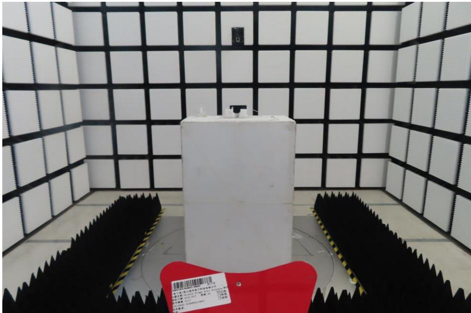
X Plane for BLE/WLAN 2.4GHz
