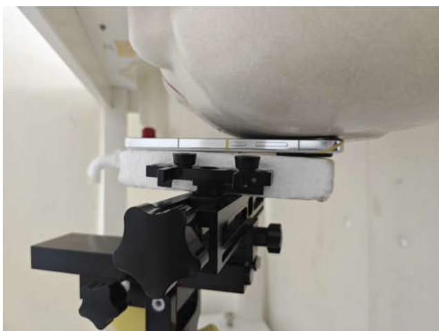
Left Cheek, Test Separation 0 mm
