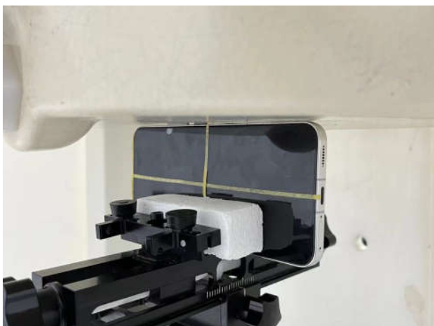
Right Side, Test Separation 0 mm
