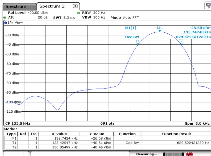
**Remark:** Because the measured signal is CW adjusting the RBW per C63.10 would not be practical since measured bandwidth will always follow the RBW and the result will be approximately twice the RBW.
