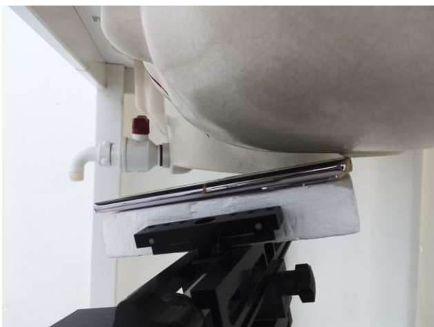
Left Tilted, Test Separation 0 mm
