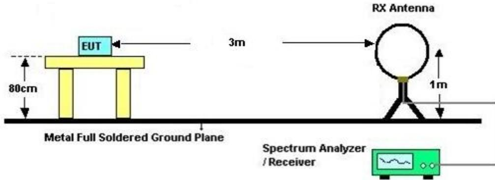
For radiated test above 30MHz
