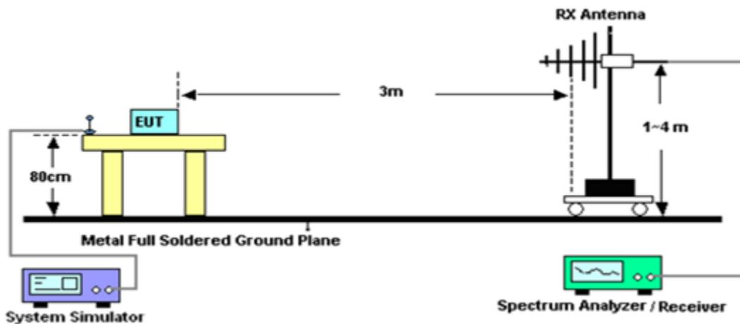
For radiated test above 1GHz
