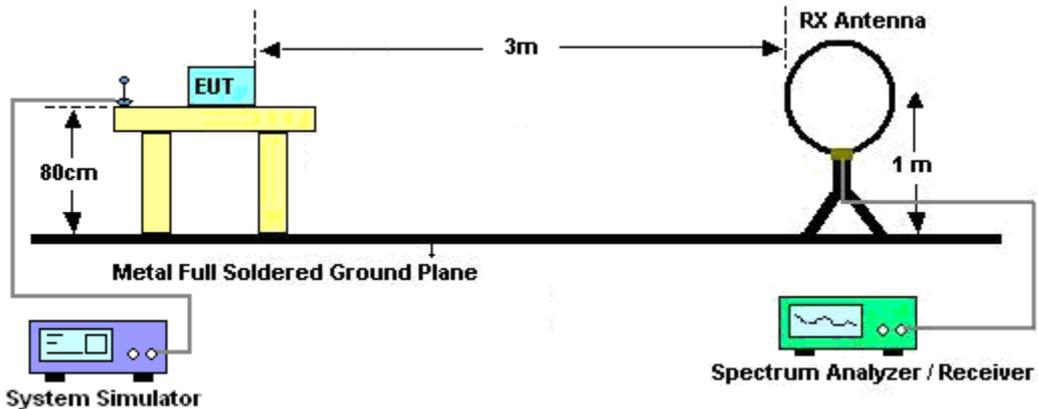
For radiated test from 30MHz to 1GHz
