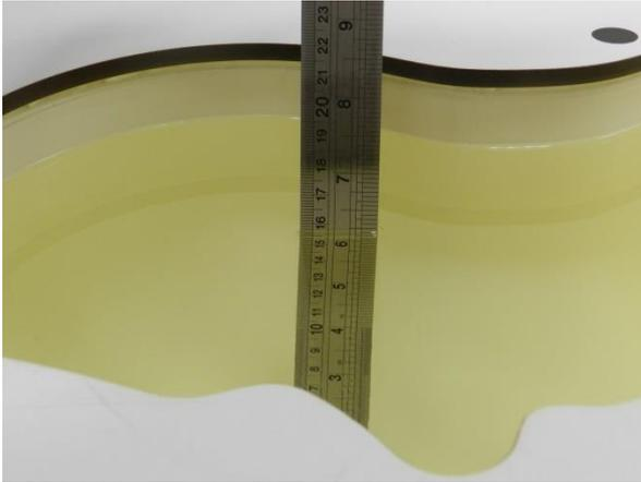
Fig 12.1 Photo of Liquid Height for Head SAR
